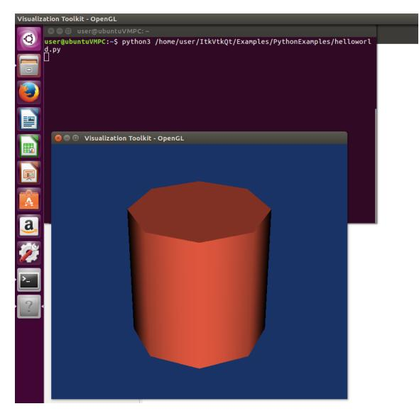
Figure 25. VTK sample helloworld application using Python wrapping
