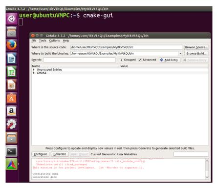
Figure 19. Application project files successfully generated
