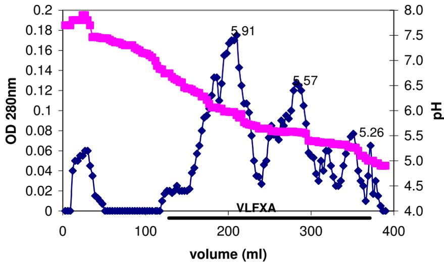
Fig. 5. Chromatofocusing of VLFXA preparation from CM-cellulose on PBE 94. Column: 0.6×38 cm. 21 mg of VLFXA fraction from CM-cellulose were dissolved in 4 ml of start buffer. Elution conditions: start buffer 0.025 M imidazole-HCl, pH 7.4, elution buffer pH 4.0, polybuffer 74-HCl (dilution 1/8), flow rate 13 ml/h, fraction volume 3 ml. ♦, protein fractions detected by absorbance at 280 nm; ---- pH gradient.
