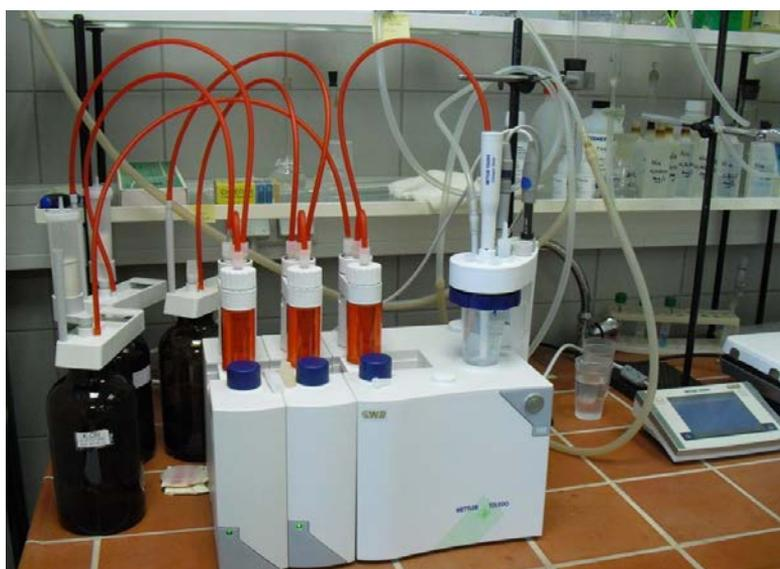
Figure 15. Mettler Toledo T90 titrator for surface charge measurements.
