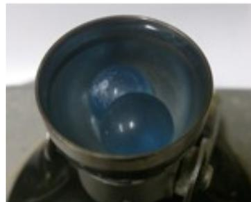
Figure 12. Vibration mill closed (left) and opened (right) with 2 glass balls with diameters of 8 mm.
