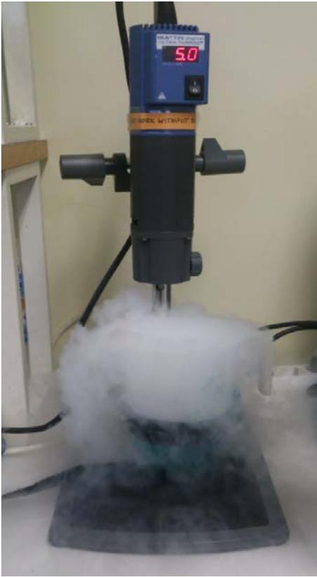
Figure 10. Cold pretreatment with Ultra Turrax T25 disperser.
