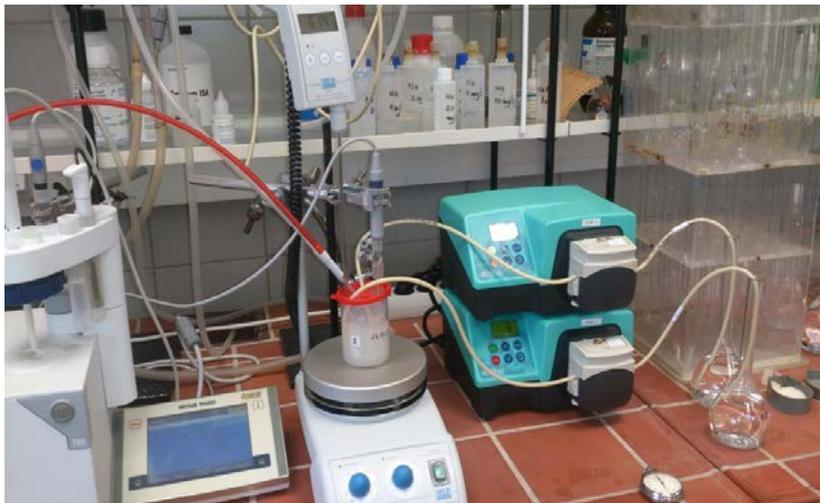
Figure 13. HAp synthesis devices consisting of a pH controller, magnetic stirrer with temperature controller, two peristaltic pumps and two additional solvents.
