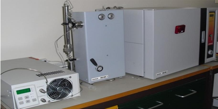
Figure 8. Experimental device for  $scCO_2$  extraction (Detailed description in Paper I and II).
