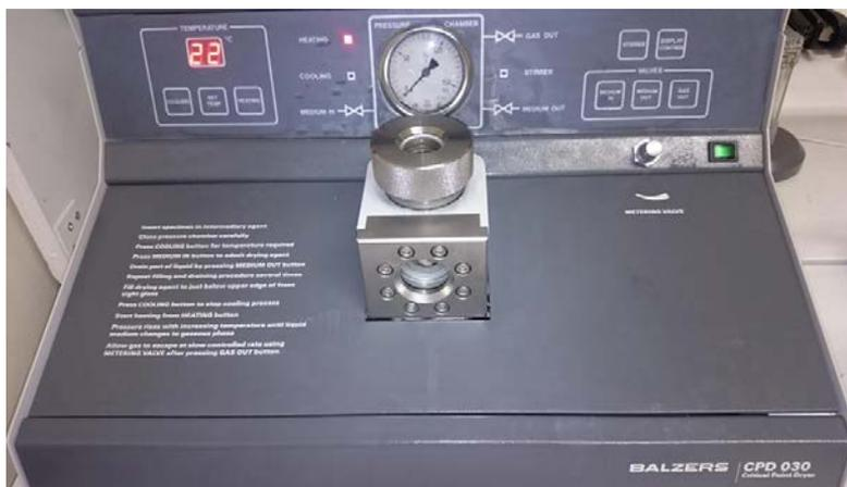
Figure 14. Balzers CPD 030 critical point dryer.
