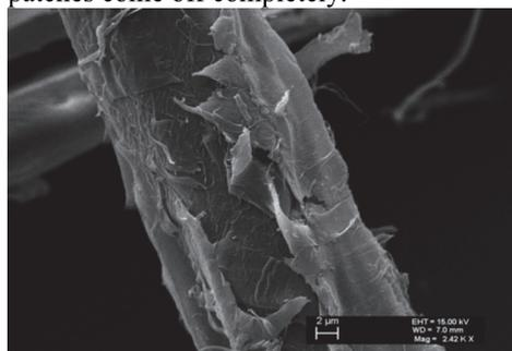
Fig. 4. Peeling effect after scCO<sub>2</sub> treatment.
