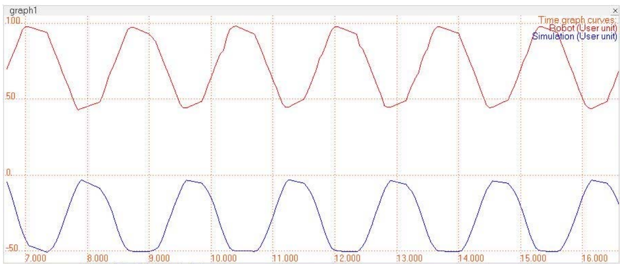
Figure 6.2 – Graph of real servo positions and simulated servo positions was made in V-REP.
