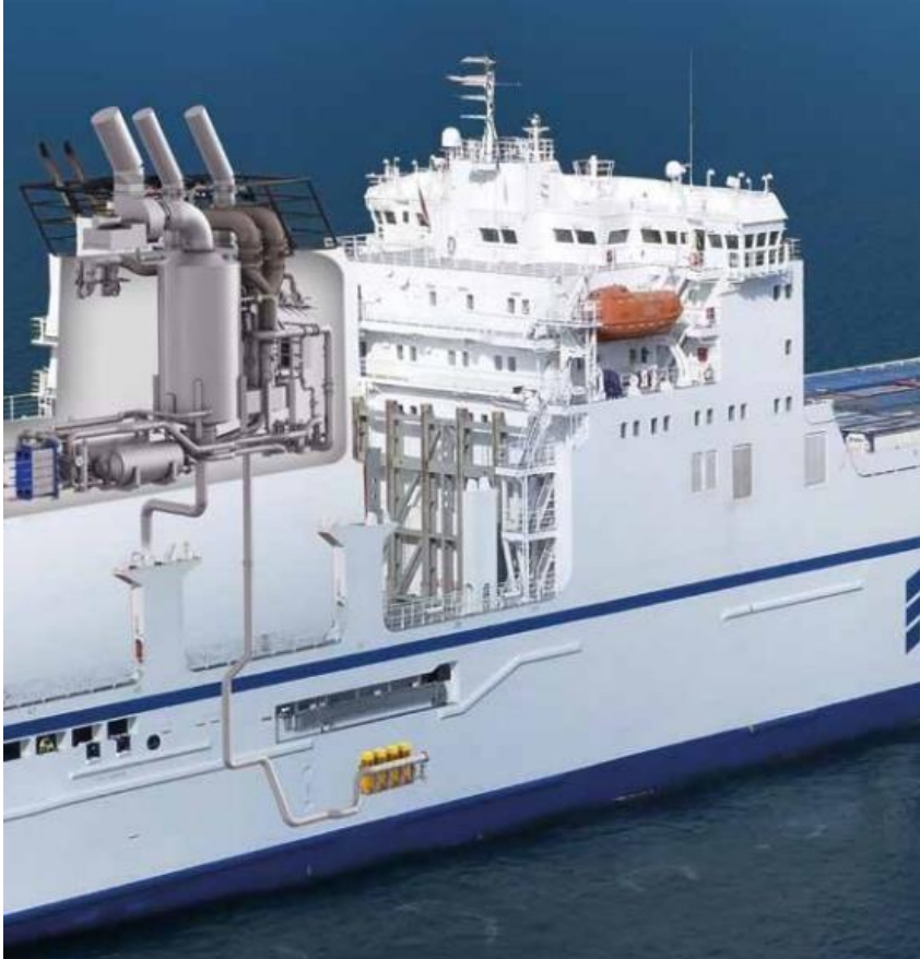
Figure 23. Scrubber installed onboard of Transfennica Ship.
