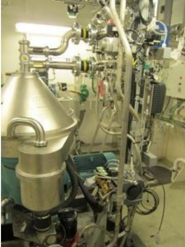
Figure 18. The centrifuge is a high-speed separator.
