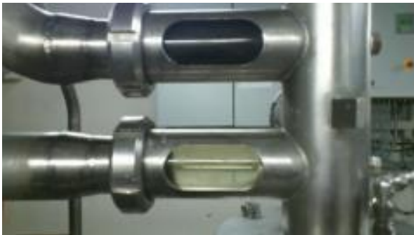
Figure 19. The dirty water is feed in through the top with a turbidity of approx. 250 FNU and the clean water leaves the separator 26 below the feed pipe with a turbidity of approx. 10 FNU. The separated sludge is shot from the separator into a collecting tank.
