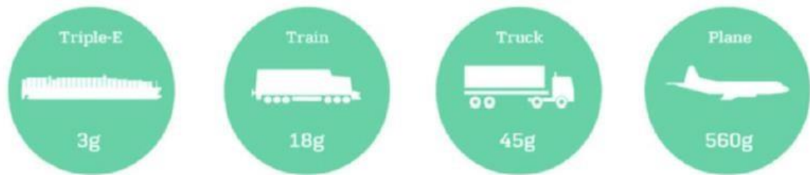
Figure 10. Estimated CO 2 emission for transporting 1 tonne of goods 1 kilometre for different transportation modes. (Triple-E is a family of very large container ships of more than 18000 TEU). Source: (Psaraftis, 2019).
