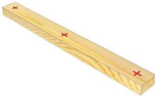
Figure 11. Position for measuring L*a*b color values [20] and measuring points on the specimens
