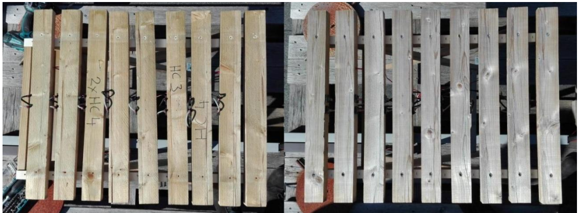
Figure 16. Under (left) and top (right) of the specimens on 5 th of May 2017 for evaluation decay of the specimens
