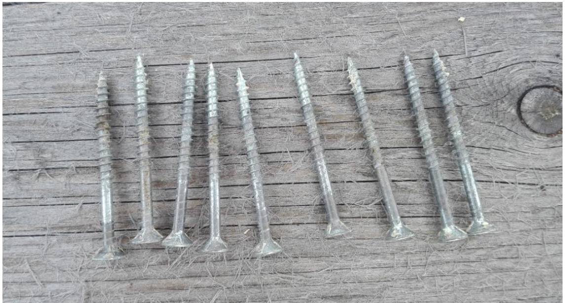
Figure 22. Galvanized screws removed from performance table on 29 th of April 2016 for inspection
