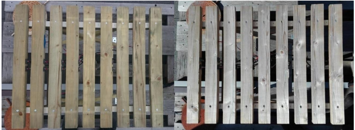
Figure 17. Topside of performance table on 8 th of April 2016 (left) and on 5 th of May 2017 (right)
