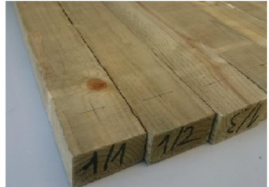
Figure 11. Position for measuring L*a*b color values [20] and measuring points on the specimens
