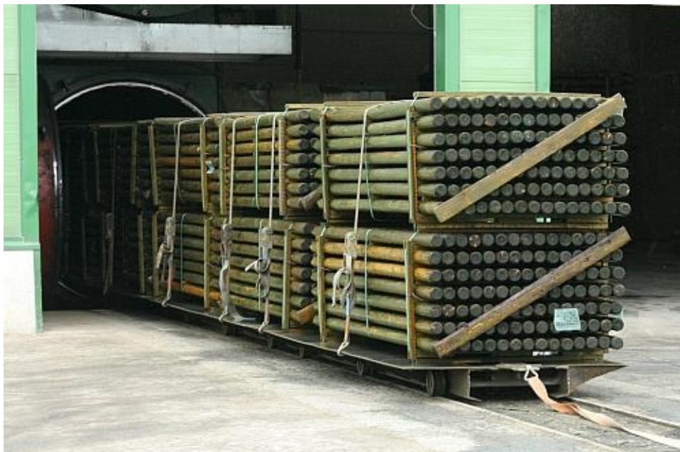
Figure 3. AS Imprest products exiting from auroclave after impregnation [9]
