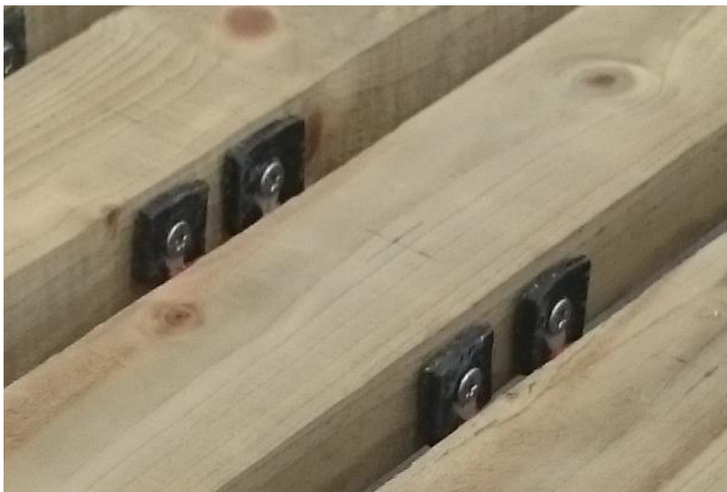
Figure 13. Isolated fasteners were used for fixing electrodes on wood specimens
