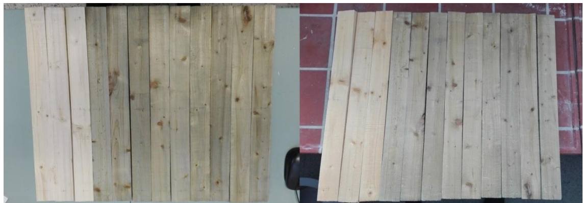
Figure 29. Test specimens before (left) and after (right) 336 hours of artificial UV irradiation
