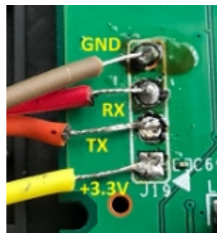
Figure 51. UART pins from EA6350 router - Retrieved from [38]
