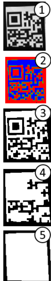
Figure 4.27 Example of processing. 1. Raw cropped image of hypercube at wavelength 1320 nm. 2. K-means clustering with 3 clusters. Background is always assigned to 0. 3. Binarized k-means result. 4. Fill holes. 5. Convex hull of the object.
