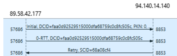
Figure 29. 0-RTT rejected by Adguards public resolver.
