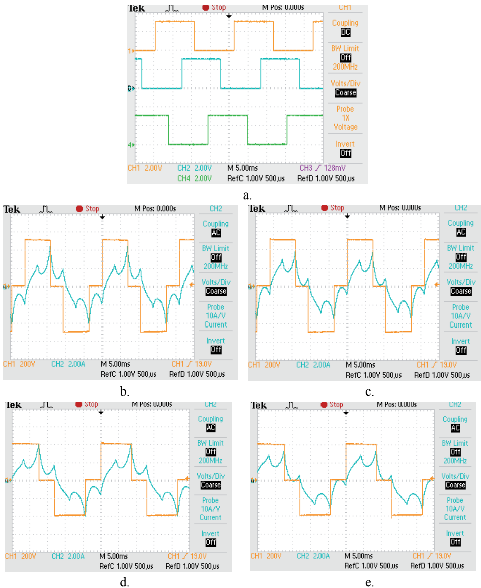
Fig. 2.7 Timing diagrams of the six-step operation from the TUT experimental setup: (a) control signals; (b) unload, f=50 Hz, line-to-line voltage and phase current; (c) load, f=50 Hz, line-to-line voltage and phase current; (d) unload, f=40 Hz, line-to-line voltage and phase current; (e) load, f=40 Hz, line-to-line voltage and phase current
