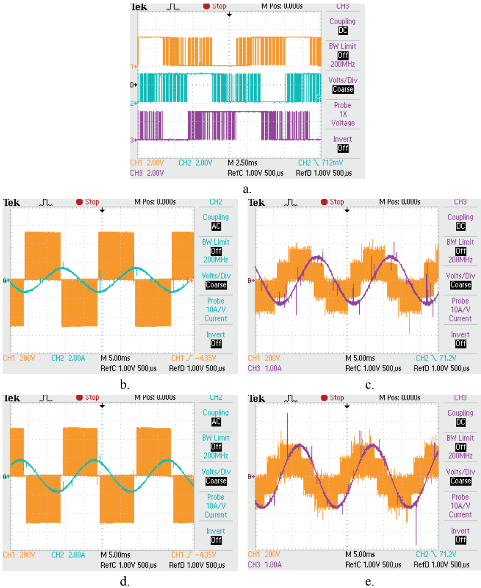
Fig. 3.8 Timing diagrams of current-dependent clamping from the TUT experimental setup: (a) control signals; (b) unload, line-to-line voltage and phase current; (c) unload, phase voltage and current; (d) load, line-to-line voltage and phase current; (e) load, phase voltage and current
