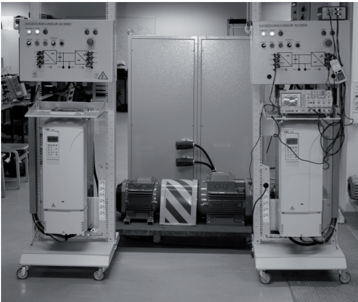
Fig. 2.1 View of the ABB ACS800 experimental setup
