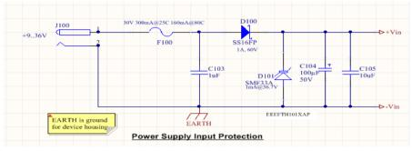
Figure 25: Power supply input for the converters
