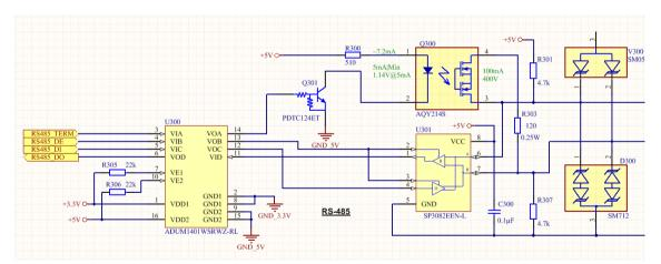
Figure 28: RS-485 circuitry with terminal resistor relay and galvanic isolation
