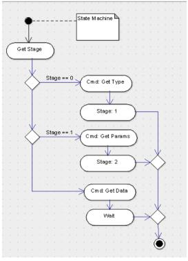
Figure 33: State machine flowchart
