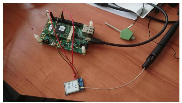
Figure 15: Connecting an XBee SX 868 to an RCM6700 development board for testing
