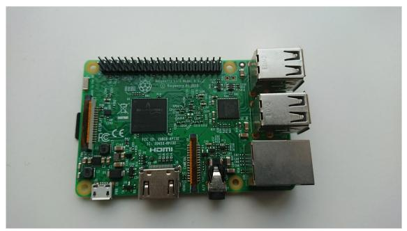
Figure 6: Raspberry Pi 3 Model B
