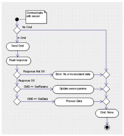
Figure 34: Communication with sensor flowchart
