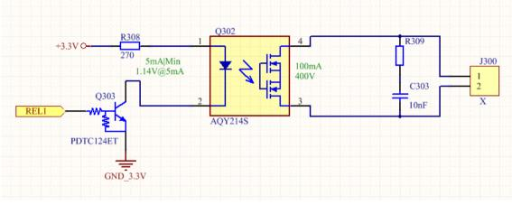
Figure 29: Alarm indication relay
