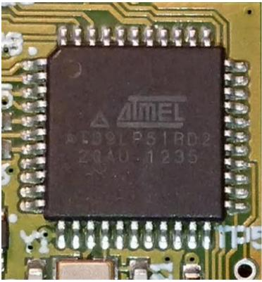
Figure 9: Atmel AT89LP51 microcontroller (8051 architecture), the one that is currently used in ROW
