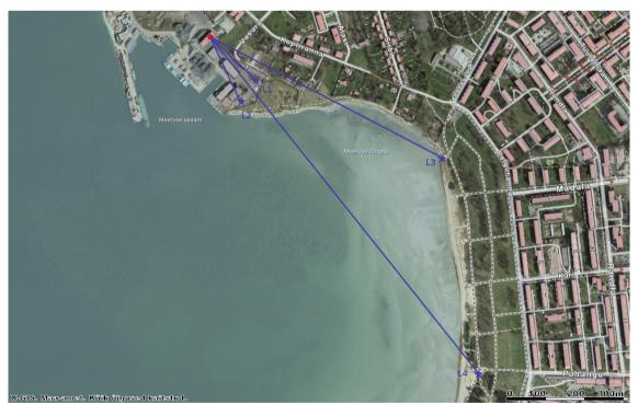
Figure 16: Range testing local modem locations (blue stars) and remote modem (red star)
