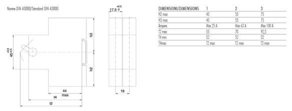
Figure 21: Enclosure dimensions according to DIN 43880 [28]
