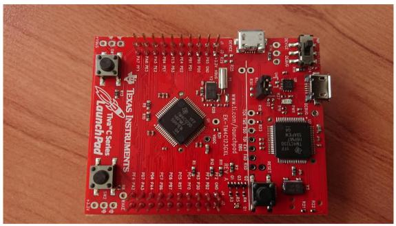
Figure 8: Texas Instruments LaunchPad with a TMC123G controller based on ARM Cortex-M4 series. This LaunchPad contains an additional microcontroller for programming and debugging.
