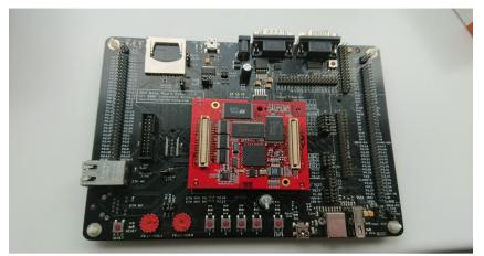
Figure 7: NXP LPC2468 (based on an older ARM7 processor) module with Keil MCB2360U development kit
