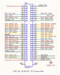
Figure 23: Mini PCI Express header
