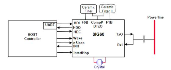
Figure 12: SIG60 interfacing and external components [15]
