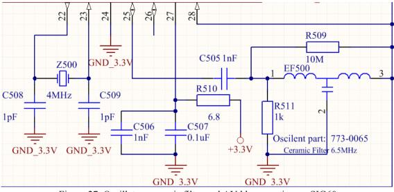
Figure 27: Oscillator, ceramic filter and AVdd connection on SIG60
