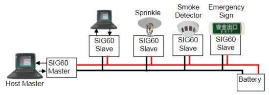
Figure 10: Example of SIG60 in fire protection network [15]
