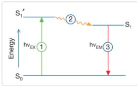
Figure 1: Jablonski diagram illustrating fluorescence process [3]
