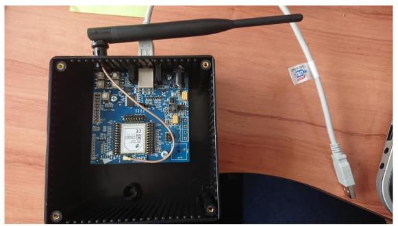
Figure 14: XBee 868LP with a Development kit
