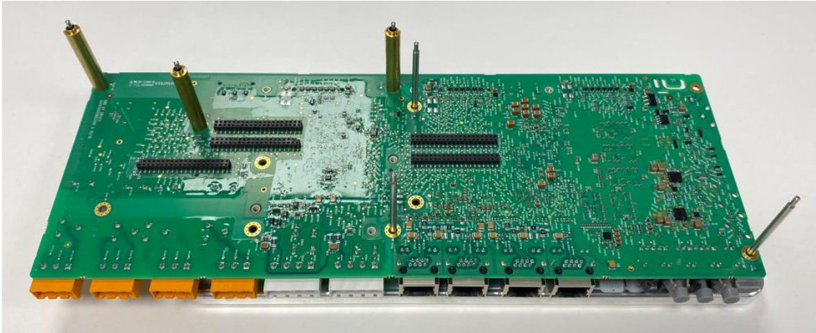
Figure 1.2 Bottom PCB (Alfa) positioned in the jig
