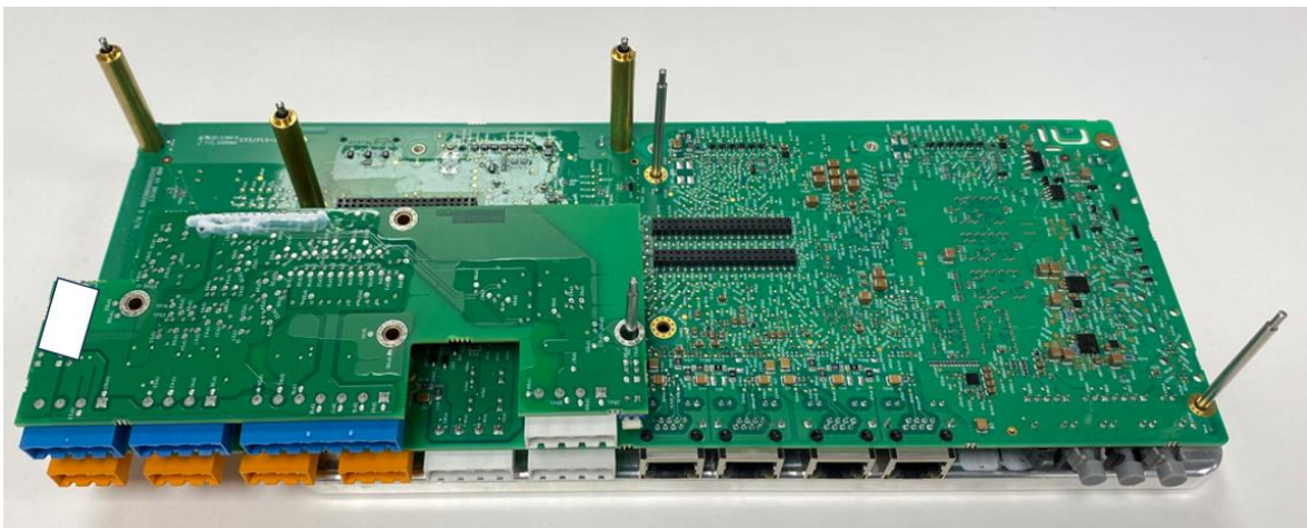
Figure 1.3. The Bravo PCB is added on the top of Alfa PCB
