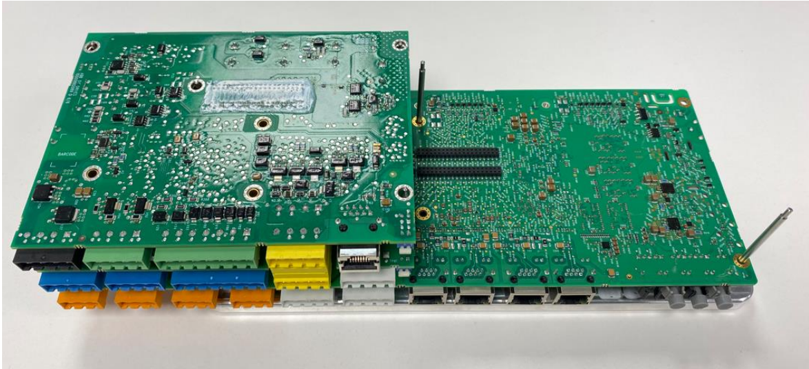
Figure 1.4. The Charli PCB is added to the assembly
