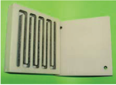
Fig. 6 Ceramic heat exchanger made of AlN with meander-like structure
