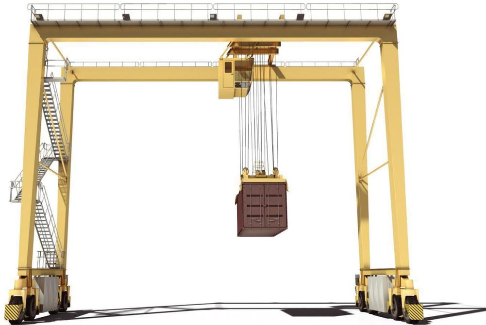
Figure 1. RTG Crane Model [Image source: \[47\]](#).
