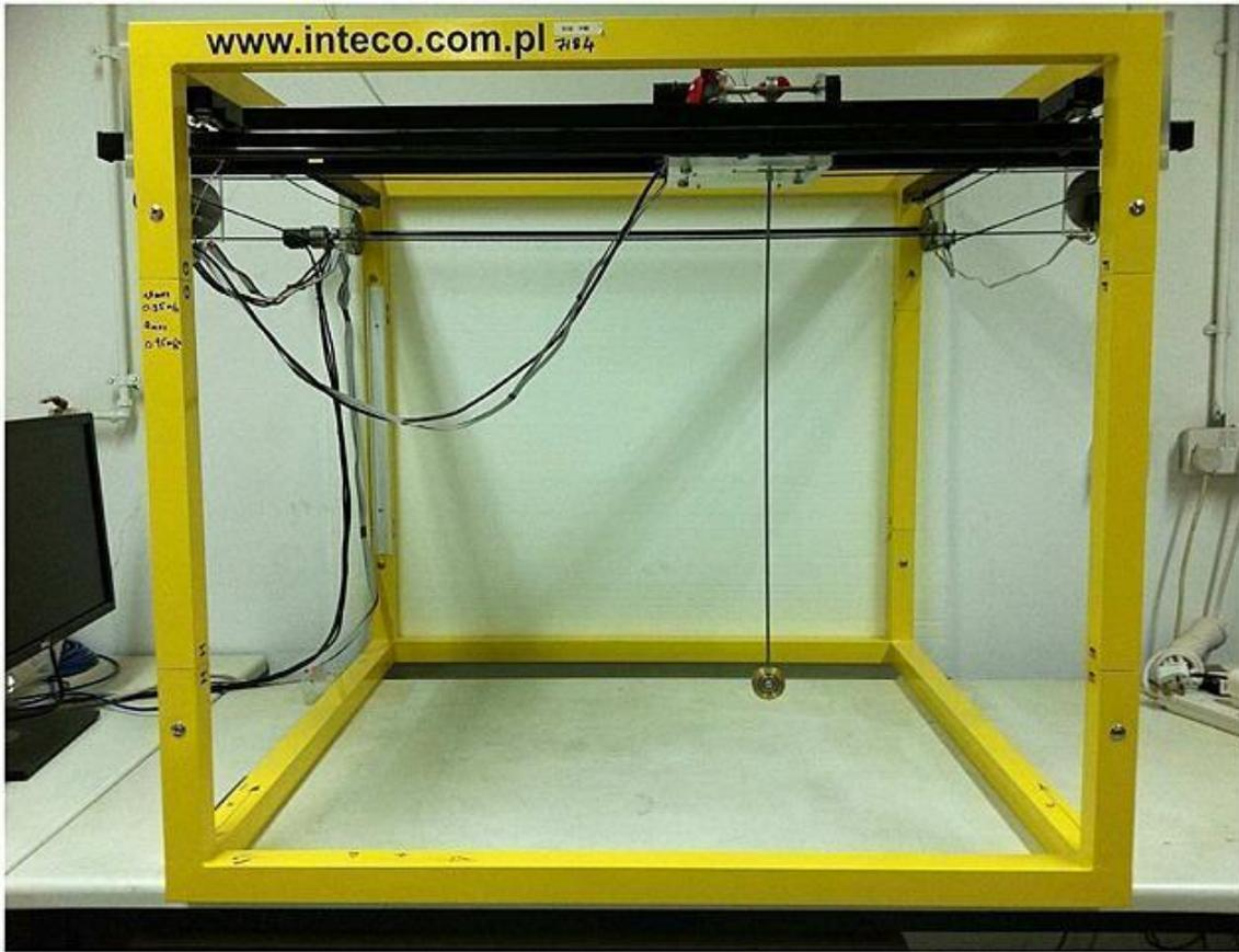
Figure 2. Laboratory Scale RTG Crane Model. Image source: [46].
