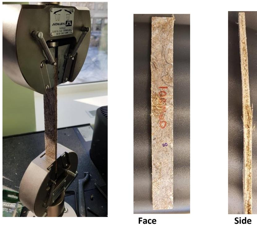
Figure 3.1 Tensile test process with test specimen after testing
