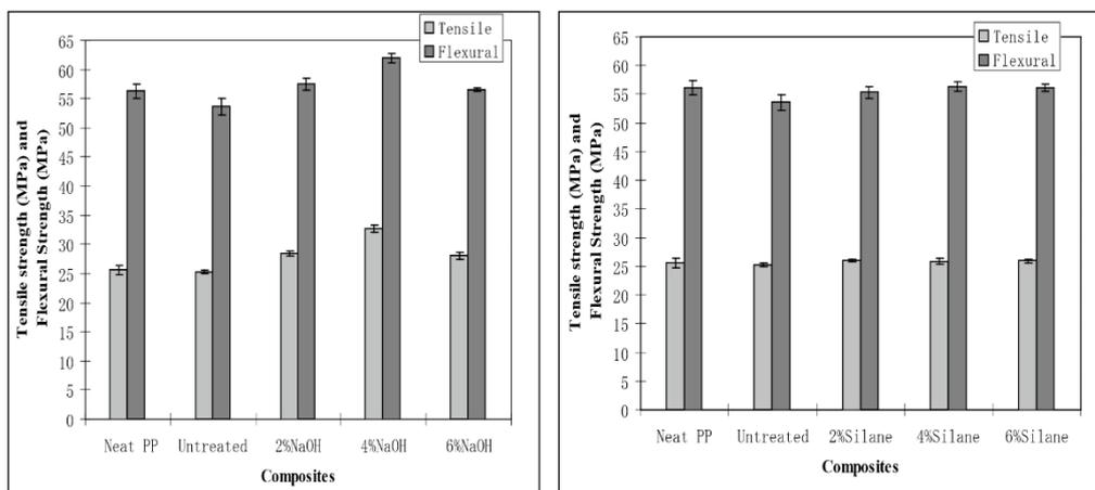
Figure 1.2 Tensile and flexural strengths of a) alkali and b) silane-treated hemp fiber-reinforced PP composites. Source (Suardana et al., 2011)
