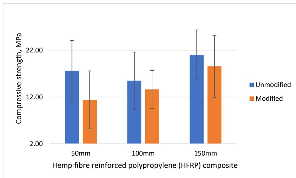
Figure 3.5 The maximum compressive strength of modified and unmodified hemp fibre reinforced polypropylene (HFRP) composite.
