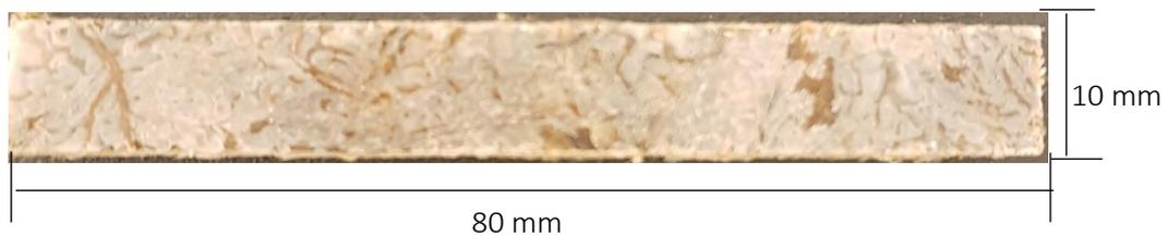
Figure 2.6 Flexural test specimen
