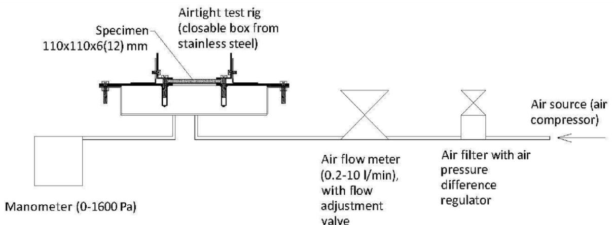
Figure 2.12 Equipment's complex scheme for carrying out the air permeability test. Source: (Villu K., 2016).
