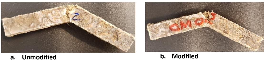
Figure 3.10 Impact failure mode for (a) and (b) HFRP composites
