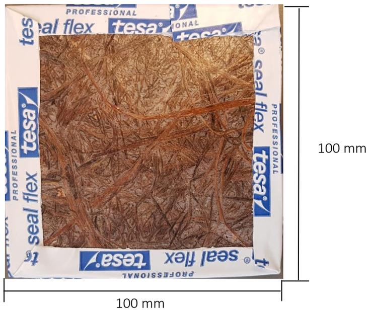
Figure 2.11 Air permeability test specimen.
