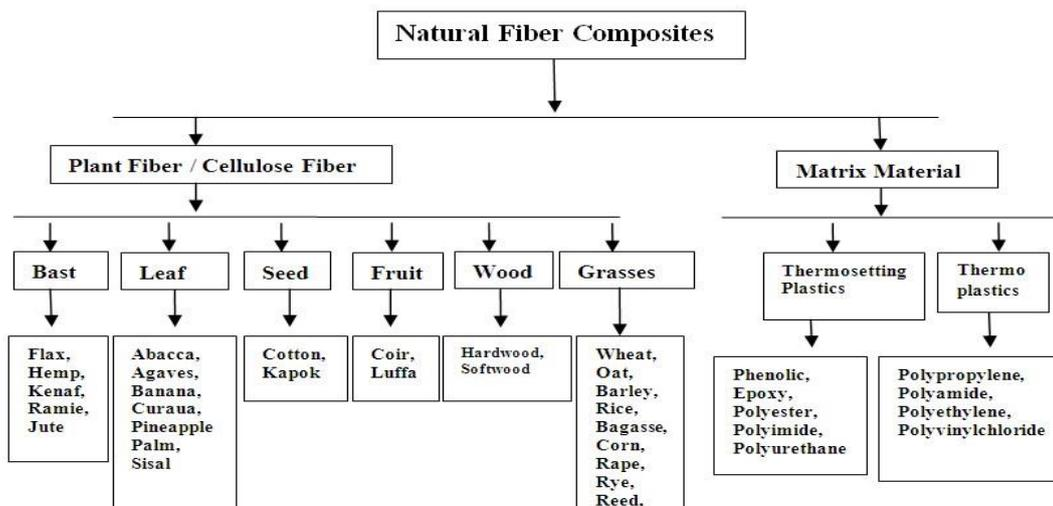
Figure 1.4 Natural fibres and matrices for polymer composites. (Sanjay et al., 2010).
