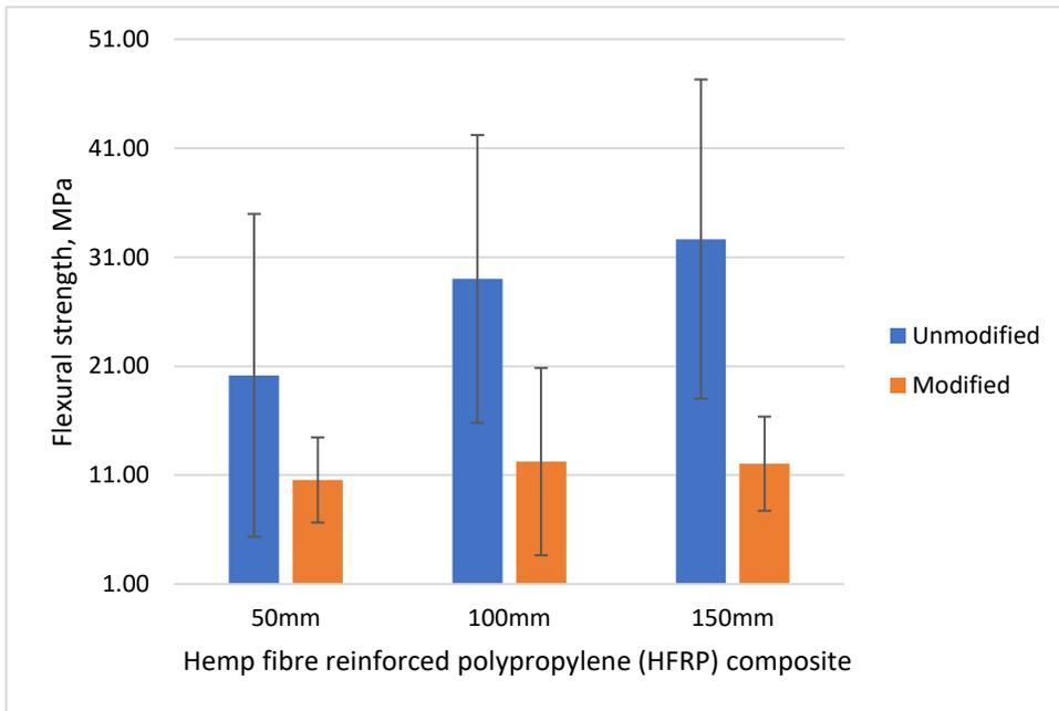
Figure 3.7 Flexural strength of HFRP composites
