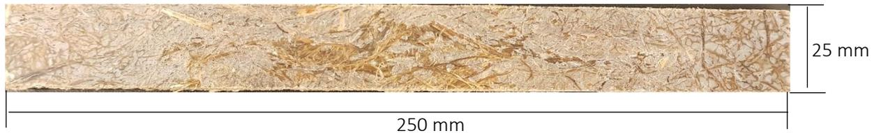
Figure 2.4 Tensile test specimen
