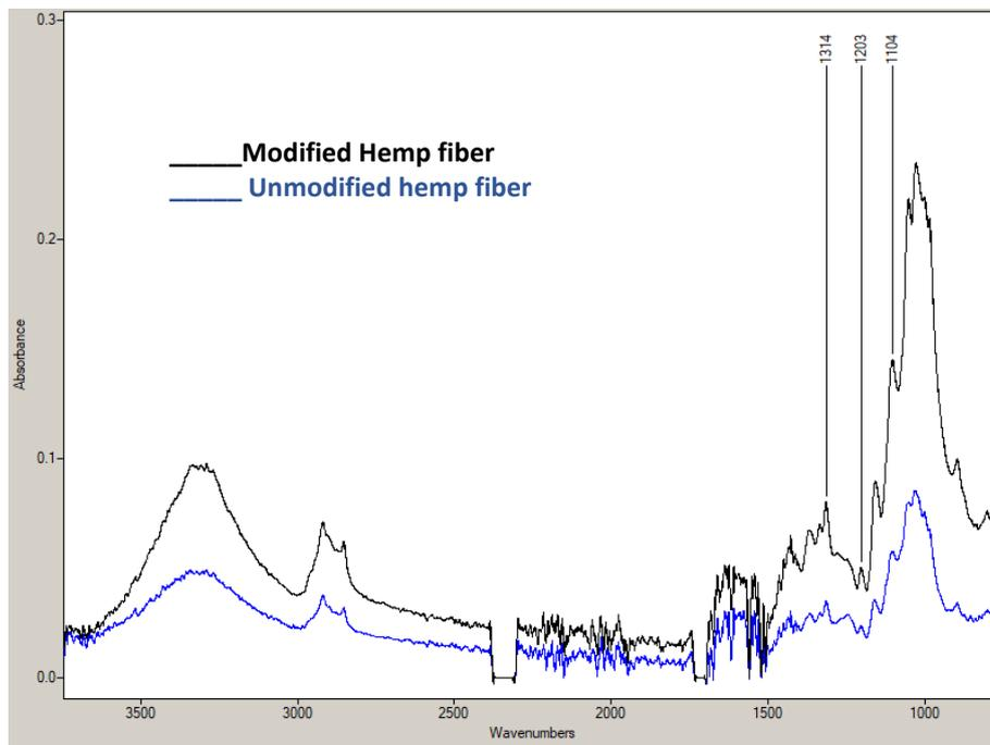
Figure 3.15. FTIR spectra of modified and unmodified hemp fibres
