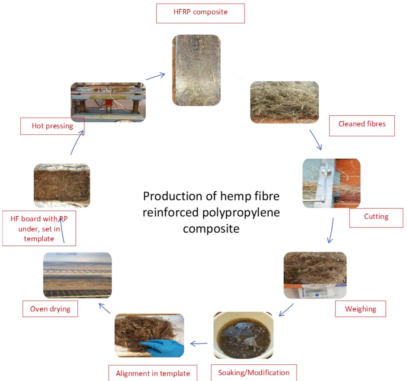
Figure 2.3 Schematic of the hemp fibre board reinforced polypropylene production
