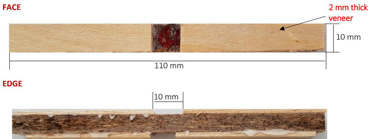
Figure 2.5 Compressive test specimen
