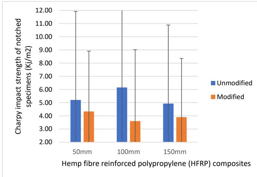
Figure 3.9 Charpy impact strength of HFRP composites
