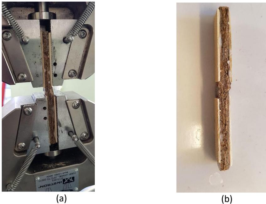
Figure 3.4 Compressive test (a) & failure type (delamination)(b)
