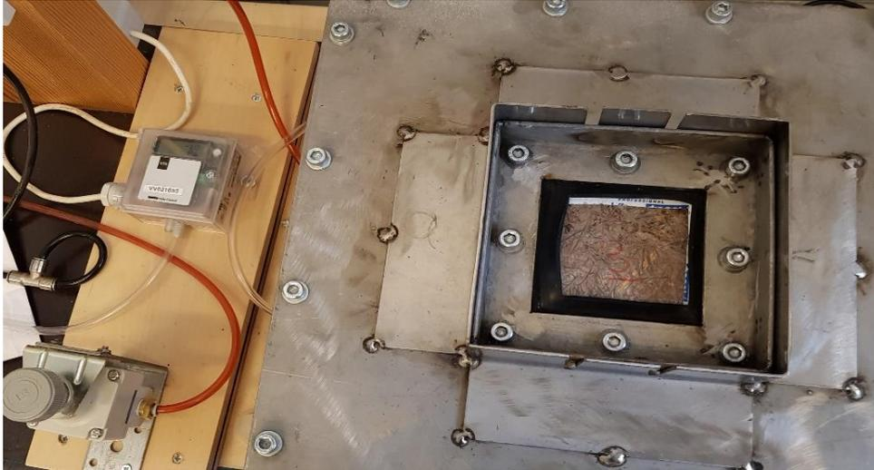
Figure 2.13 Air permeability specimen in test box
