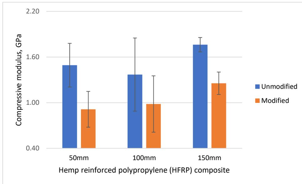
Figure 3.6 Compressive modulus of HFRP composite from modified and unmodified hemp fibres
