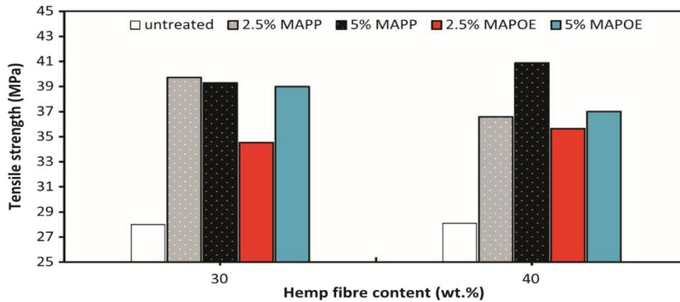
Figure 1.3 The influence of coupling agent type and their content on tensile strength of the noil hemp fibre reinforced polypropylene composites. Source: (Etaati et al., 2014).
