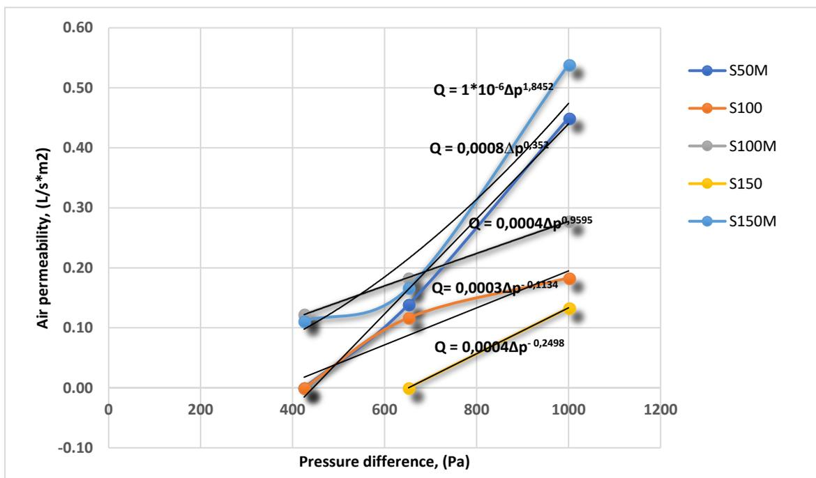
Figure 3.14 Growth rate of air flows in second pressure test stage.
