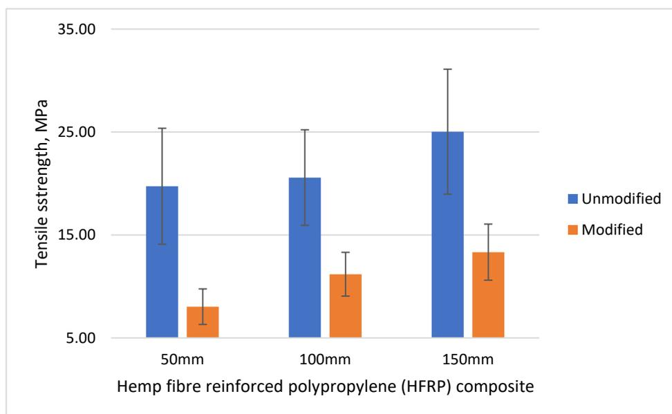
Figure 3.2 Tensile strength of HFRP composites
