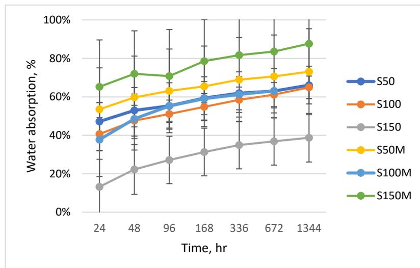
Figure 3.11 Water absorption of HFRP composites
