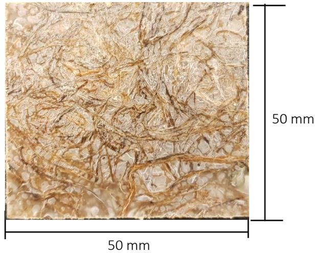
Figure 2.10 Water absorption and thickness swelling specimen
