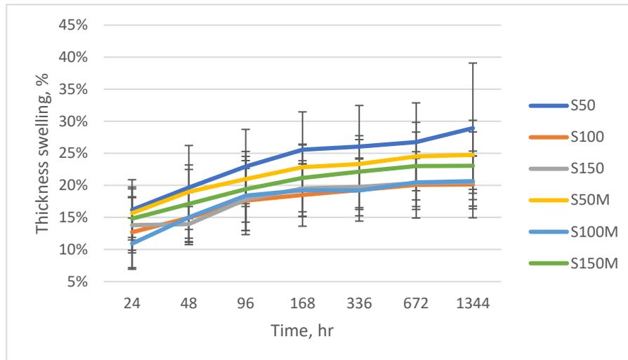
Figure 3.13 Thickness swelling of HFRP composite
