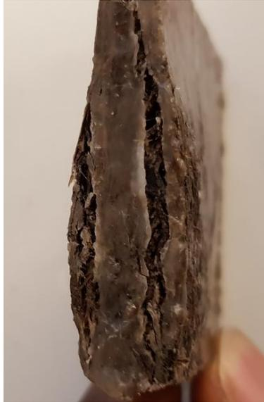
Figure 3.12 Wax removal from specimen edge during soaking.
