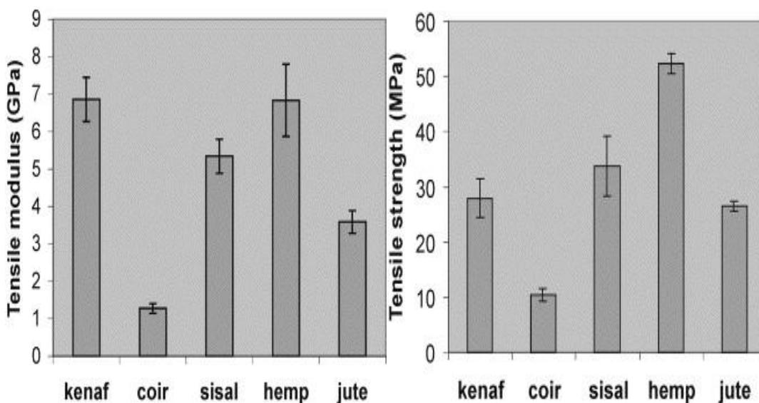
Figure 1.5 Tensile strength & Tensile modulus of fibre reinforced polypropylene composites. (Wambua et al. 2003).
