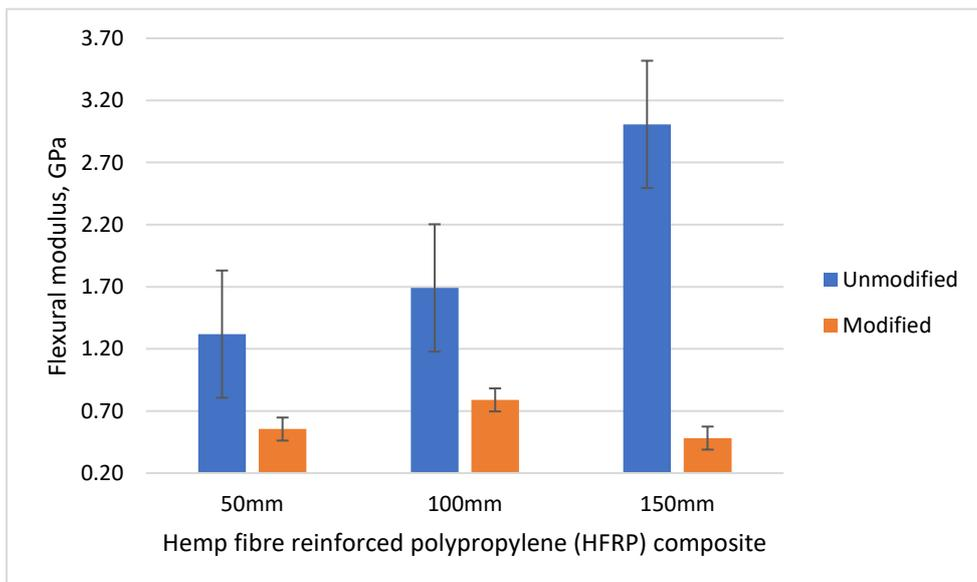
Figure 3.8 Flexural modulus of HFRP composites
