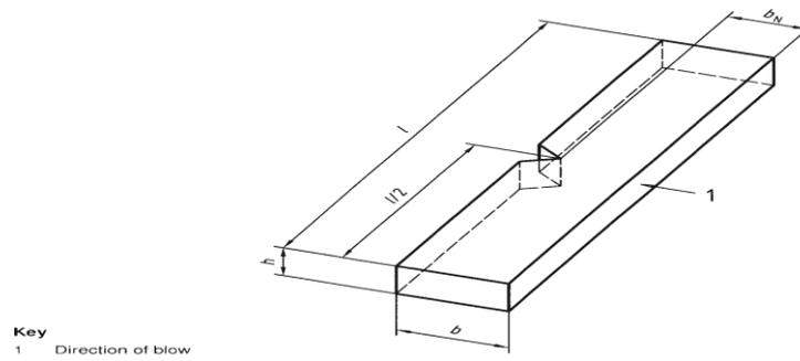
Figure 2.9. Charpy impact edge wise schematics (Source: EN ISO 179-12000)
