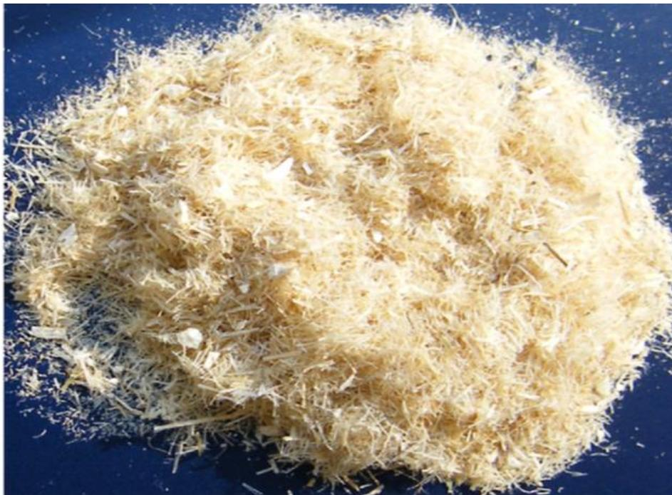
Figure 1.1. Hemp fibre (HF). Source: (Denis et. al (2016))
