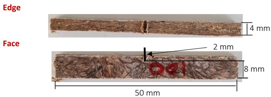
Figure 2.7 Charpy impact test specimen
