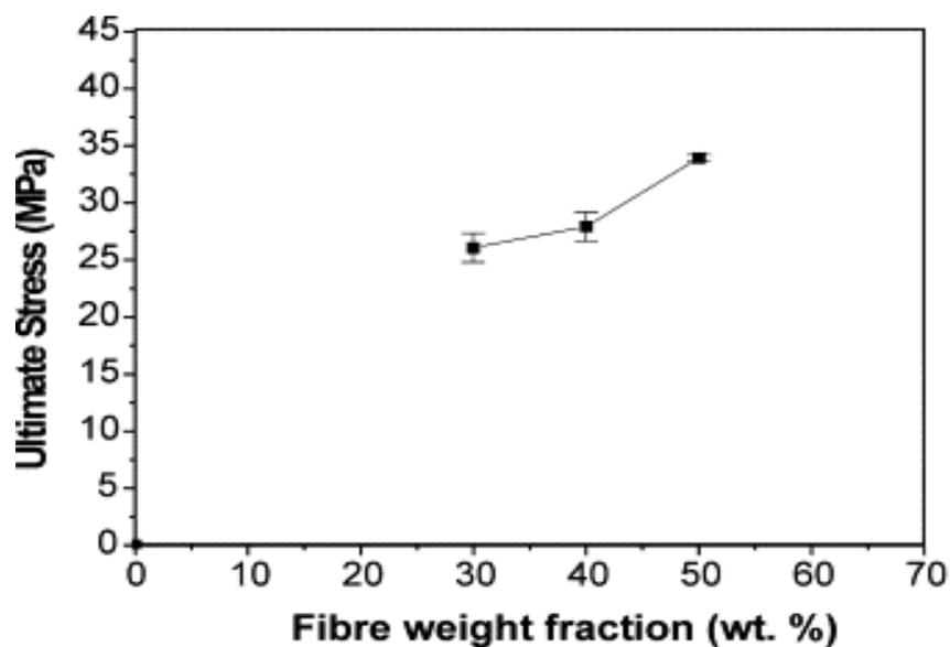
Figure 1.6 Effect of fibre weight fraction on the tensile strength of KFRP composites. Source: (Thomason, 2015).
