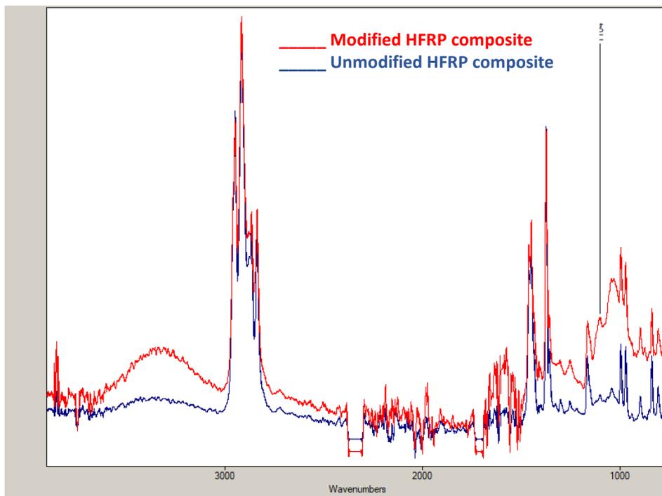
Figure 3.16 FTIR spectra of modified and unmodified hemp fibre composite.
