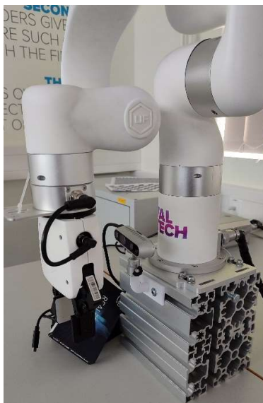
Figure 4-2 shows the 3d Printed Mount and Camera Position. When robot arm is moved away it grants a field of view that maximizes possibility of detecting dangerous items
