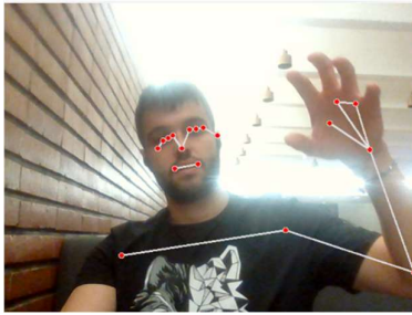
Figure 4-3 sample of pose estimator node. In this example the 4 points of the left hand note in red are used to approximate the feature of interest for tracking hands
