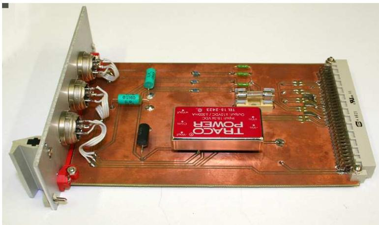
Fig. 3.22 Voltage measurement PCB
