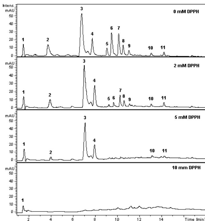
**Figure 10.** The chromatograms of the *S. melongena* extract registered at  $\lambda = 280$  nm at different concentrations of DPPH. **Peaks:** 1 – quinic acid derivative, 2 – unknown compound, 3 – isomer 1 of chlorogenic acid, 4 – isomer 2 of chlorogenic acid, 5 – isomer 3 of chlorogenic acid, 6 – cinnamic acid derivative, 7 – isomer 1 of dihydroxycinnamoyl amide, 8 – isomer 2 of dihydroxycinnamoyl amide, 9 – *N,N*-dicafeoylspermidine, 10 – kaempferol rutinoside, 11 – kaempferol glucoside.
