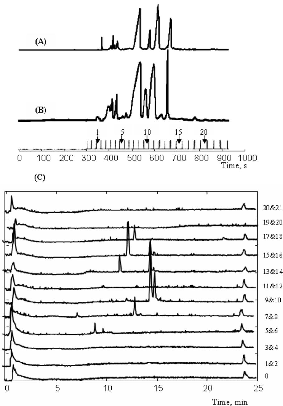
**Figure 5.** The analysis of the extract of *S. japonica*. (A) – the electropherogram of the extract of *S. japonica*; (B) – the electropherogram of the concentrated extract; (C) – the corresponding total ion chromatograms of the fractions. The CZE separation conditions are the same as in Figure 4.
