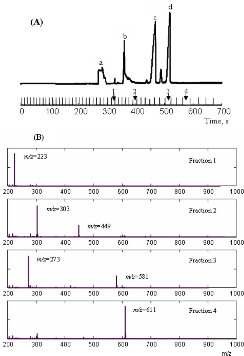
**Figure 4.** The analysis of a standard mixture of flavonoids by CE-ESI-MS. (A) The electropherogram of the solution of standards (each of 1 mM). *Peaks:* *a* – flavone; *b* – naringin; *c* – rutin; *d* – quercitrin. (B) Mass spectra of the corresponding fractions.
