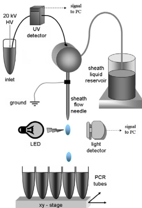
**Figure 2.** A schematic of the fraction collector
