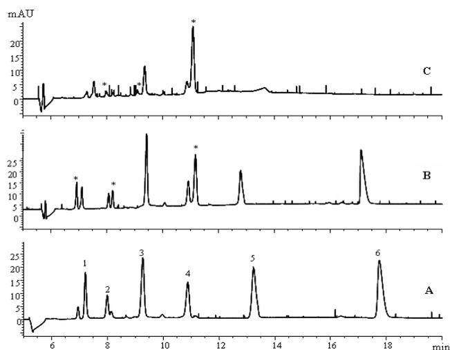
**Figure 6.** The electropherograms of the monitoring of the oxidation reaction by a stable free radical DPPH. **A** – the model solution of phenolic compounds (50  $\mu$ M); **B** – the model solution of the phenolic compound treated with a 0.2 mM DPPH; **C** – the model solution of the phenolic compound treated with a 0.8 mM DPPH. **Peaks:** 1 – *trans*-resveratrol; 2 – astringin; 3 – rutin; 4 – 3-chlorogenic acid; 5 – quercetin; 6 – gallic acid; \* – a product of the oxidation reaction.
