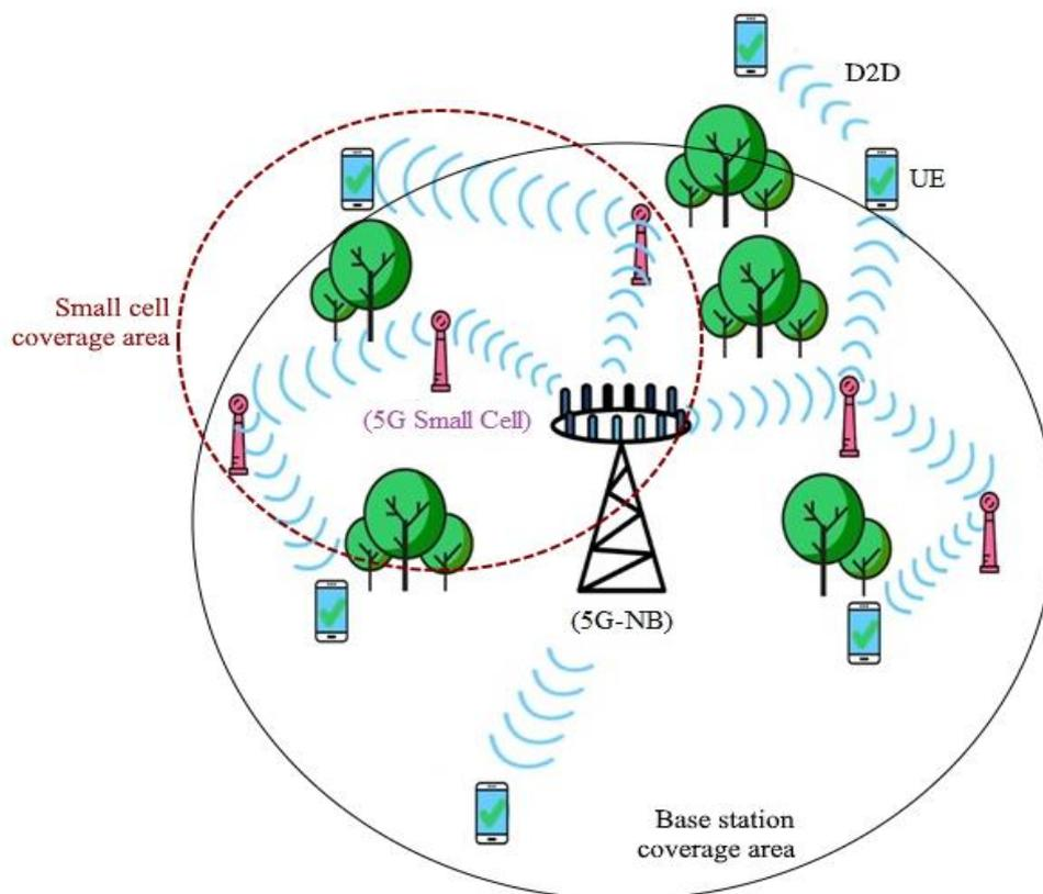
Figure 6. Visualized use principle of the 5G small cells and general network topology [12].
