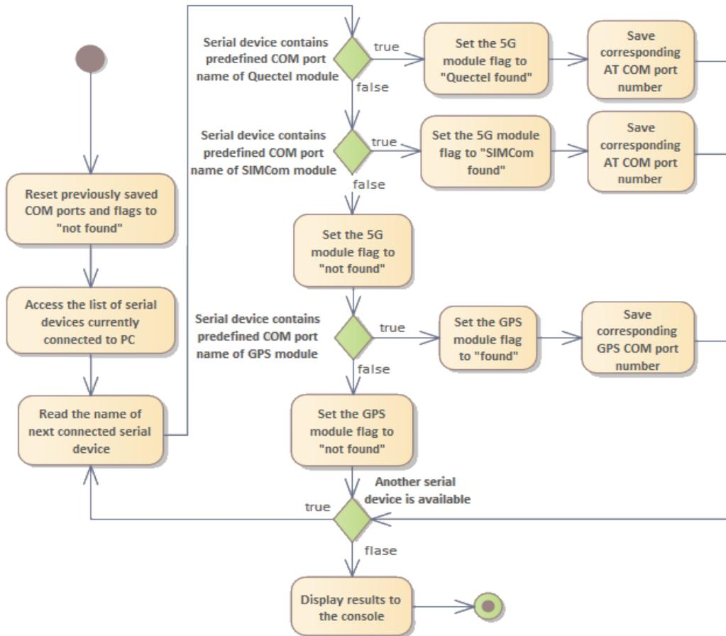
Figure 22. Activity diagram for the “COMFind” function.
