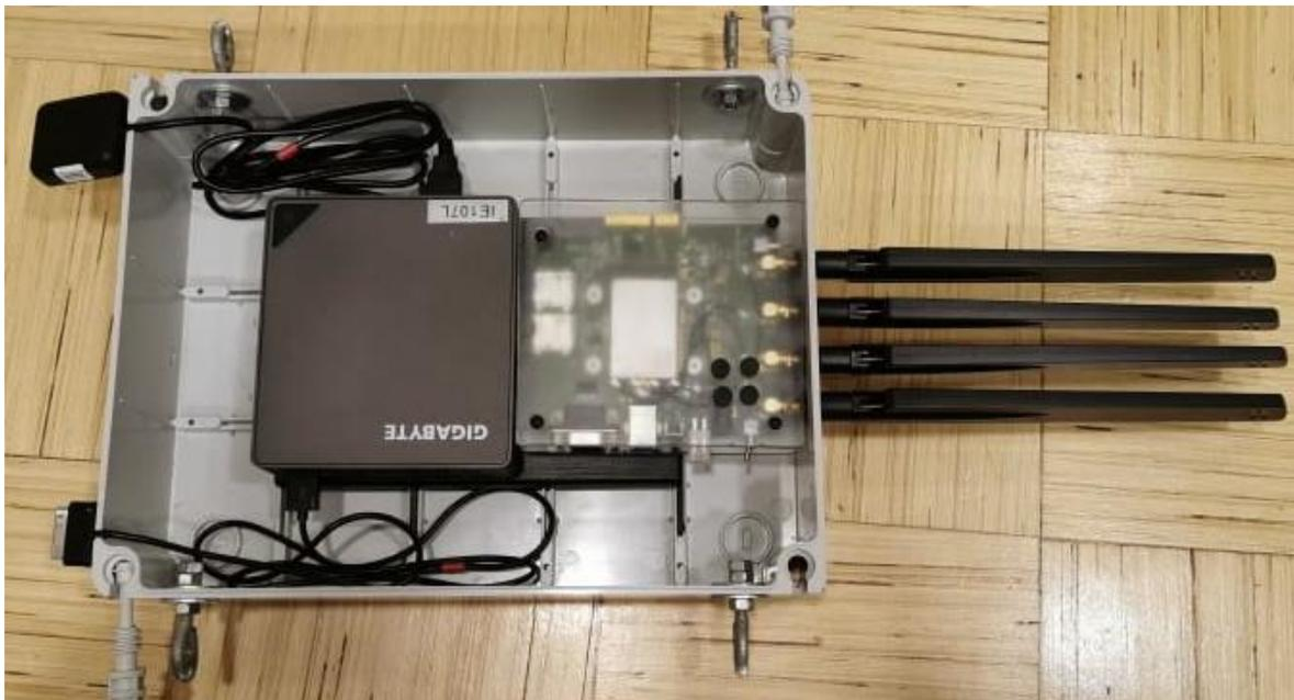
Figure 14. Implemented testbed setup inside the ABS plastic box.
