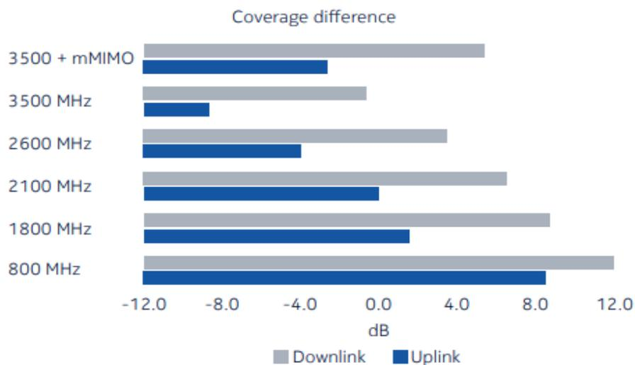
Figure 8. 5G coverage test results at the sub-6 GHz frequencies in comparison with 4G LTE performance (by Nokia) [16].
