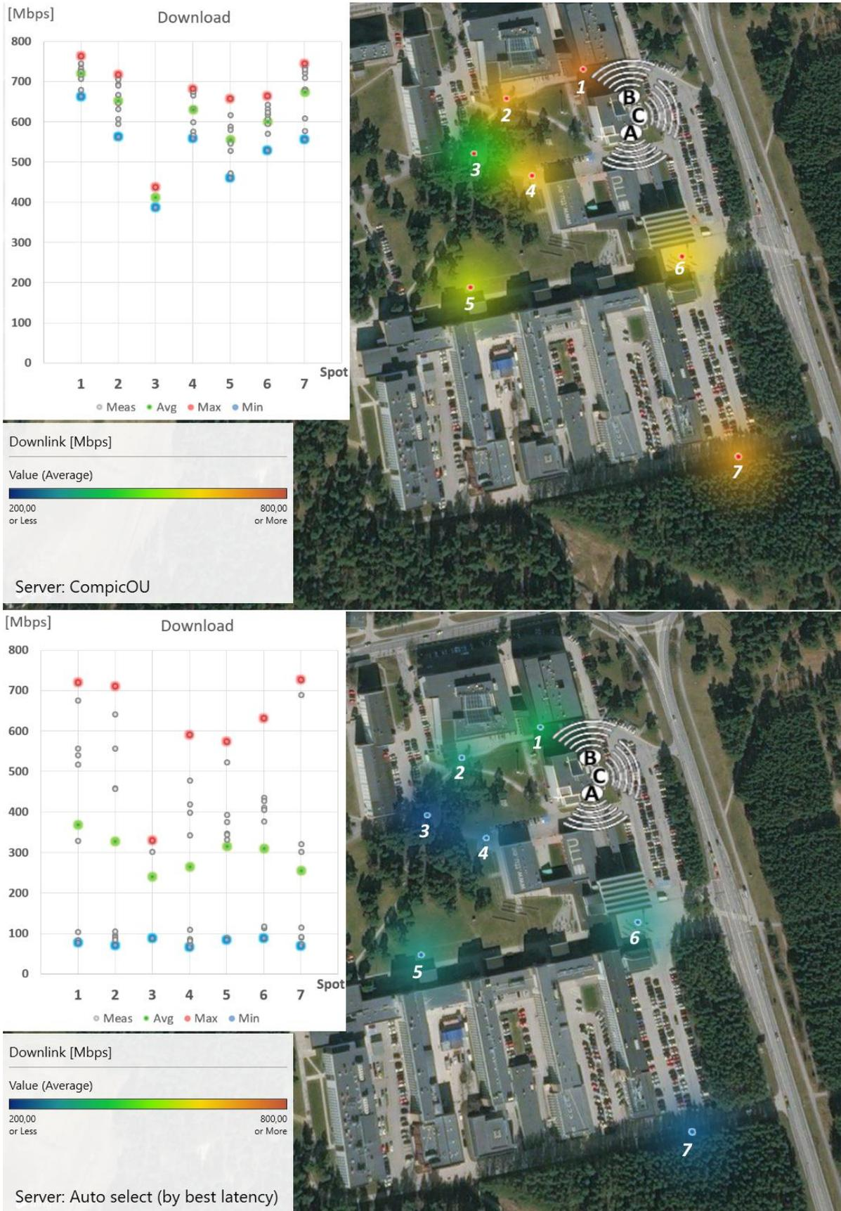
Figure 37. Heatmaps, based on average measured downlink speed for the “CompicOU” server (top), and for the automatically picked servers (bottom).
