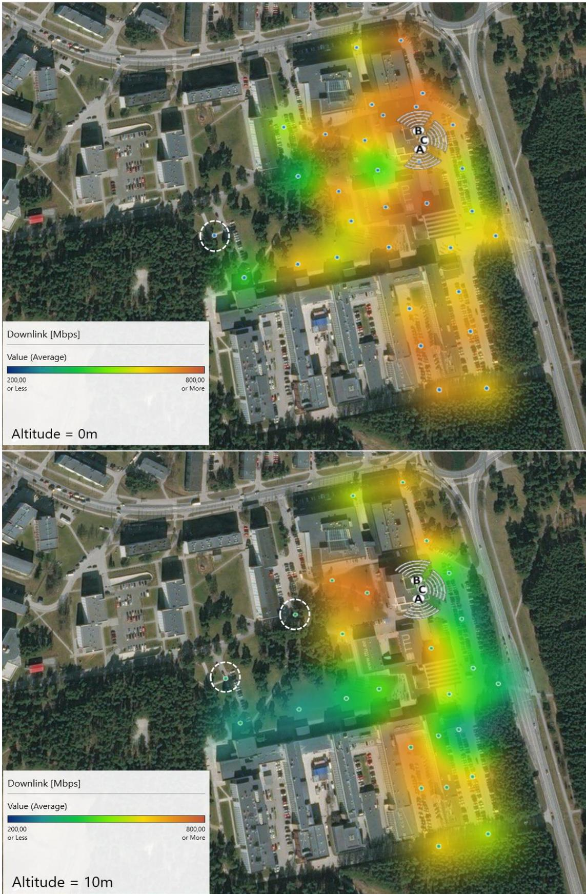
Figure 41. Heatmaps based on the measured downlink speed for 5G band within TUT campus area at the ground level (top), and 10 m altitude (bottom).
