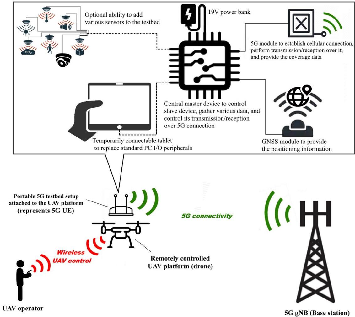
Figure 12. Full structural scheme of the implemented testbed, used for the aerial measurements.
