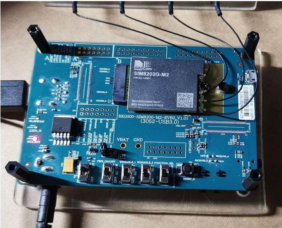
Figure 18. SIMCom SIM8202G 5G module with 8XG000-SIM8200-M2-EVB2 development board.
