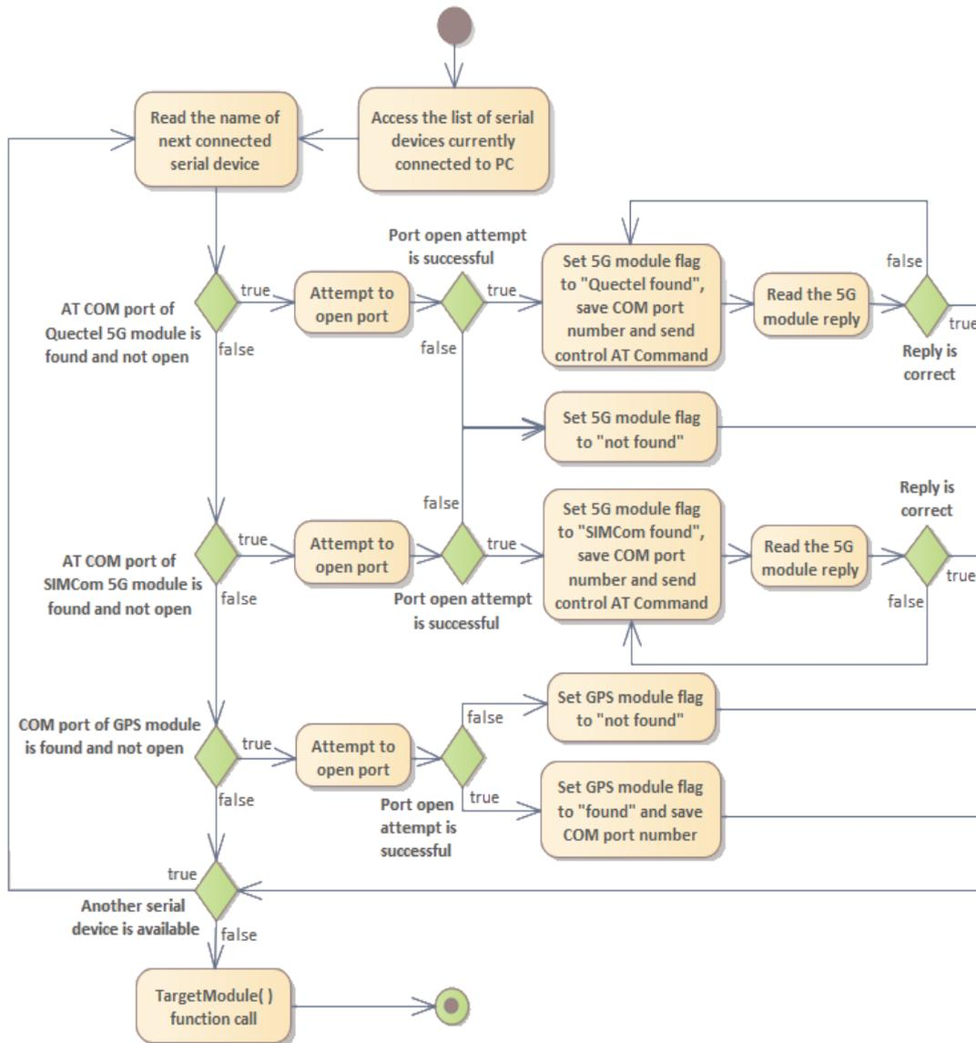
Figure 26. Activity diagram for the “COMRepair” function.
