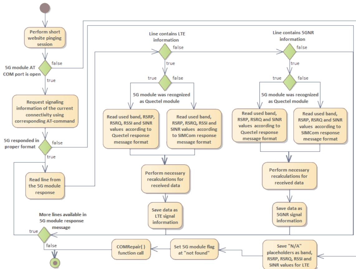
Figure 27. Activity diagram for the “GetSignalData” function.
