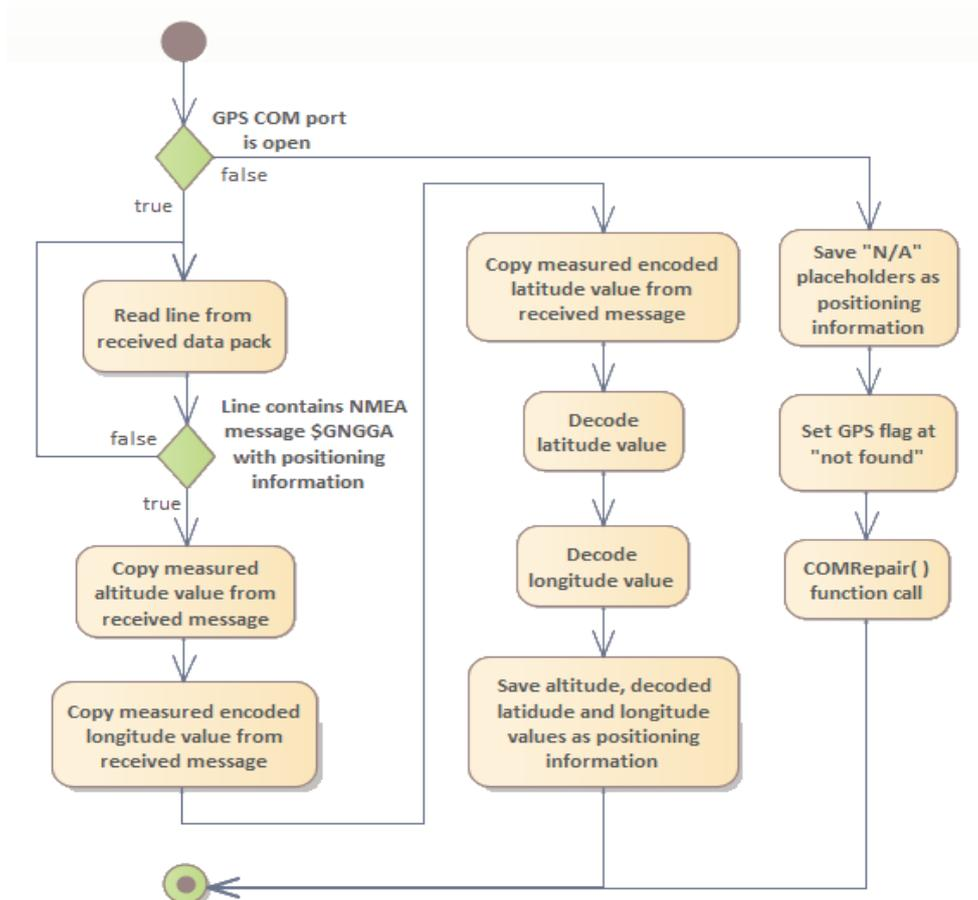
Figure 25. Activity diagram for the “GetLocationData” function.
