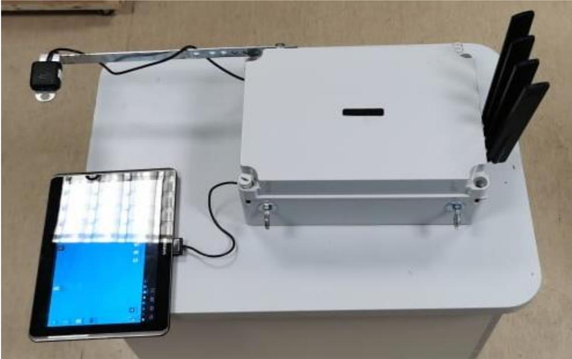
Figure 15. Testbed setup packed in a plastic box and prepared to be attached to the drone.
