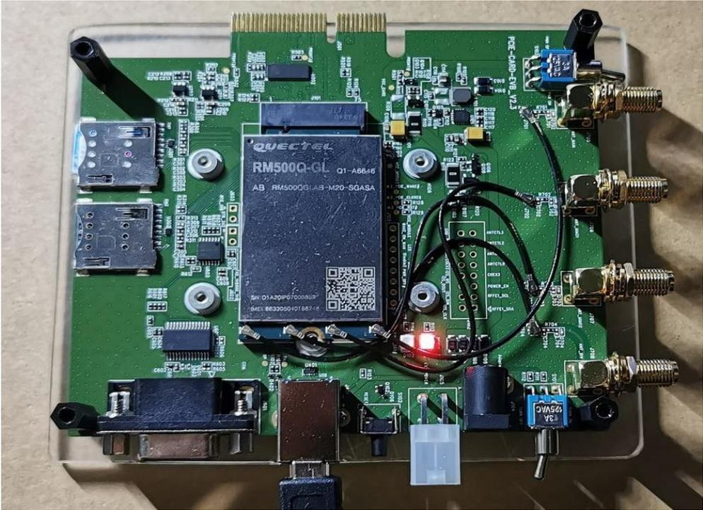
Figure 17. Quectel RM500Q-GL 5G module with PCIECARDEVB-KIT development board.
