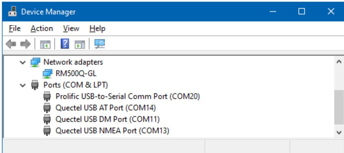
Figure 21. Windows device manager showing connected GNSS and 5G modules.
