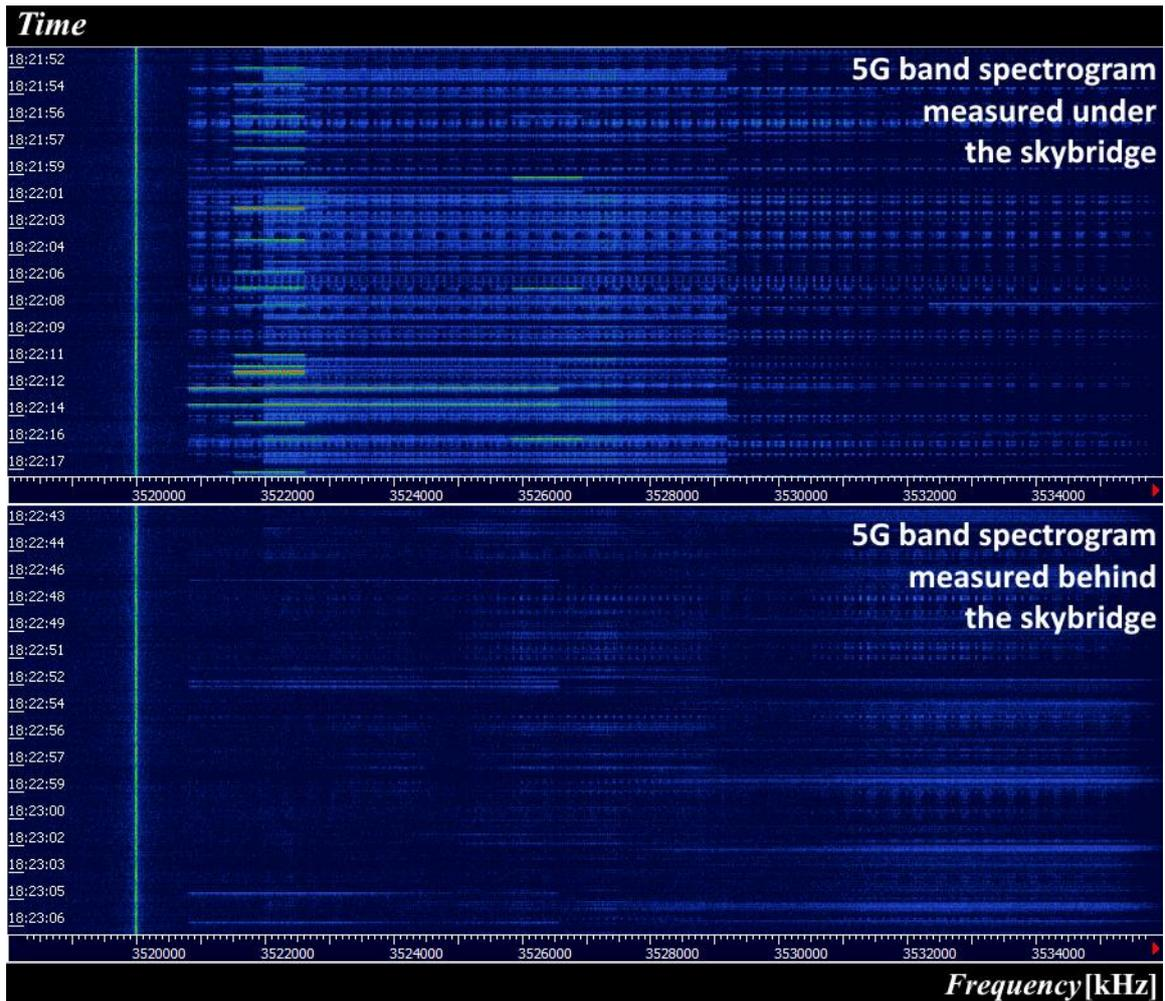
Figure 33. Spectrogram of the 5G band, measured under the skybridge (up), and behind the skybridge (bottom), displayed in HSDR software.
