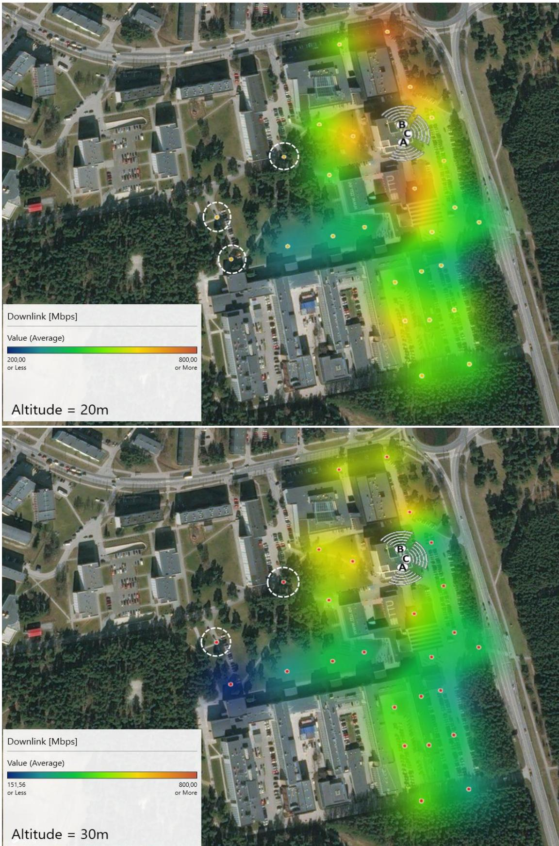
Figure 42. Heatmaps based on the measured downlink speed for 5G band within TUT campus area at the 20 m altitude (top), and 30 m altitude (bottom).
