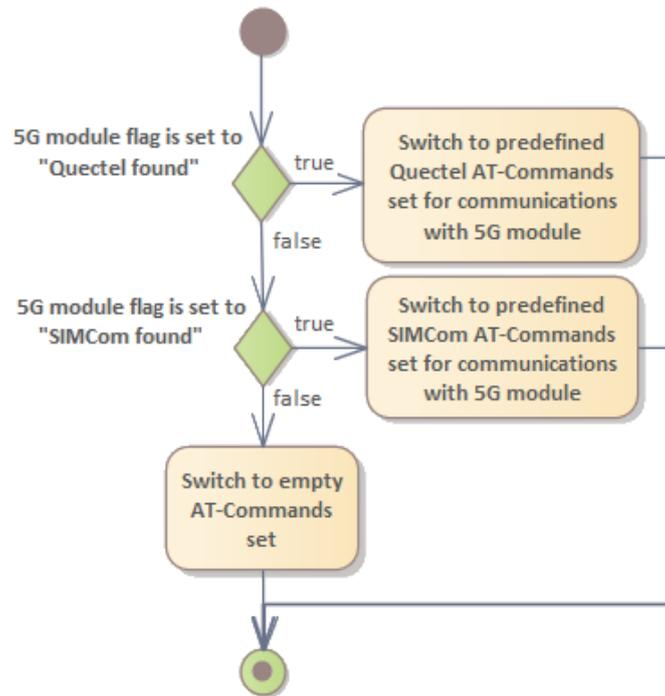
Figure 23. Activity diagram for the “TargetModule” function.
