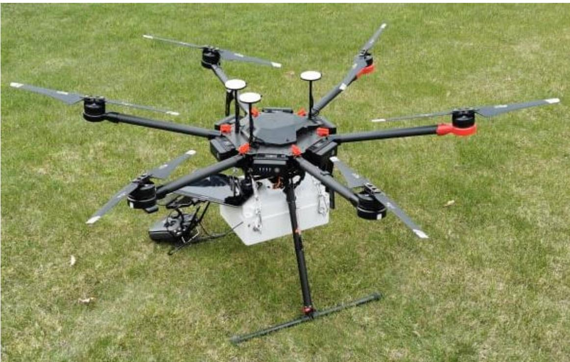
Figure 16. Used DJI MATRICE 600 Pro drone with the attached testbed setup.
