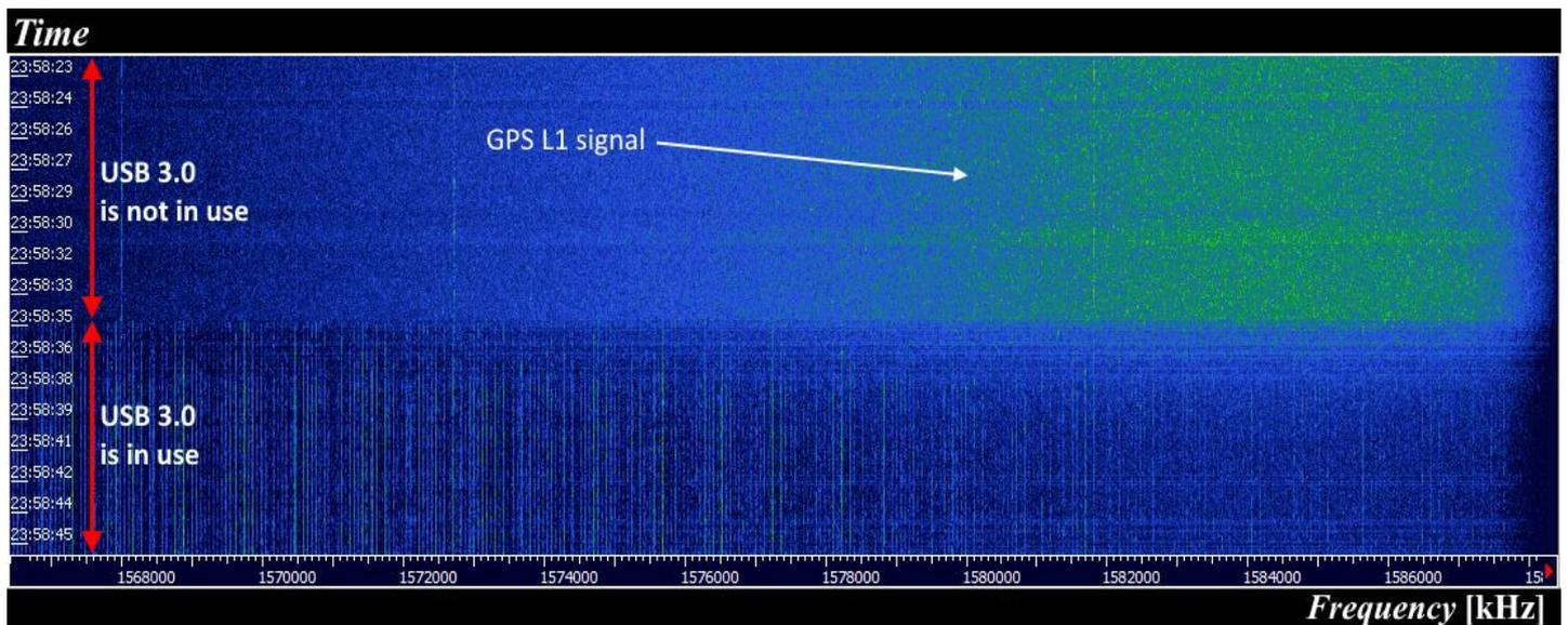
Figure 46. Spectrogram of the captured USB 3.0 RF interference at the GPS L1 frequency, displayed in HSDR software environment.
