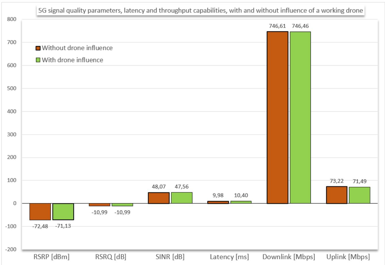
Figure 45. Column chart of the measured signal quality, latency, and throughput parameters with and without the possible influence of a drone.
