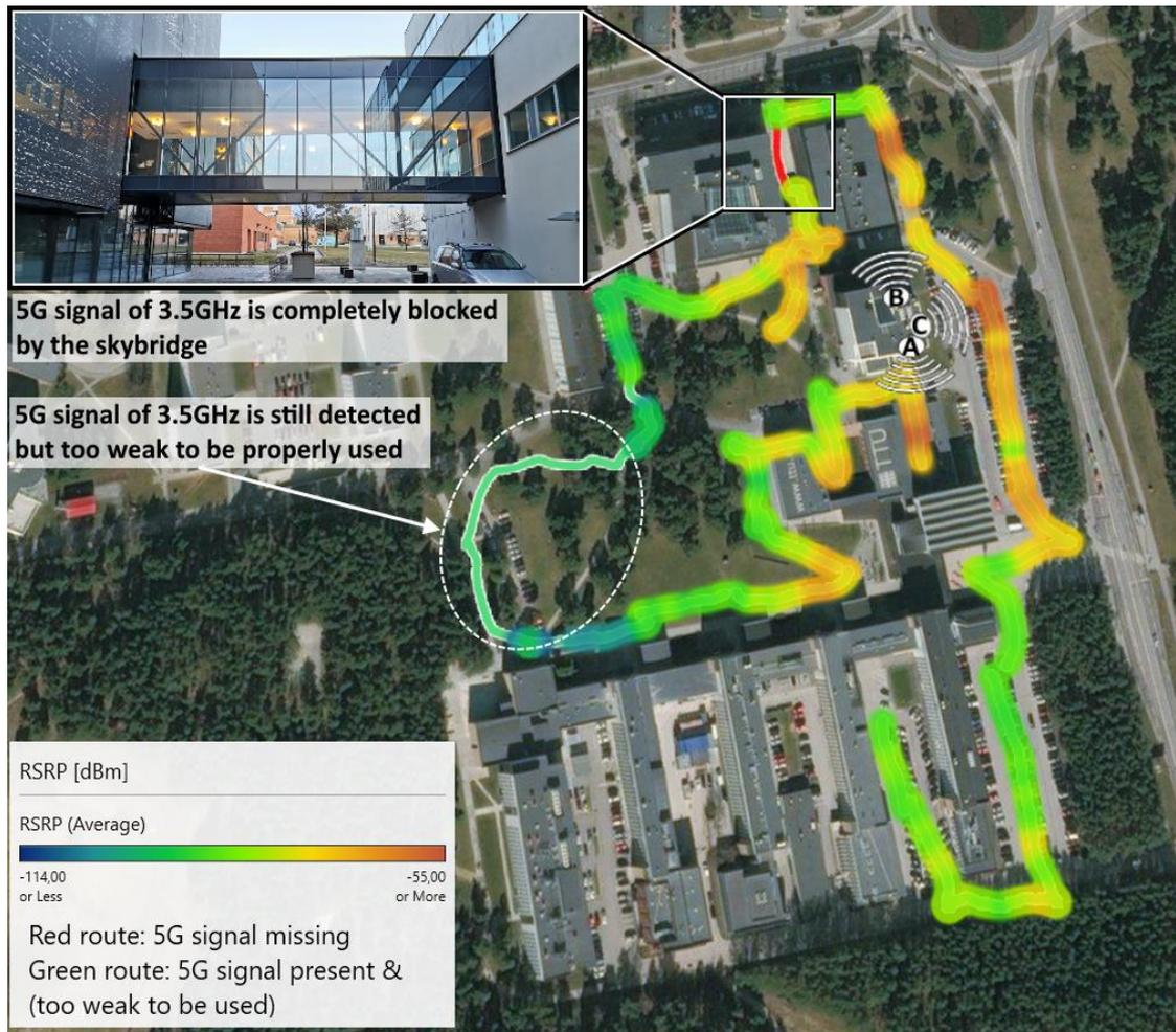
Figure 32. 5G signal coverage heatmap based on the measured SS-RSRP within TUT campus area.
