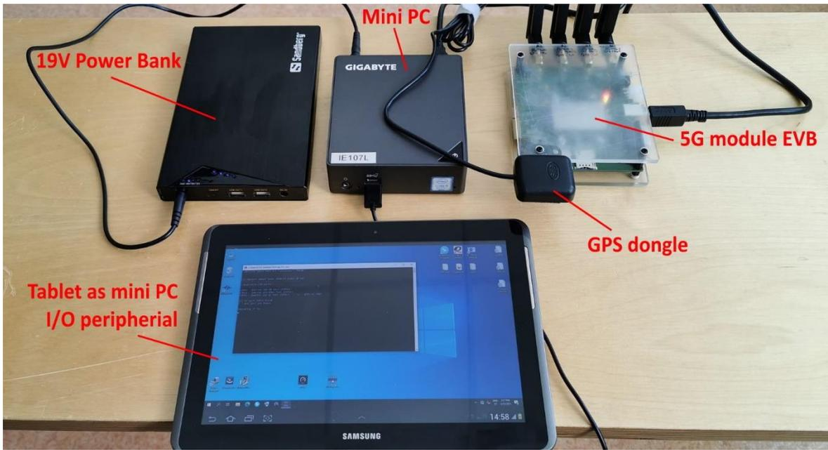
Figure 13. Hardware used in the implemented testbed setup.
