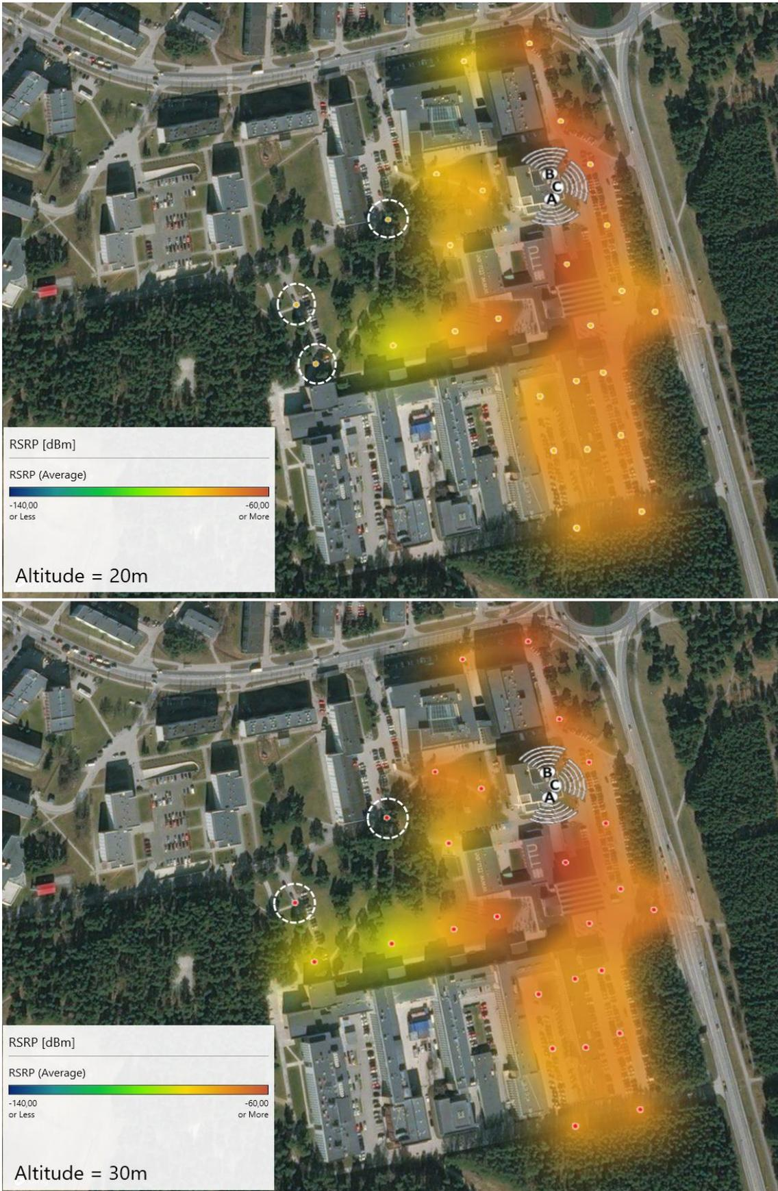
Figure 40. 5G signal coverage heatmaps based on the measured SS-RSRP within TUT campus area at the 20 m altitude (top), and 30 m altitude (bottom).
