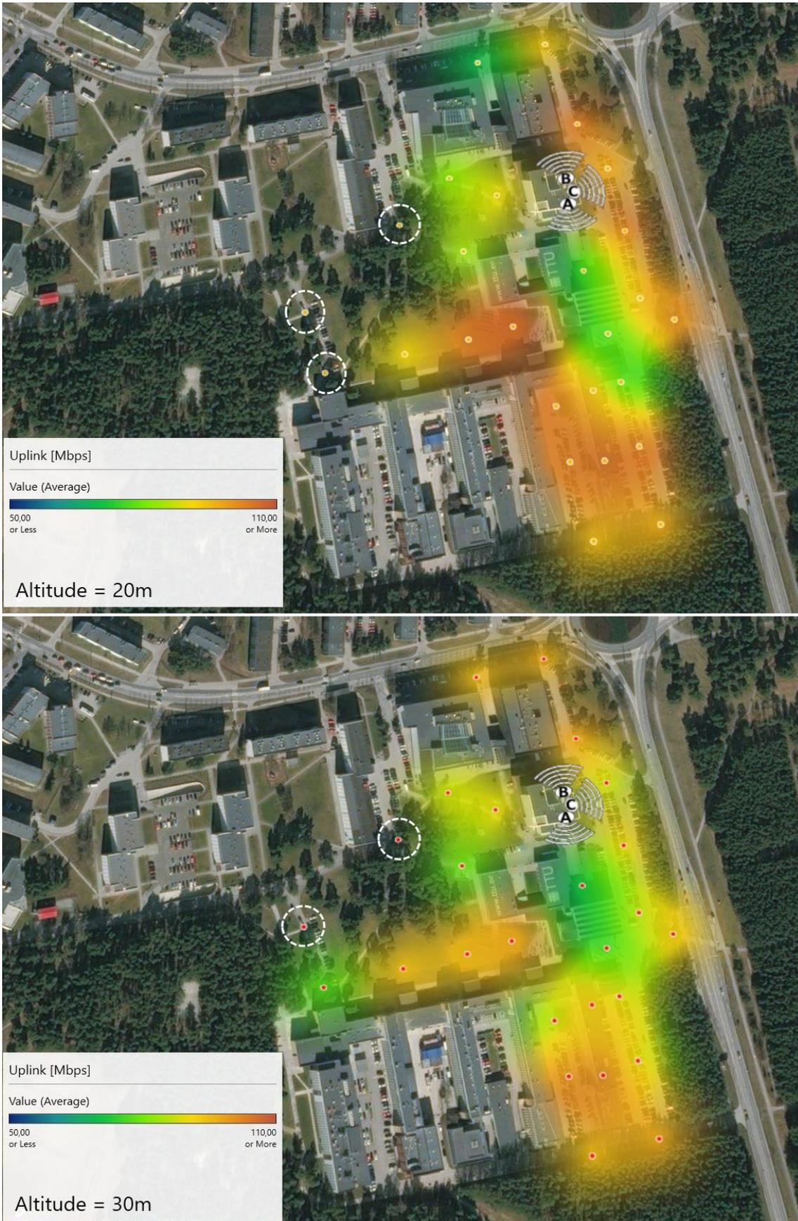
Figure 44. Heatmaps based on the measured downlink speed using 5G band within TUT campus area at the 20 m altitude (top), and 30 m altitude (bottom).
