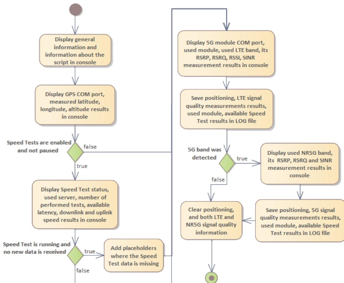
Figure 28. Activity diagram for the “DisplayData” function.
