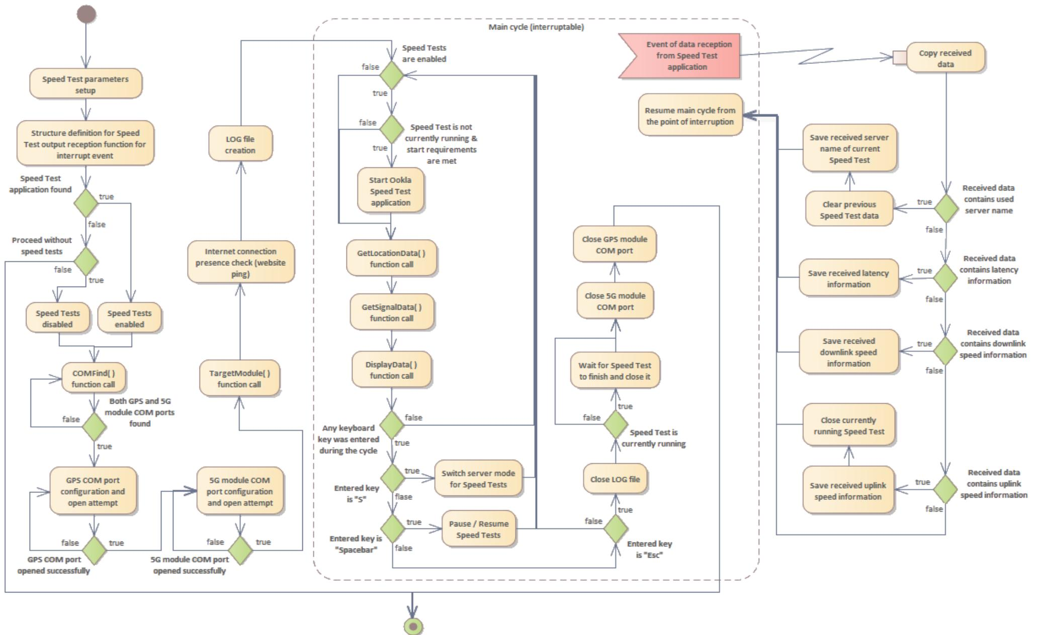
Figure 20. Activity diagram for the main function of the implemented program.
