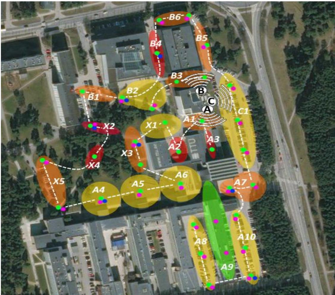
Figure 31. TUT campus area map with marked 5G antennas, key areas for measurements, exact measurement spots and routes of planned coverage and throughput measurements.
