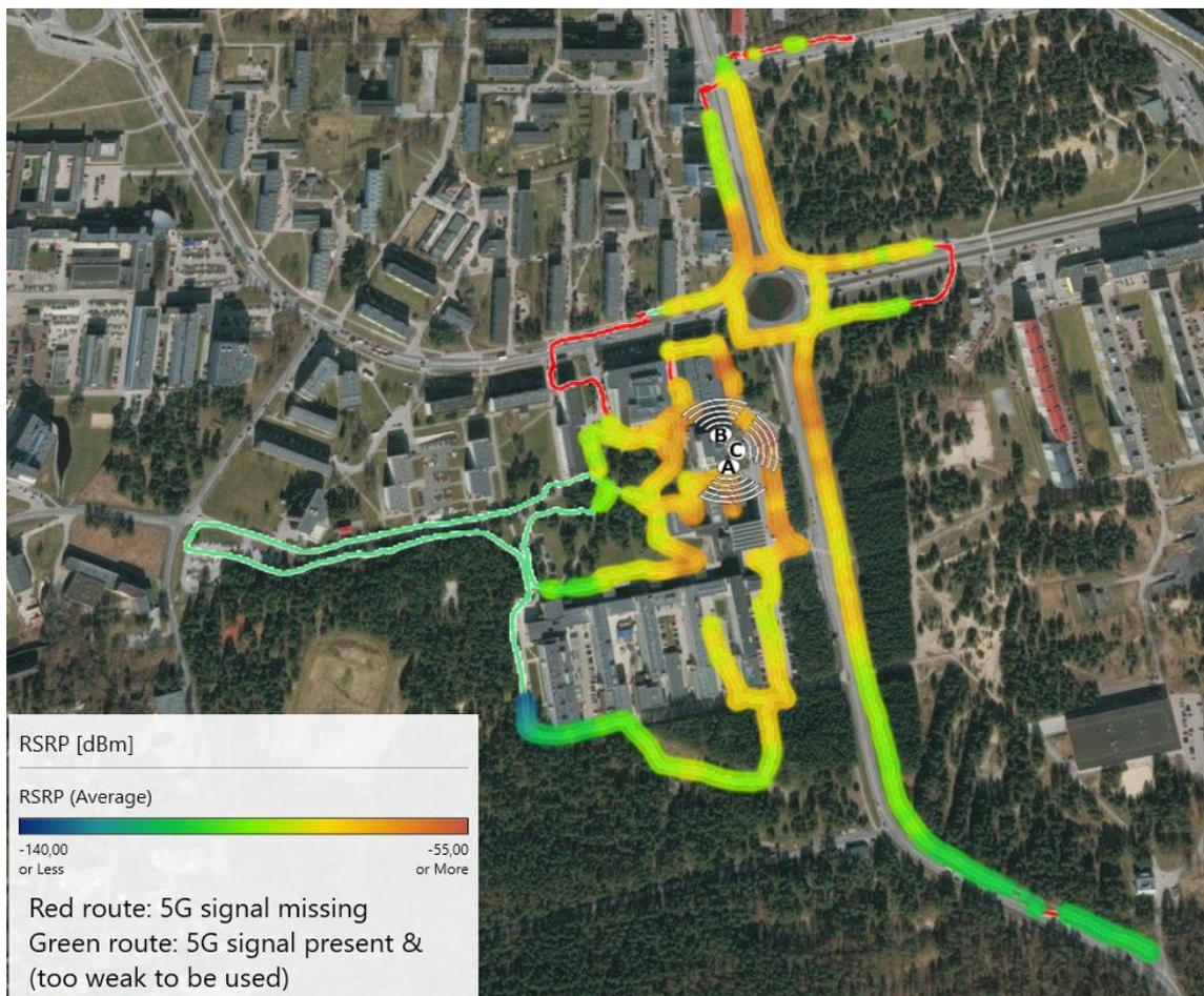
Figure 34. 5G signal coverage heatmap based on the measured SS-RSRP within and slightly outside TUT campus area.
