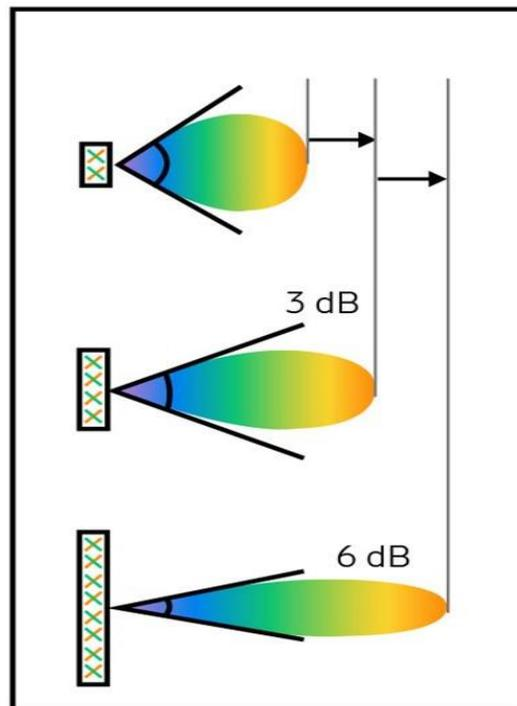
Figure 5. Visualization of the gain and width of the beam generated by different number of cooperative antennas in the array [11].
