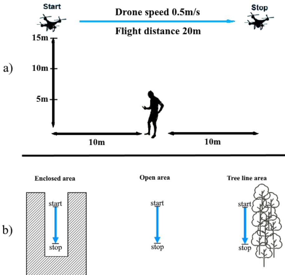
Figure 9. (a) Illustrated methodology for the drone delivered 5G connectivity tests and (b) illustrated areas of testing [23].
