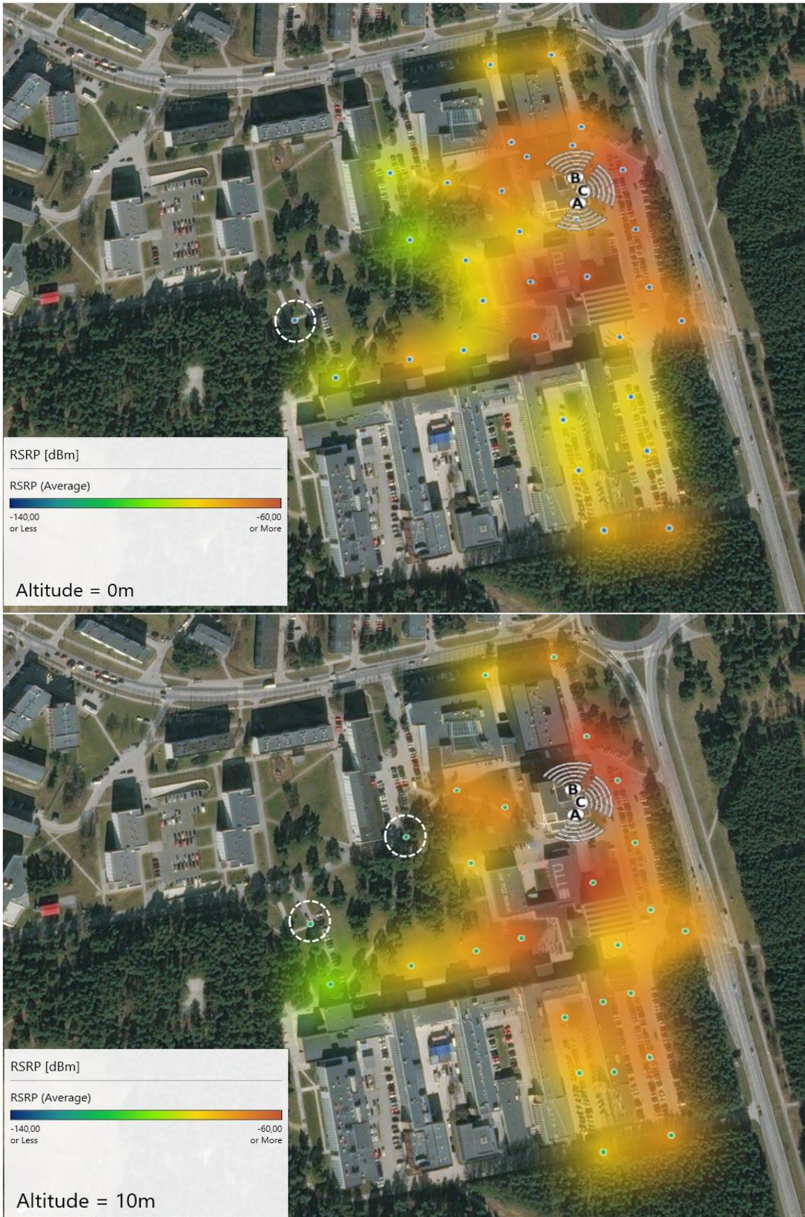
Figure 39. 5G signal coverage heatmaps based on the measured SS-RSRP within TUT campus area at the ground level (top), and 10 m altitude (bottom).
