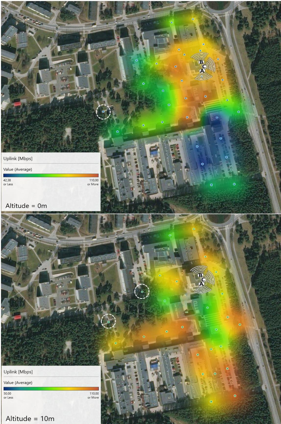
Figure 43. Heatmaps based on the measured uplink speed using 5G band within TUT campus area at the ground level (top), and 10 m altitude (bottom).
