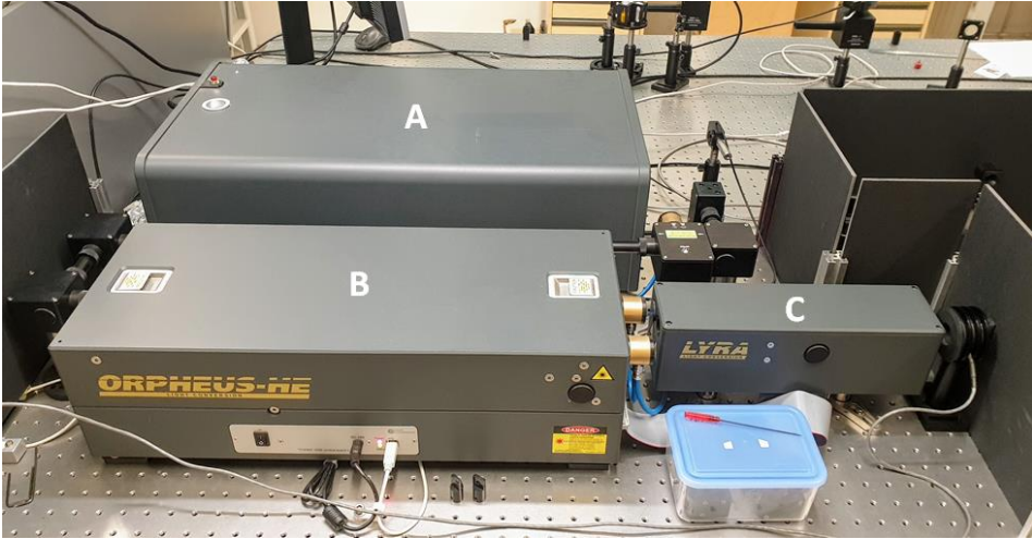
Figure 11: Tabletop layout of the femtosecond pulse laser system (Light Conversion). A – PHAROS-SP pump laser, B – ORPHEUS-HE optical parametric amplifier, C – LYRA second harmonic generator.
