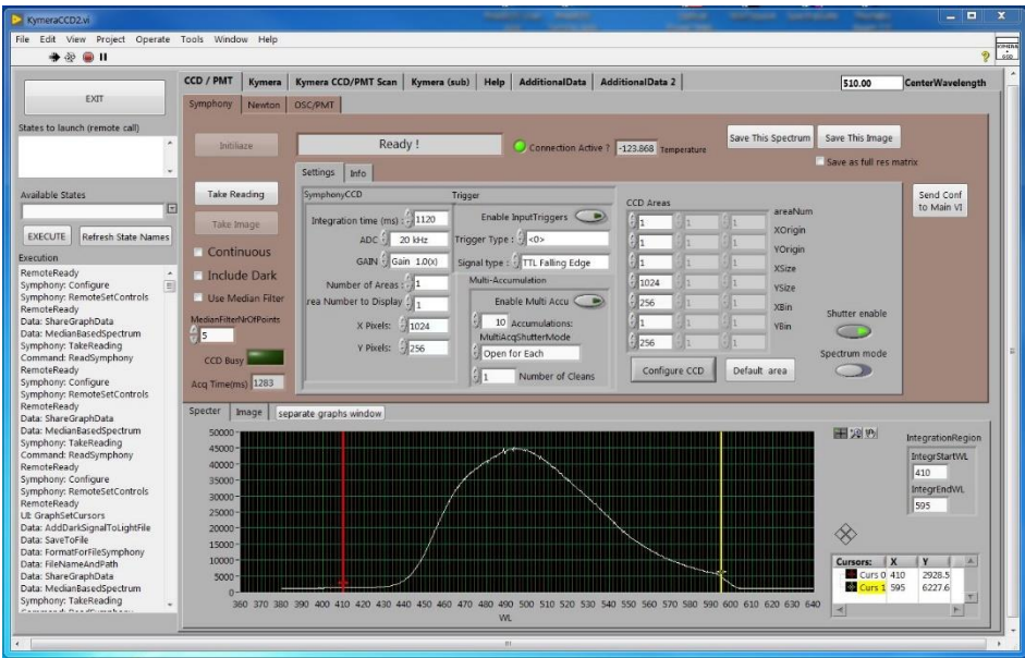
Figure 42: LabView Symphony CCD control window, integrated fluorescence is collected between red, \lambda_{min} , and yellow, \lambda_{max} , vertical markers at the bottom graph. The user can also set the integration time (1120 ms at the current acquisition) and amplification factor (1.0).
