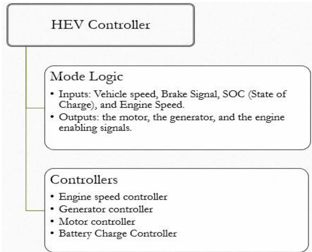
Figure 4.2. Hybrid Electric Vehicle Control Structure
