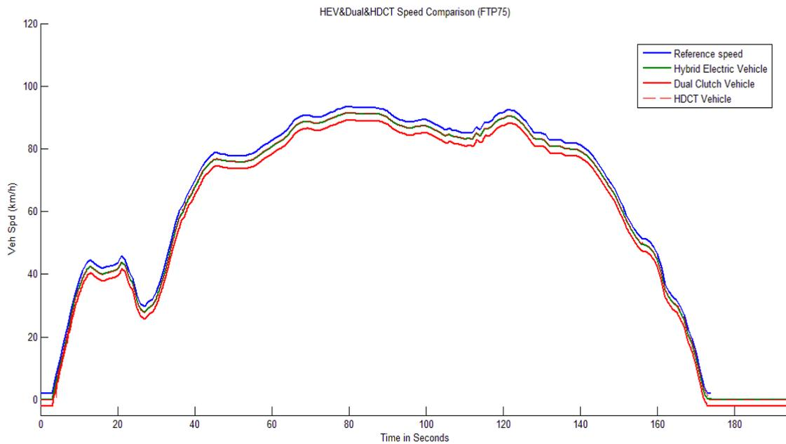
Figure 6.6. Comparison between the models and reference speed (FTP75, Cold Start)
