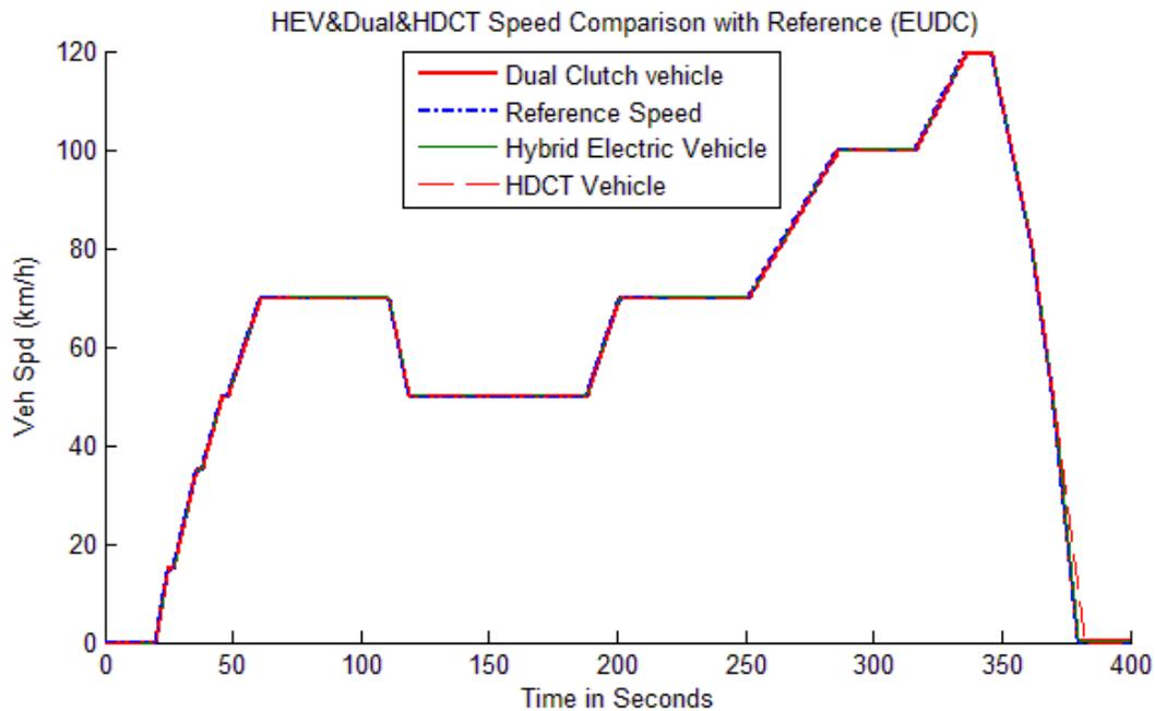
Figure 6.24. Comparison between the models and reference speed (EUDC)
