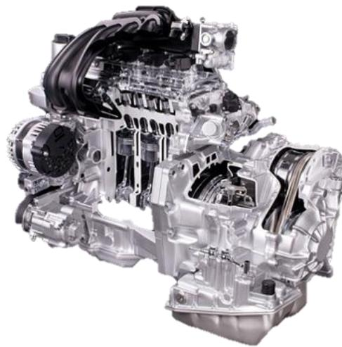
Figure 2.7. Nissan HR15DE engine with Xtronic CVT [27]
