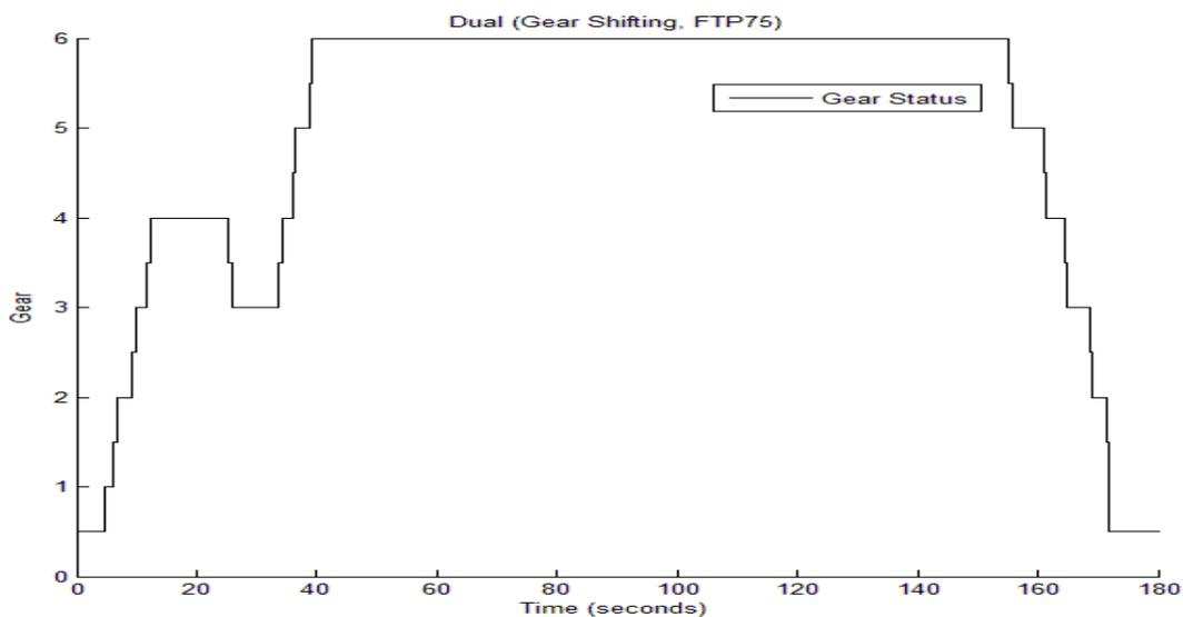
Figure 6.25. Gear-shifting for Dual Clutch Transmission Conventional Vehicle (FTP75, Cold Start)
