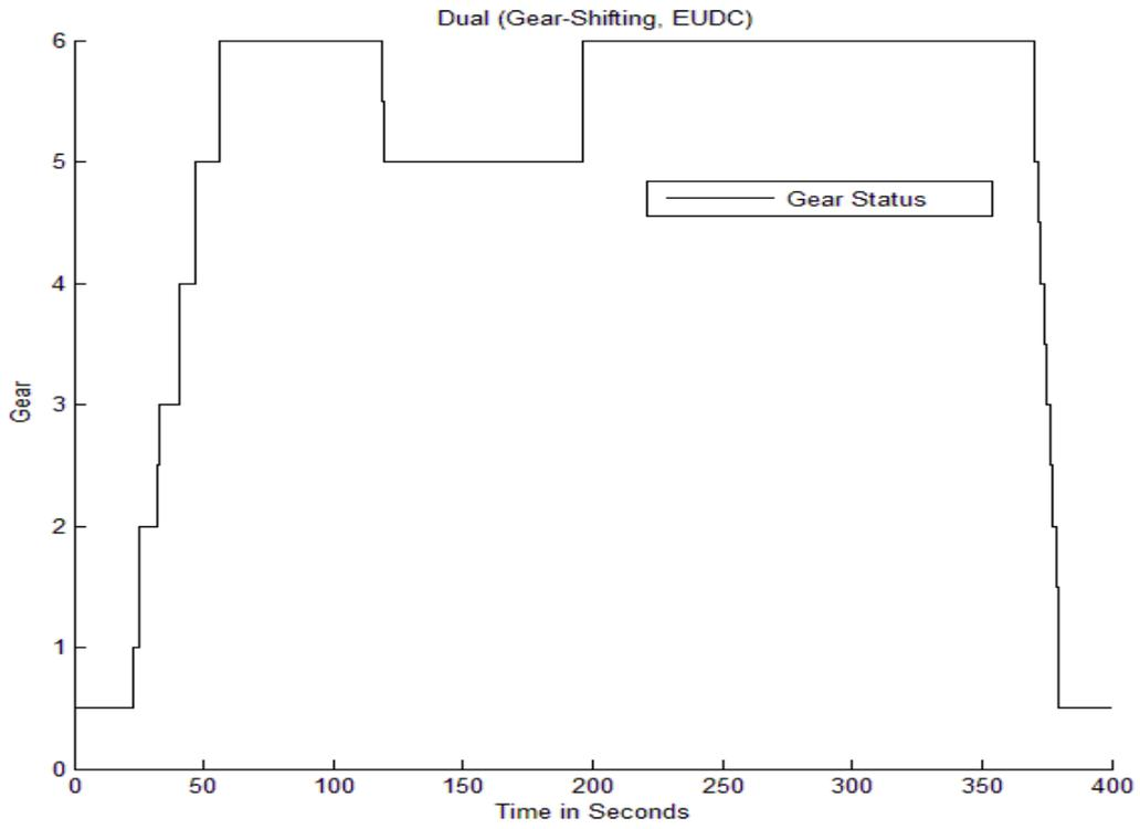
Figure 6.29. Gear-shifting for Dual Clutch Transmission Conventional Vehicle (EUDC)
