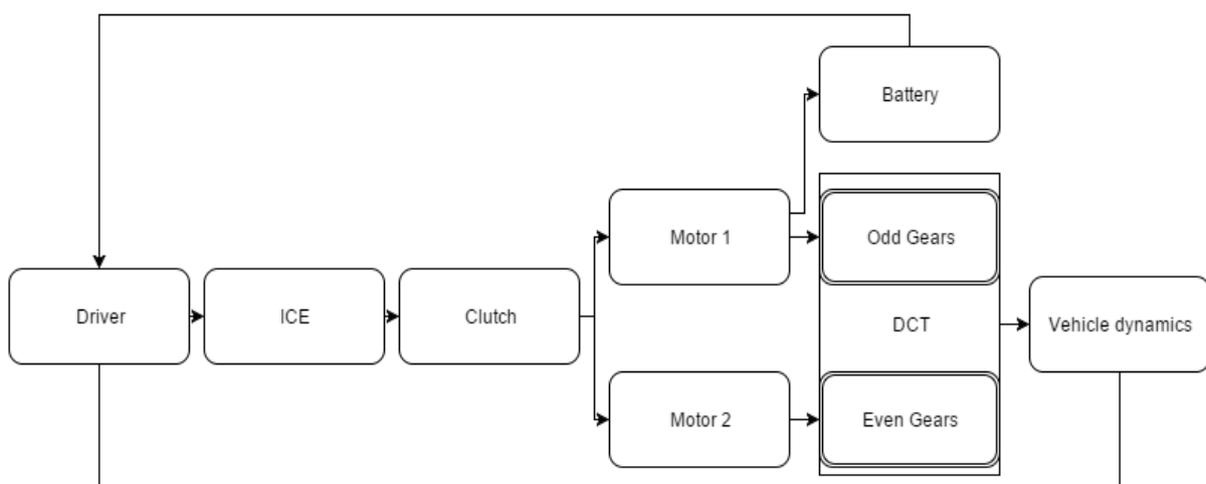
Figure 5.1. Hybrid Electric Vehicle model including Dual Clutch Transmission
