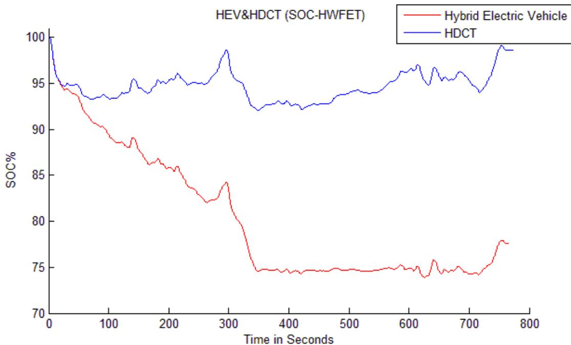
Figure 6.31. State of Charge comparison for HDCTV and HEV (HWFET)
