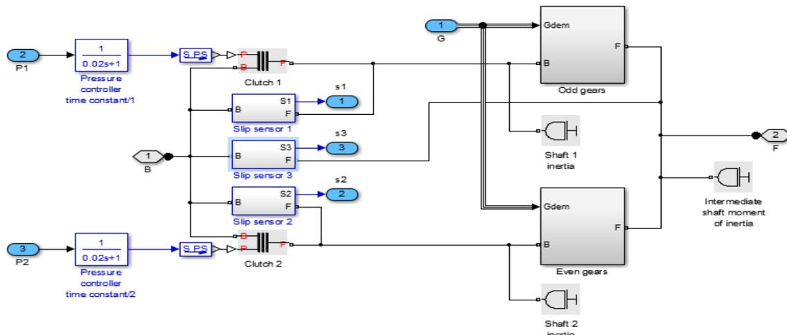
Figure 3.2. Dual Clutch Transmission model in Simulink
