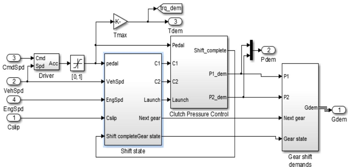
Figure 5.2. Transmission Controller of Dual Clutch Transmission
