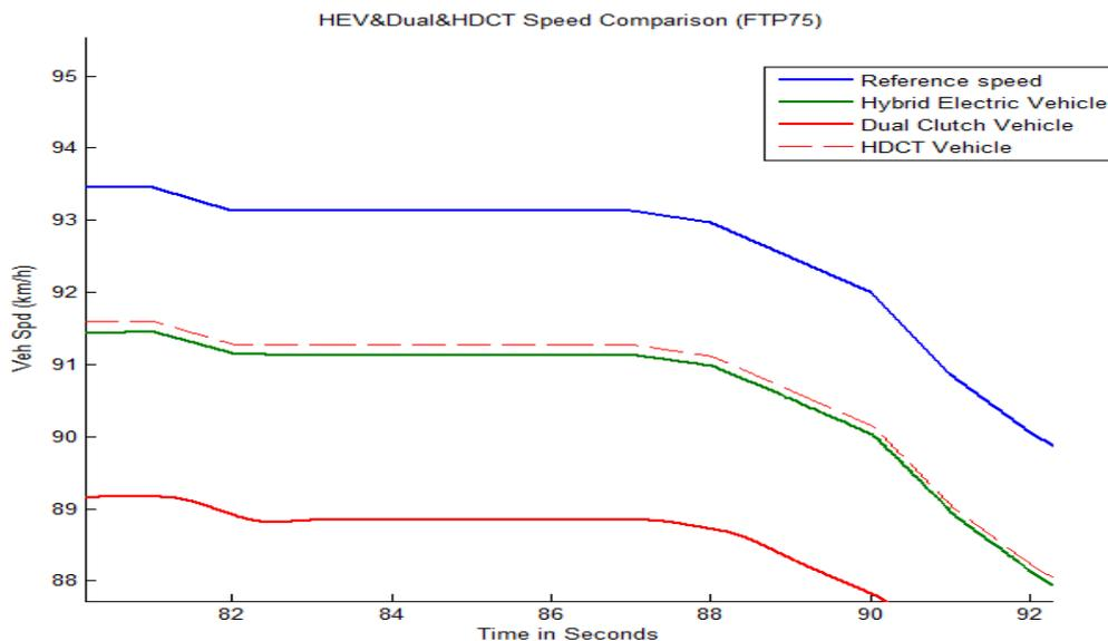
Figure 7.1. Chosen section of comparison between the three models, as (FTP75, Cold Start) is the reference drive cycle
