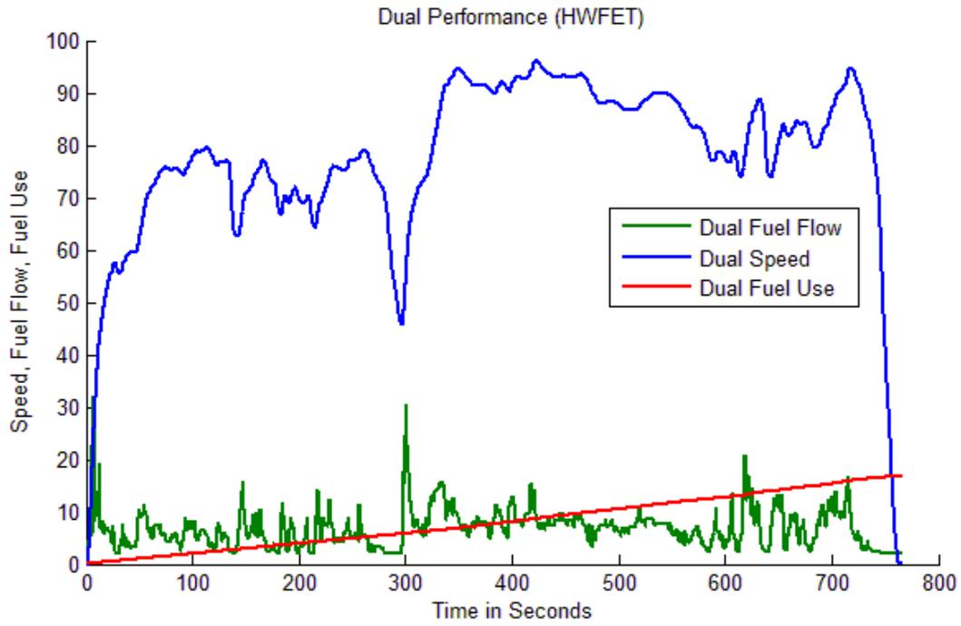
Figure 6.14. Dual Clutch Transmission Conventional Vehicle's (Performance – Fuel Flow – Fuel Use) (HWFET)
