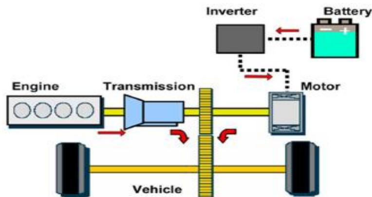
Figure 2.9. Parallel HEV configuration [32]
