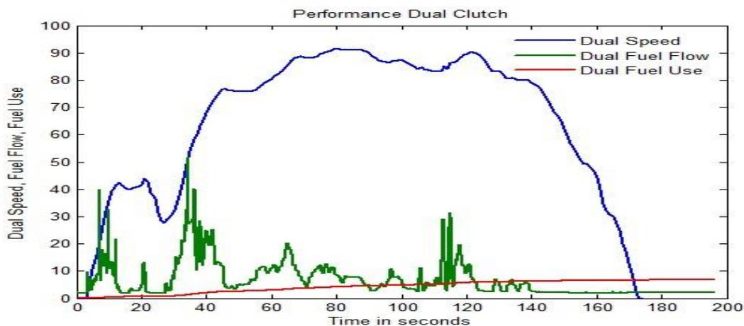
Figure 6.2. Dual Clutch Transmission Conventional Vehicle's (Performance – Fuel Flow – Fuel Use) (FTP75, Cold Start)
