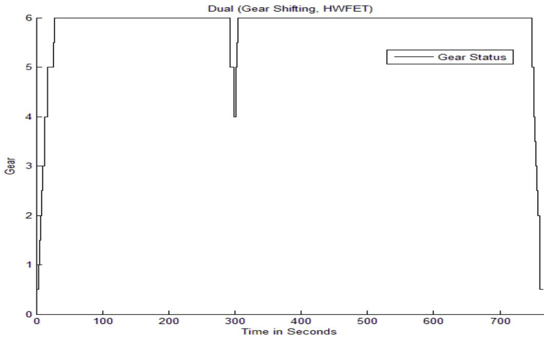
Figure 6.27. Gear-shifting for Dual Clutch Transmission Conventional Vehicle (HWFET)
