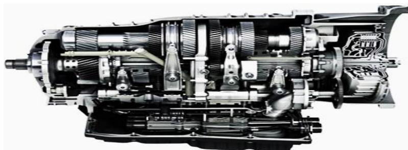
Figure 2.6. VW/Audi's DSG [26]
