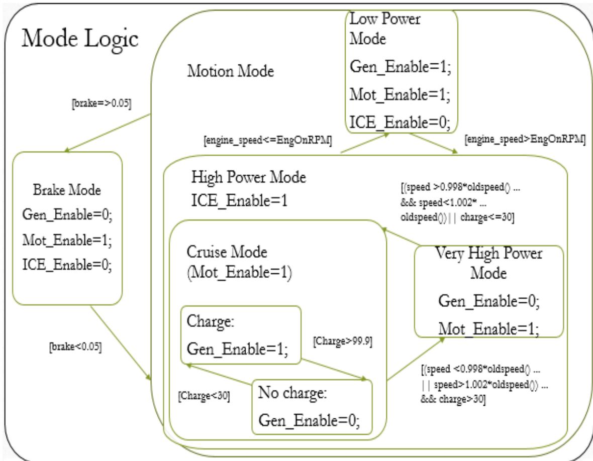
Figure 4.3. Mode Logic Block
