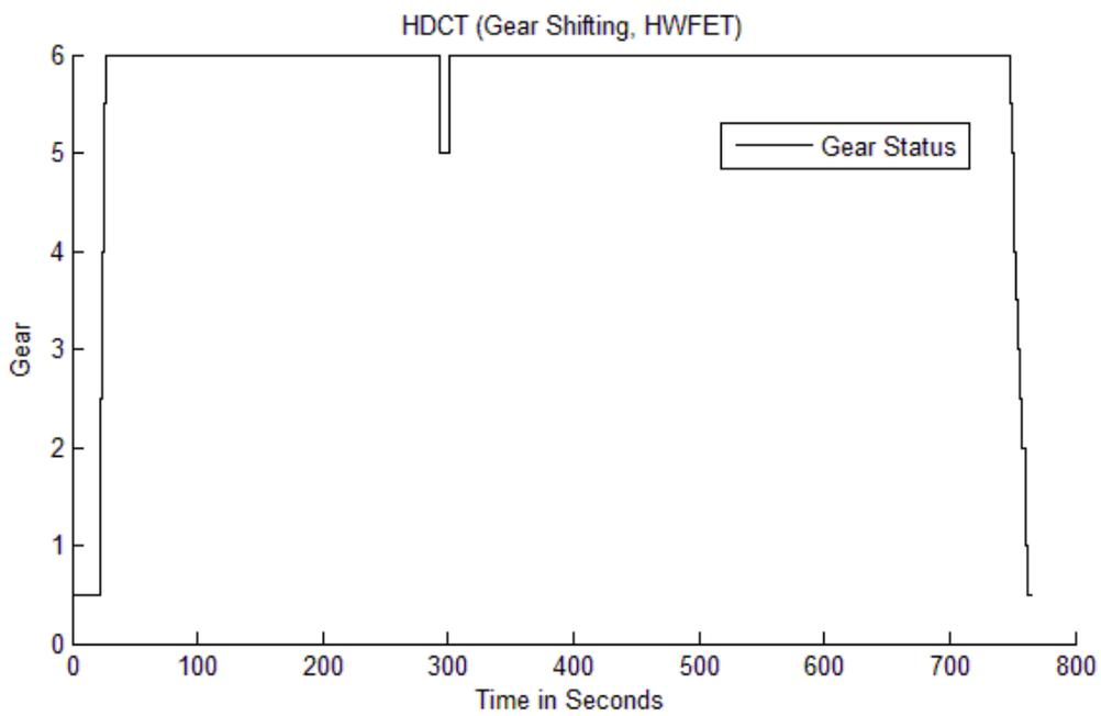
Figure 6.28. Gear-shifting for Dual Clutch Transmission Hybrid Vehicle (HWFET)
