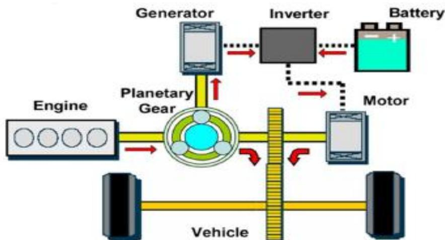
Figure 2.10. Series-Parallel Configuration [32]
