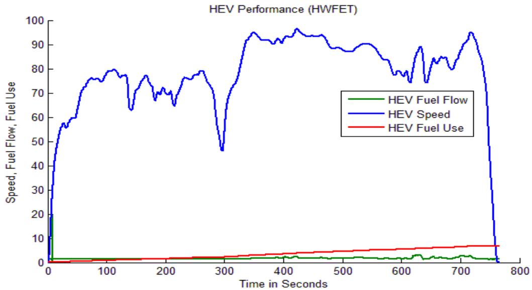
Figure 6.15. Hybrid Electric Vehicle (Performance – Fuel Flow – Fuel Use) (HWFET)
