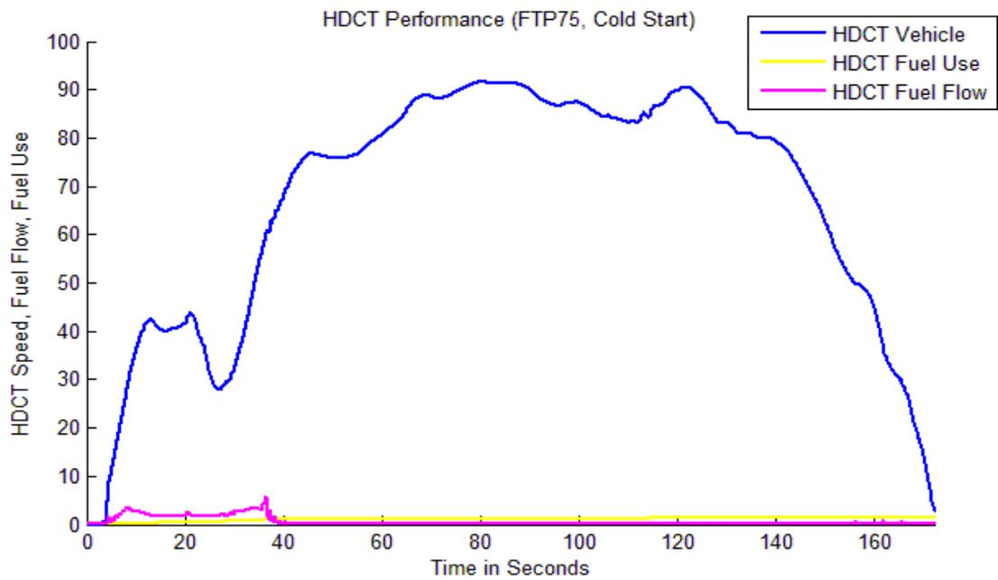
Figure 6.4. Hybrid Electric Vehicle with Dual Clutch Transmission (Performance – Fuel Flow – Fuel Use) (FTP75, Cold Start)
