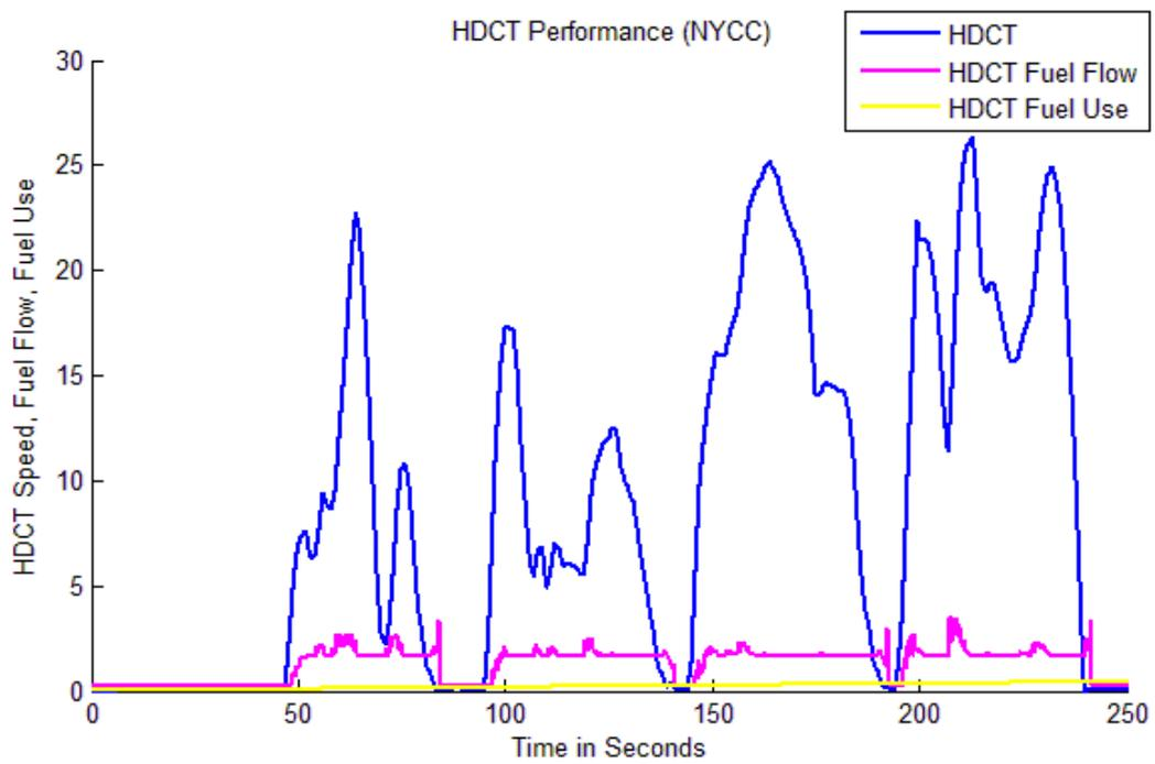
Figure 6.10. Hybrid Electric Vehicle with Dual Clutch Transmission (Performance – Fuel Flow – Fuel Use) (NYCC)
