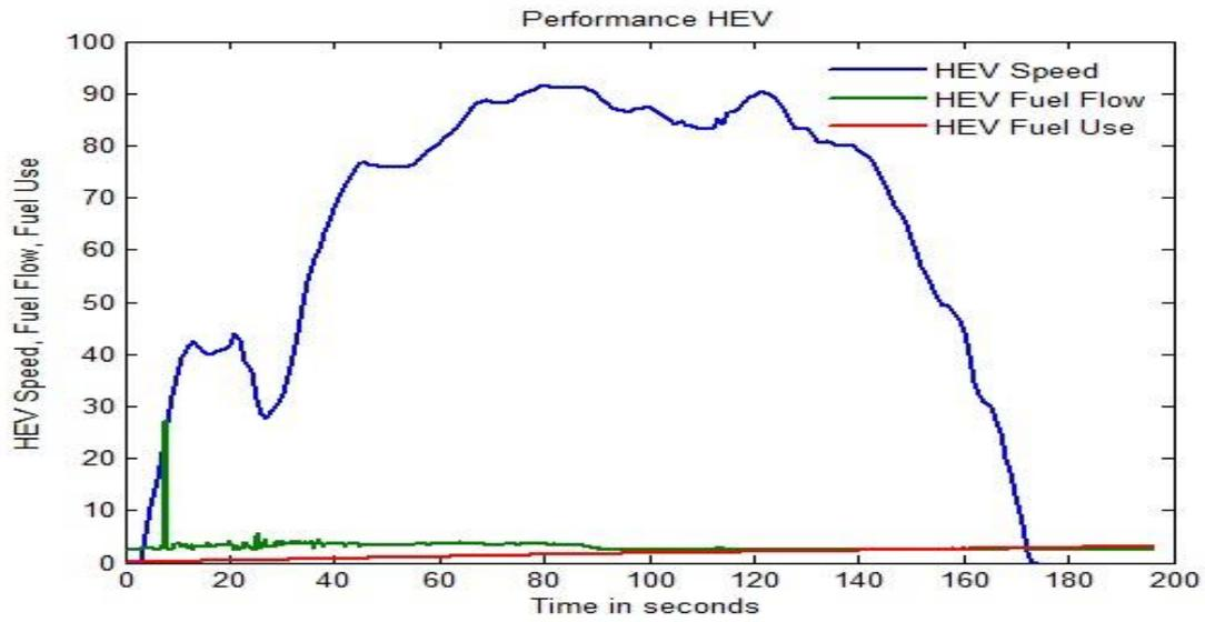
Figure 6.3. Hybrid Electric Vehicle (Performance – Fuel Flow – Fuel Use) (FTP75, Cold Start)
