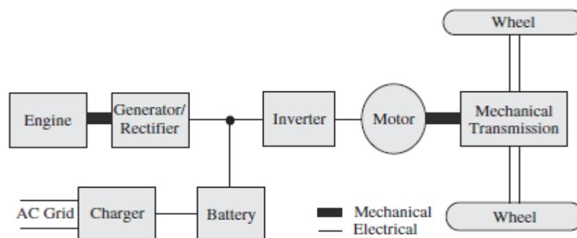
Figure 2.11. Series architecture of PHEV [3]
