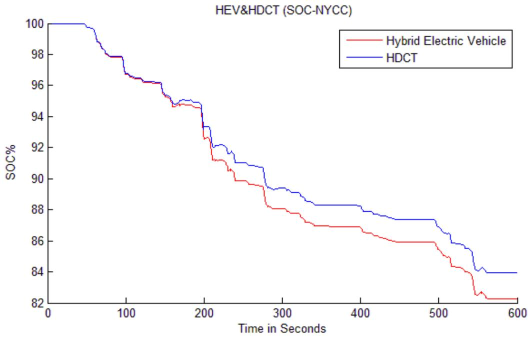
Figure 6.32. State of Charge comparison for HDCTV and HEV (NYCC)
