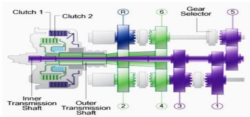
Figure 2.5. Six-speed Dual Clutch Transmission [23]
