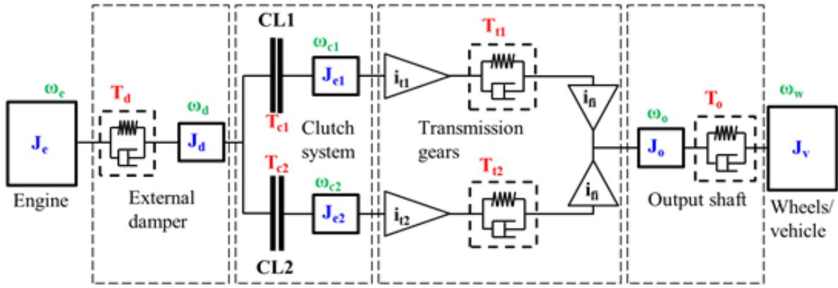
Figure 3.1. Powertrain model including Dual Clutch Transmission [35]
