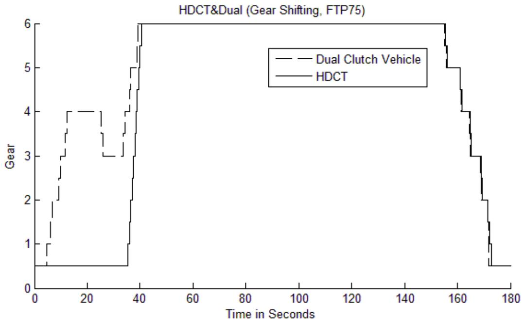
Figure 7.5. Gear Status comparison between HDCT&DCVT (FTP75, Cold Start)
