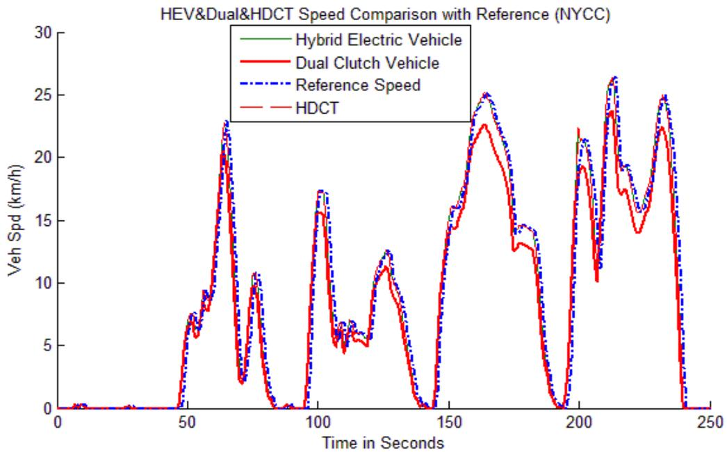
Figure 6.12. Comparison between the models and reference speed (NYCC)
