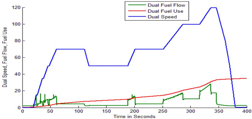
Figure 6.20. Dual Clutch Transmission Conventional Vehicle's (Performance – Fuel Flow – Fuel Use) (EUDC)
