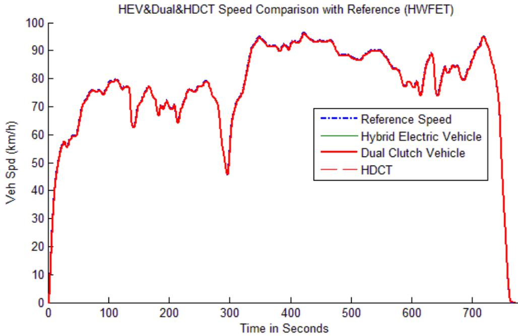
Figure 6.18. Comparison between the models and reference speed (HWFET)
