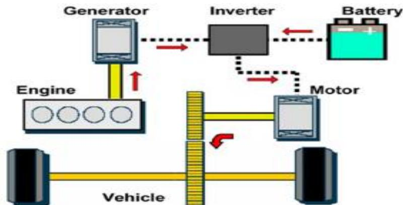
Figure 2.8. Series HEV configuration [32]
