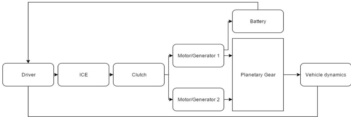
Figure 4.1. Hybrid Electric Vehicle model
