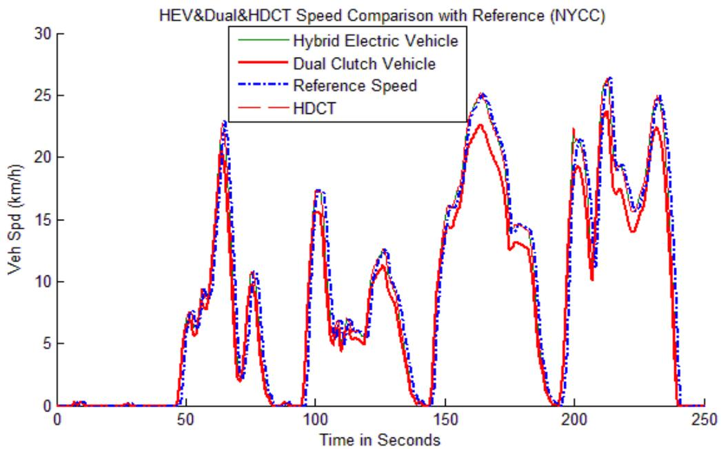
Figure 6.12. Comparison between the models and reference speed (NYCC)
