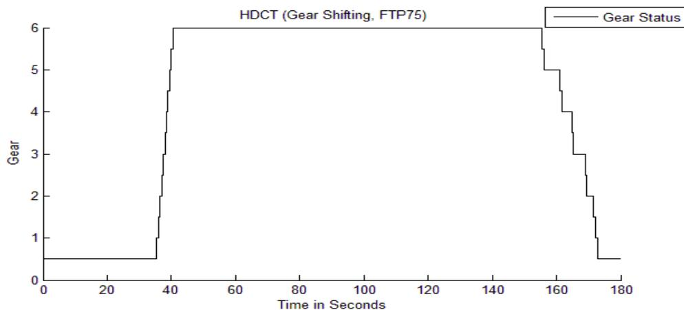
Figure 6.26. Gear-shifting for Dual Clutch Transmission Hybrid Vehicle (FTP75, Cold Start)
