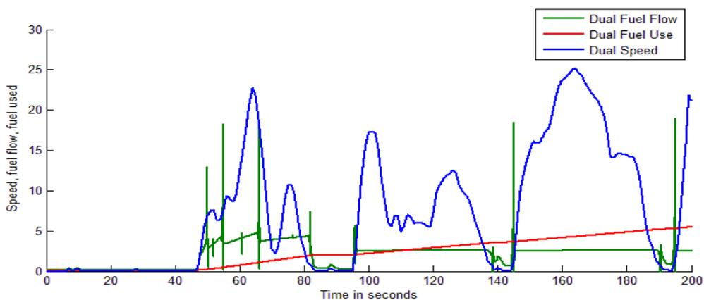
Figure 6.8. Dual Clutch Transmission Conventional Vehicle's (Performance – Fuel Flow – Fuel Use) (NYCC)
