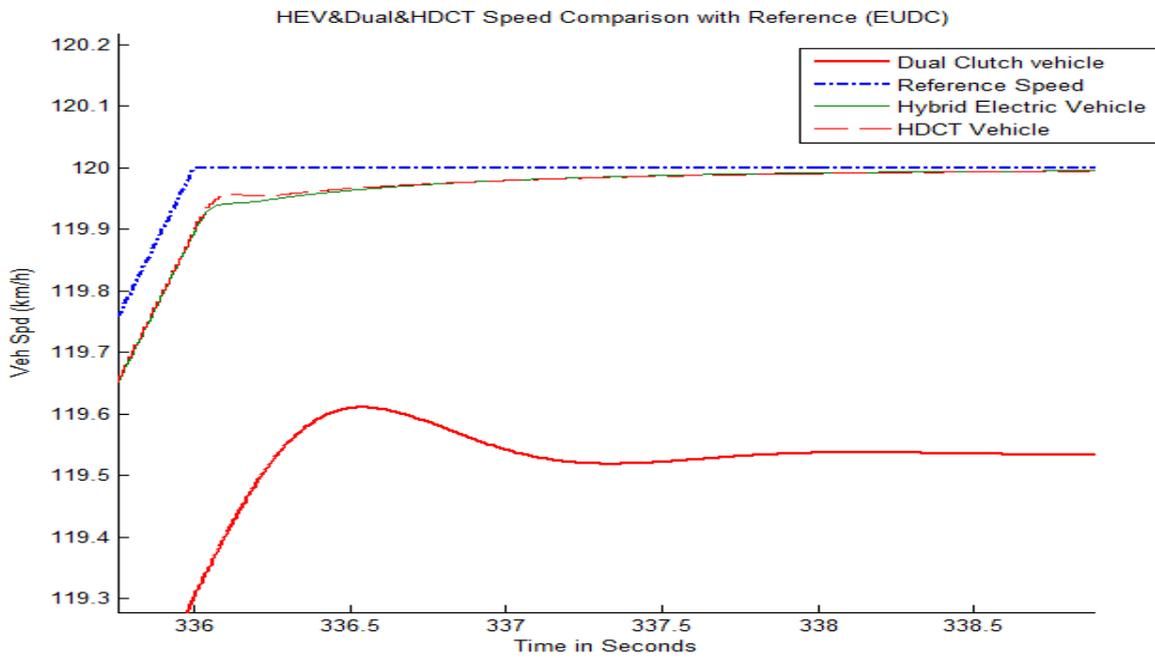
Figure 7.3. Chosen section of comparison between the three models, as (EUDC) is the reference drive cycle
