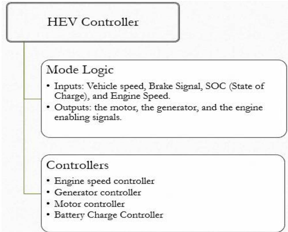
Figure 4.2. Hybrid Electric Vehicle Control Structure
