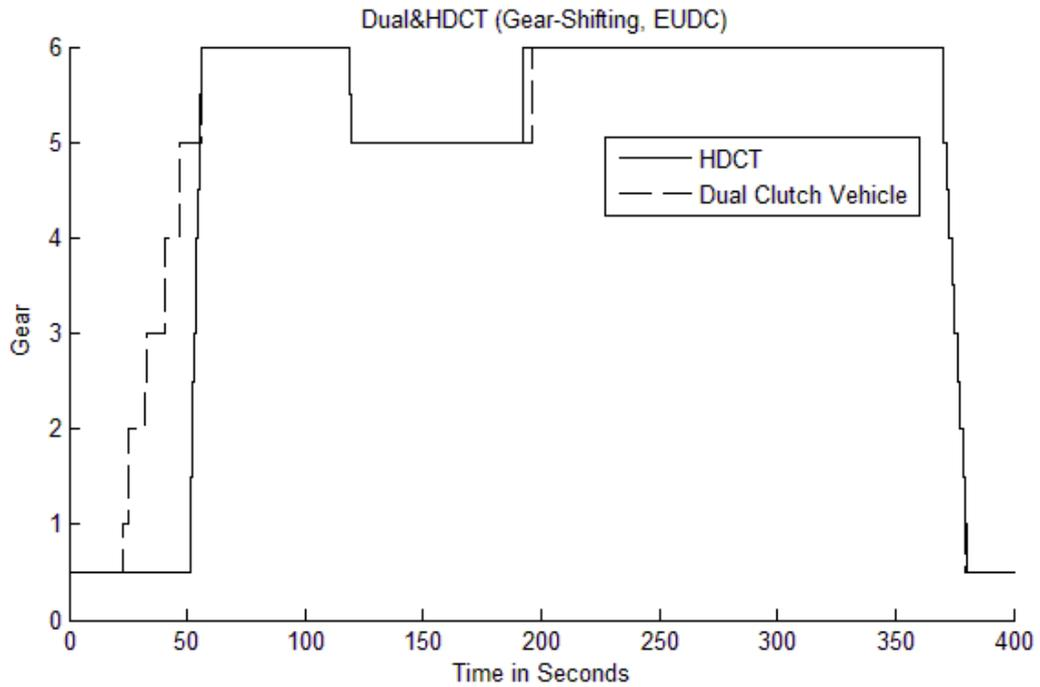
Figure 7.7. Gear Status comparison between HDCT&DCVT (EUDC)
