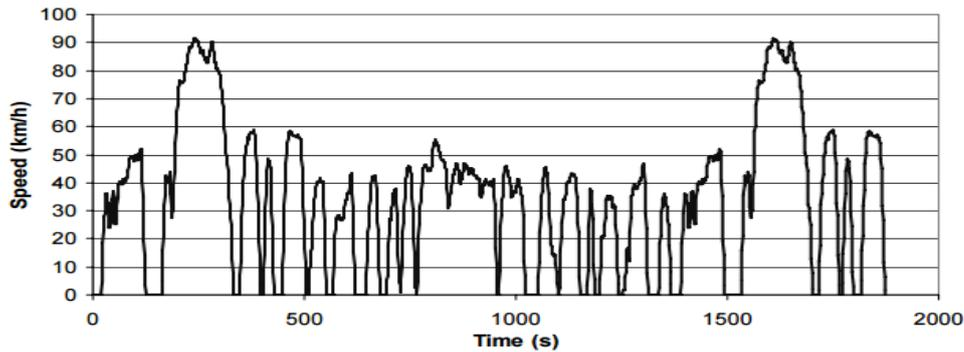
Figure 6.1. FTP75 Drive Cycle
