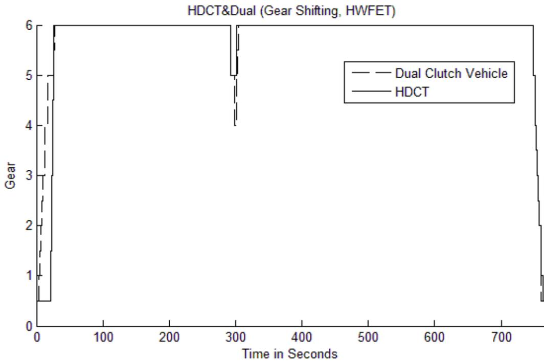
Figure 7.6. Gear Status comparison between HDCT&DCVT (HWFET)
