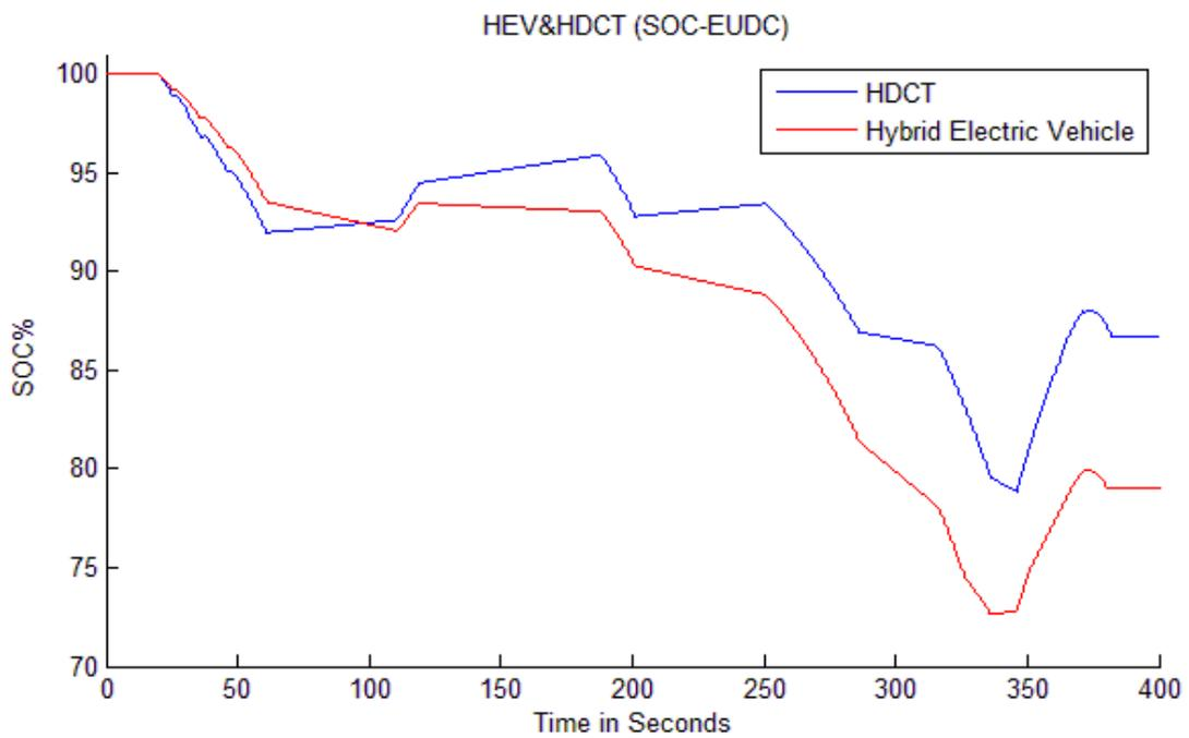
Figure 6.33. State of Charge comparison for HDCTV and HEV (EUDC)
