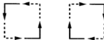
Fig. 1-3. XY routing with turn model representation © ACM 1992
