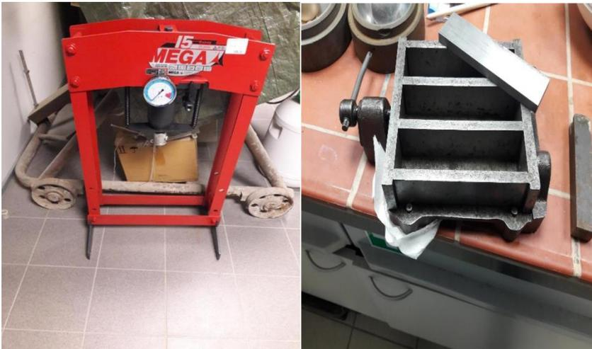
**Figure 4.** Pictures of hydraulic press and cuboid mold
