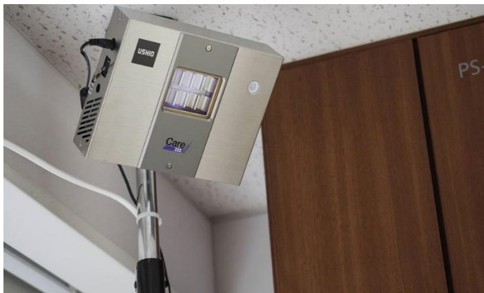
Joonis 6 Ushio inc. kaug-UV-lamp Care222 [36]
