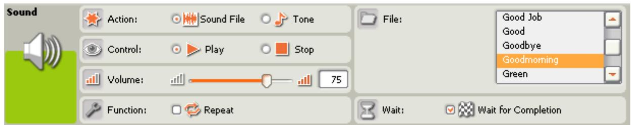
Figure 0.24 NXT-G Loop / sound block and settings
