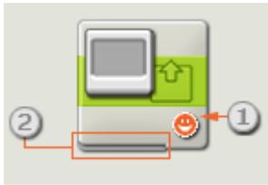
1. This icon shows whether the block is set to display an image, some text, or a drawing; or whether it will just reset the display to the default icon.
