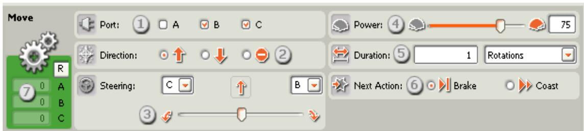
Figure 0.23 NXT-G motor block and settings
