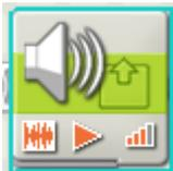
This block allows to program output sounds that will be played by the NXT controller. The volume level is controlled by this block.
