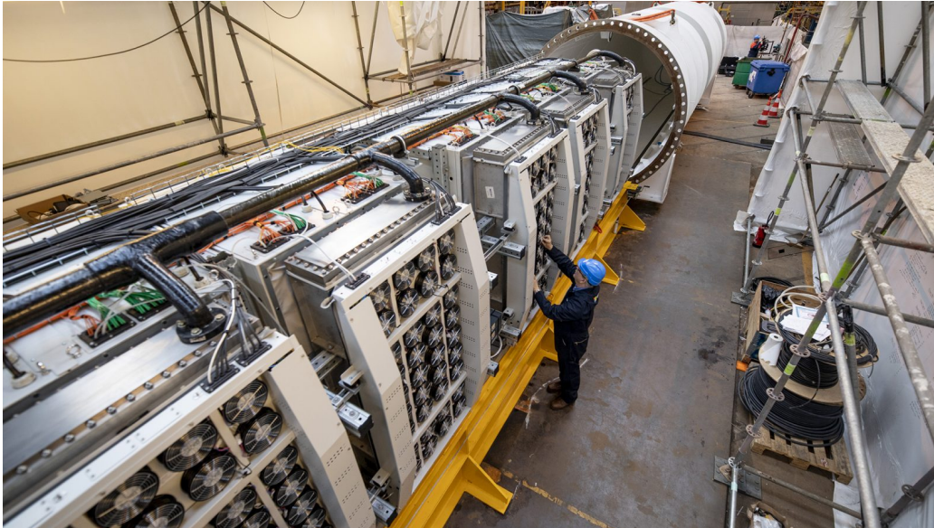
Joonis 4. Project Natick 2 sisemus (Microsoft Finds Underwater Datacenters Are Reliable, Practical and Use Energy Sustainably, 2020)
