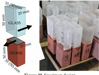
Figure 39. Specimen design
