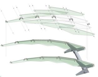
**Figure 4.** Detail drawing of Yurakucho load bearing structure by R. Hughes [17]
