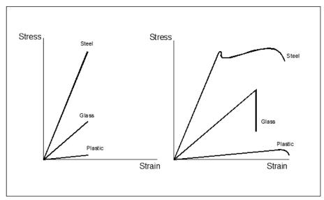
Figure 10. Stress-strain behavior of common materials
