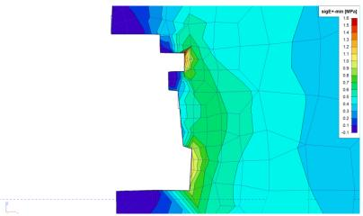
**Figure 73.** Close-up of the 2D model of the SW tower above axis C (screen proof from Scia Engineer 15). Inner stress magnitudes in the natural stone masonry by the load combination 1: Self-weight (Stone Masonry) + Point Loads from Glass
