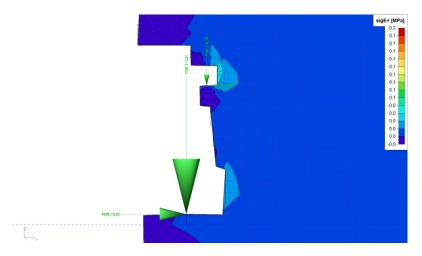
**Figure 75.** Close-up of the 2D model of the SW tower above axis C (screen proof from Scia Engineer 15). Inner stress magnitudes in the natural stone masonry from dead load of the connected glass structure inserted as point loads
