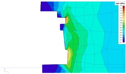
**Figure 74.** Close-up of the 2D model of the SW tower above axis C (screen proof from Scia Engineer 15). Inner stress magnitudes in the natural masonry from the self-weight of the structure
