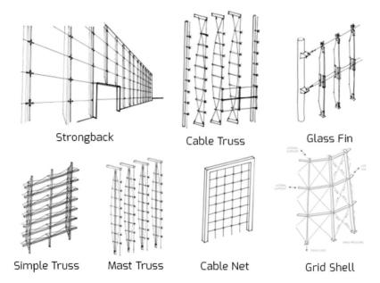
Figure 14. Common structural façade types according to M. Patterson [28]
