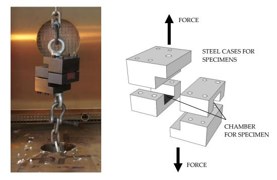
Figure 38. Design of the test set-up
