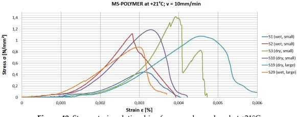
Figure 40. Stress-strain relationships for ms-polymer bond at +21°C
