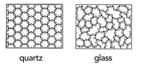
**Figure 8.** Molecular structure of SiO<sub>2</sub>, crystalline structure on the left (quartz) and amorphous on the right (glass)
