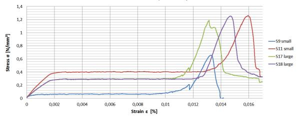
Figure 41. Stress-strain relationships for ms-polymer bond at +40°C
