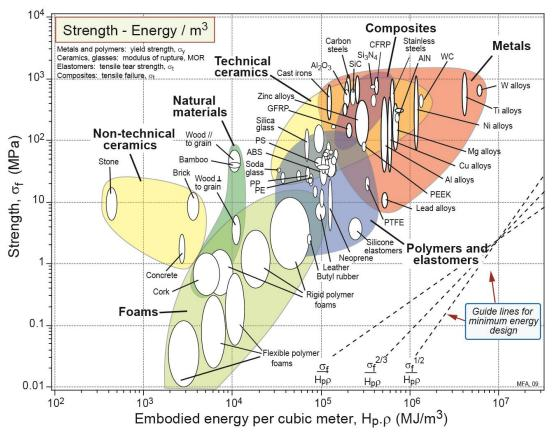
Figure 50. Embodied energy per unit cubic meter according to M. Ashby [31]
