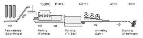
Figure 9. Float glass manufacturing process [25]
