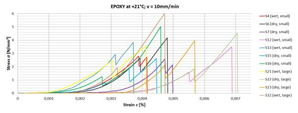
Figure 42. Stress-strain relationships for epoxy bond at +21°C
