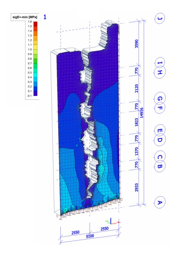
**Figure 72.** SW tower 2D model (screen proof from Scia Engineer 15). Informative graphical data of the equivalent (von Mises) stresses in the stone structure from the load combination 1: Self-weight (Stone Masonry) + Point Loads from Glass
