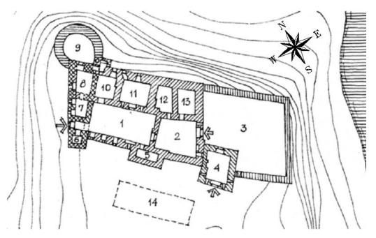
**Figure 29**. Ground plan of Toolse order castle by K. Aluve; 1 – courtyard from building stage II, 2 – stage II front yard, 3 – stage III forecourt, 4 – tower from stage III, 5 – tower from stage II, 6,7,8 – stage I residential quarters, 9 – bombard tower from stage V, 10,11,12,13 – stage II rooms, 14 – ruins of tavern, built later [60]
