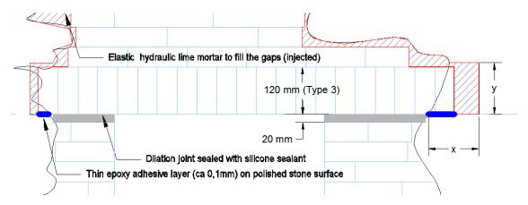
Figure 48. Dilation joints to allow vertical movement of the glass structure
