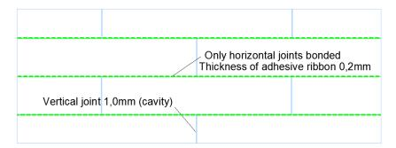
Figure 36. Structure of the glass block masonry system
