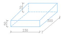
Figure 37. Special shaped glass blocks with inclined top surface for windows
