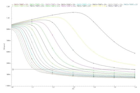
Fig. 4.6 Pass element sizes and input voltage sweep effect to dropout voltage
