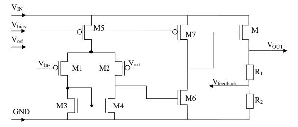
Fig. 3.2 LDO which amplifier have POMS input pair
