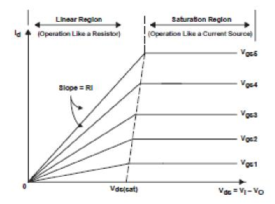
Fig. 2.6 Ideal characteristic of NMOS transistor
