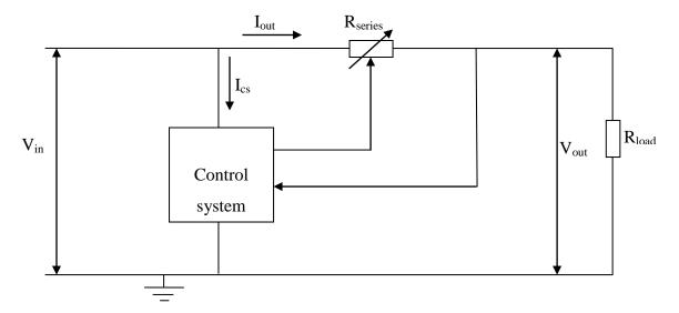
Fig. 1.1 The principle of a linear series voltage regulator
