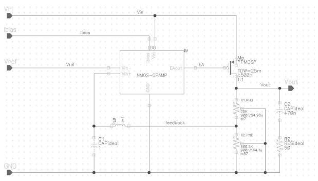
Fig 4.8 Modified schematic for AC sweep
