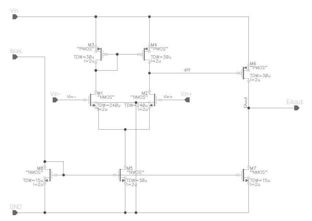
Fig 4.1 Operational amplifier with NMOS input pair design
