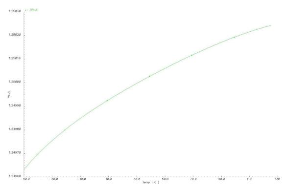
Fig 4.15 Temperature effect to output voltage
