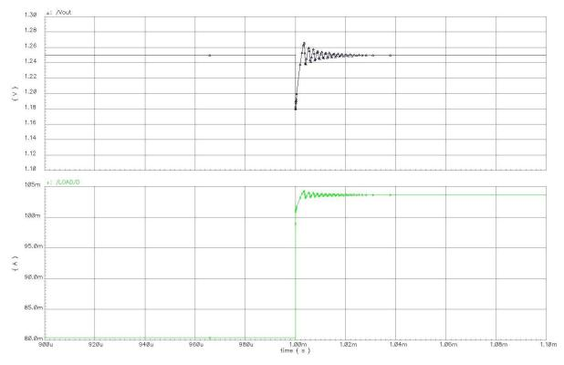
Fig 4.13 Load regulation when load change 20 mA
