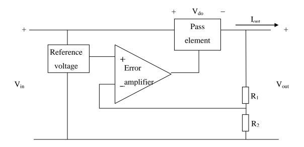
Fig. 2.3 Simple LDO block diagram
