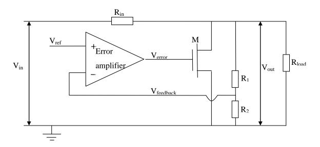
Fig. 1.5 A simple practical shunt regulator implementation
