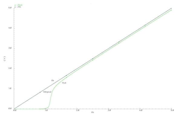
Fig 4.5 Pass element regulation
