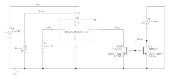
Fig. 4.4 Circuit design for simulating LDO
