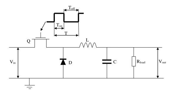
Fig. 1.8 Simple step-down switching converter
