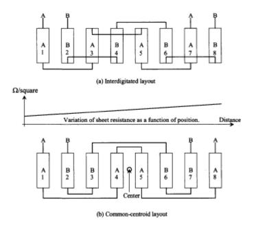
Fig. 5.1 Transistor matching methods
