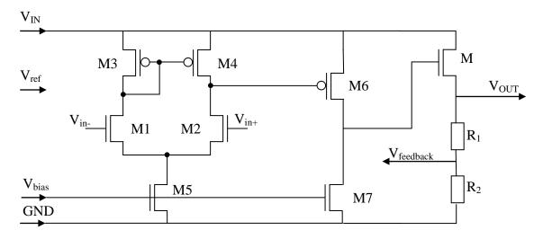
Fig. 3.1 LDO which amplifier have NOMS input pair
