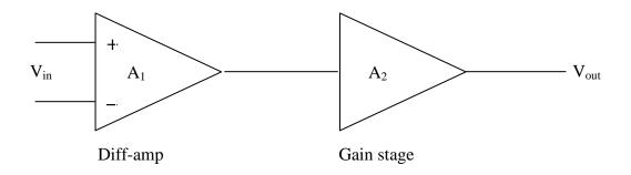
Fig. 2.7 Operational amplifier block diagram
