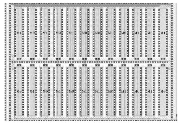
Fig 5.2 Matched differential input transistors
