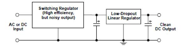
Fig. 2.1 Post regulation principle
