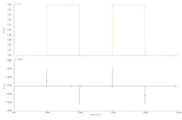
Fig 4.14 Line regulation when input voltage change 100 mV
