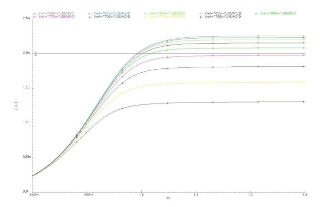
Fig. 4.2 Operational amplifier minimum supply voltage
