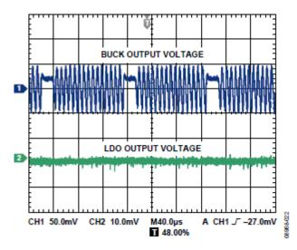
Fig. 2.2 LDO reduce buck regulator output noise
