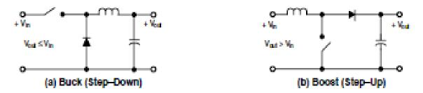
Fig 1.7 Two basic switching voltage regulators
