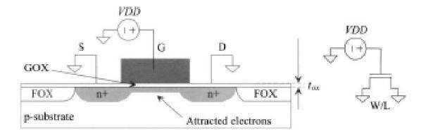
Fig. 2.5 NMOS device in strong inversion
