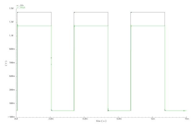
Fig 4.12 Transient response if input voltage appears with maximum load
