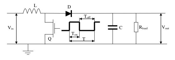
Fig. 1.9 Simple step-up switching converter
