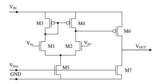
Fig 2.8 Simple operational amplifier schematic
