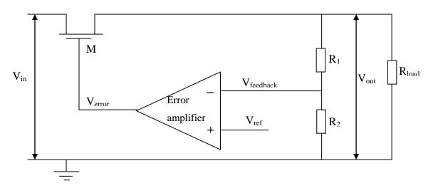
Fig. 1.2 A simple practical series pass regulator implementation
