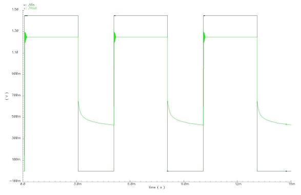
Fig 4.11 Transient response if input voltage appears with no load
