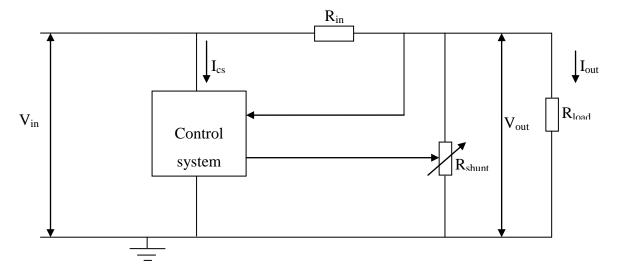
Fig. 1.4 The principle of a shunt voltage regulator
