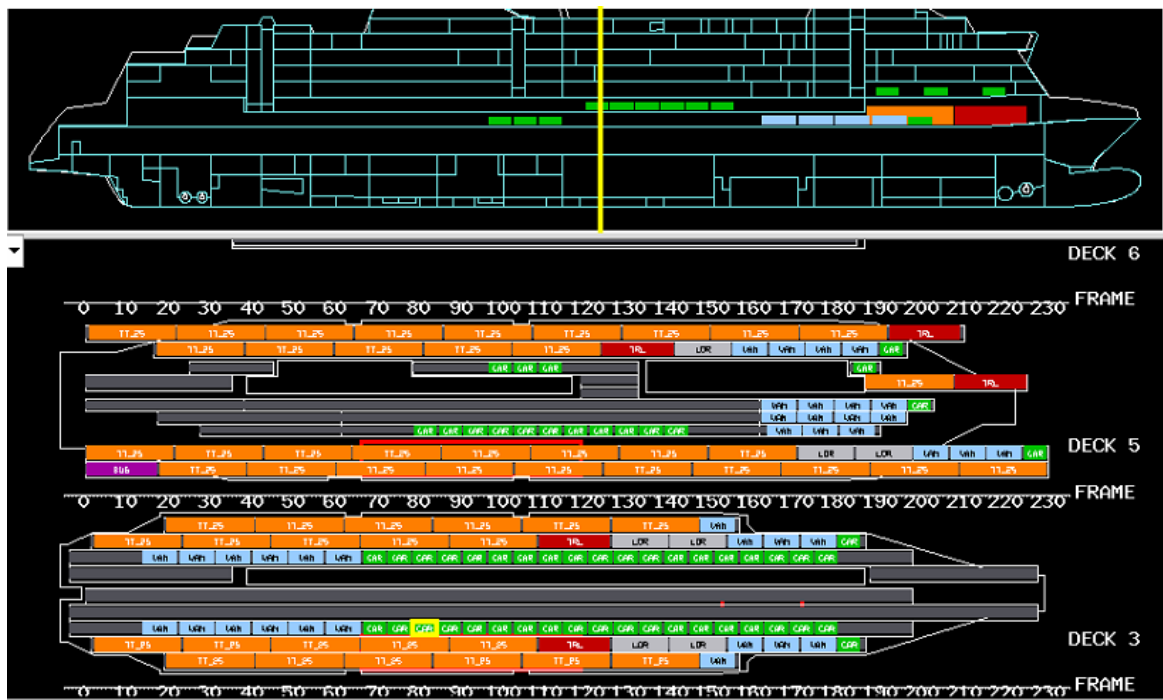
Figure 39. Visual representation of 3 and 5 deck vehicles placement
