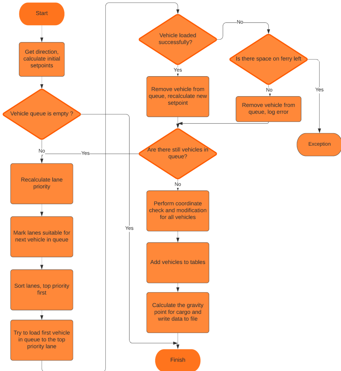
Figure 9. General loading algorithm
