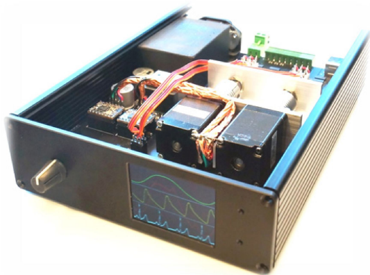
Fig. 3. Emulator of the cardio-respiratory dynamic impedance [13]
