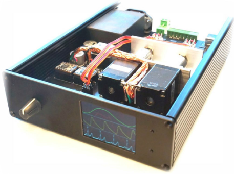
Fig. 11. Emulator of the cardio-respiratory dynamic impedance [22].
