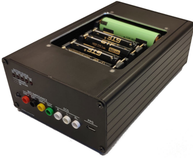
Fig. 6. Photograph of the developed device with batteries.
