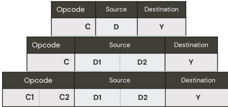
Figure 14: Mapping of miniMIPS instruction formats and the HLDD functional variable
