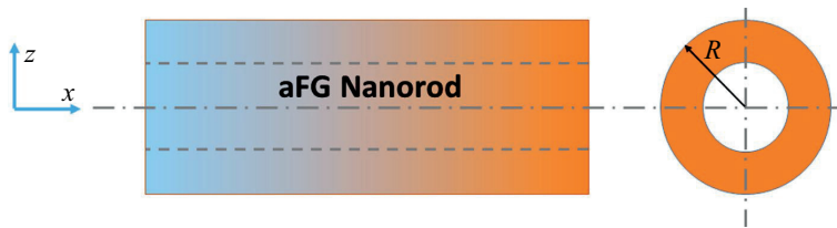
Fig 1. Axially graded nanorod continuum model.
