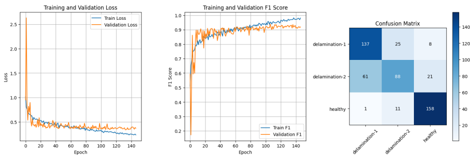
Figure 10. Training, validation loss, F_1 -score and confusion matrix for the Haar-CNN.
