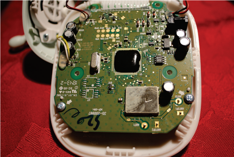
Figure 2. The inside of the baby monitor.
