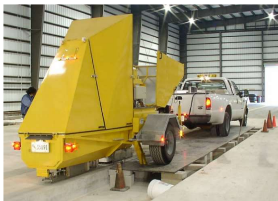
Foto 3.1. KUABi põhiseade ehk kahemassiline FWD. Foto allikast: U.S Department of Transportation. Federal Aviation Administration, [5]
