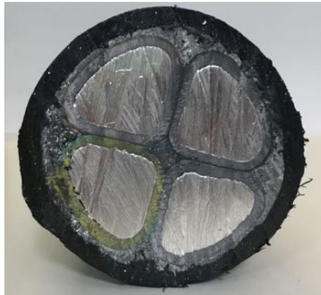
Figure 6 – Cross-section of a LV cable (type: NAY2Y 4x150mm<sup>2</sup>)
