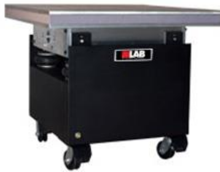
Figure 5. VibraTest™ Series Mechanical Shaker [22]
