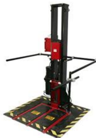
Figure 4. AccuDrop™ 500 Drop Tester [19]
