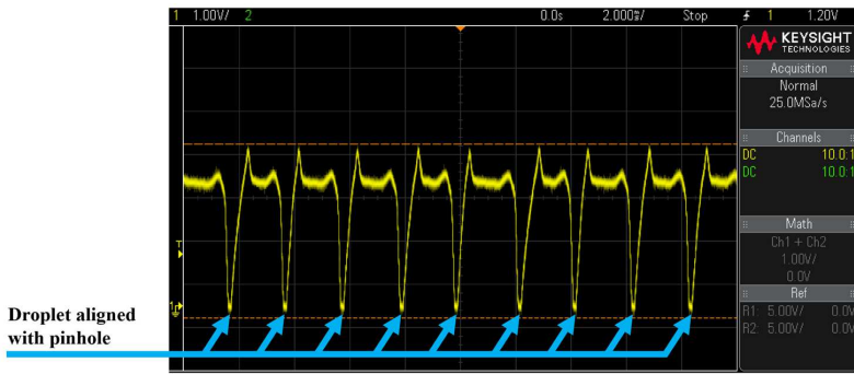
FIGURE 19. Oscilloscope screen capture of recorded amplified, inverted photodiode voltage during droplet generation with chip variant C, at a rate of ~500 Hz. Droplet alignment with the pinhole noted with blue arrows (at the “troughs”). Instability in the droplet production rate is recognizable by the varying time gaps between the „troughs“.
