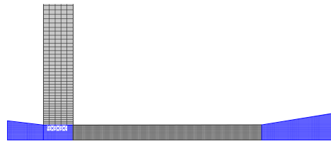
Figure 4: Tailored quadrilateral mesh with region-specific density. Avg. mesh quality: 97%. Total elements: 270,908. Mesh independence study confirms <1% droplet area variation with \geq 225,000 elements (Appendix section of Appendix 1)
