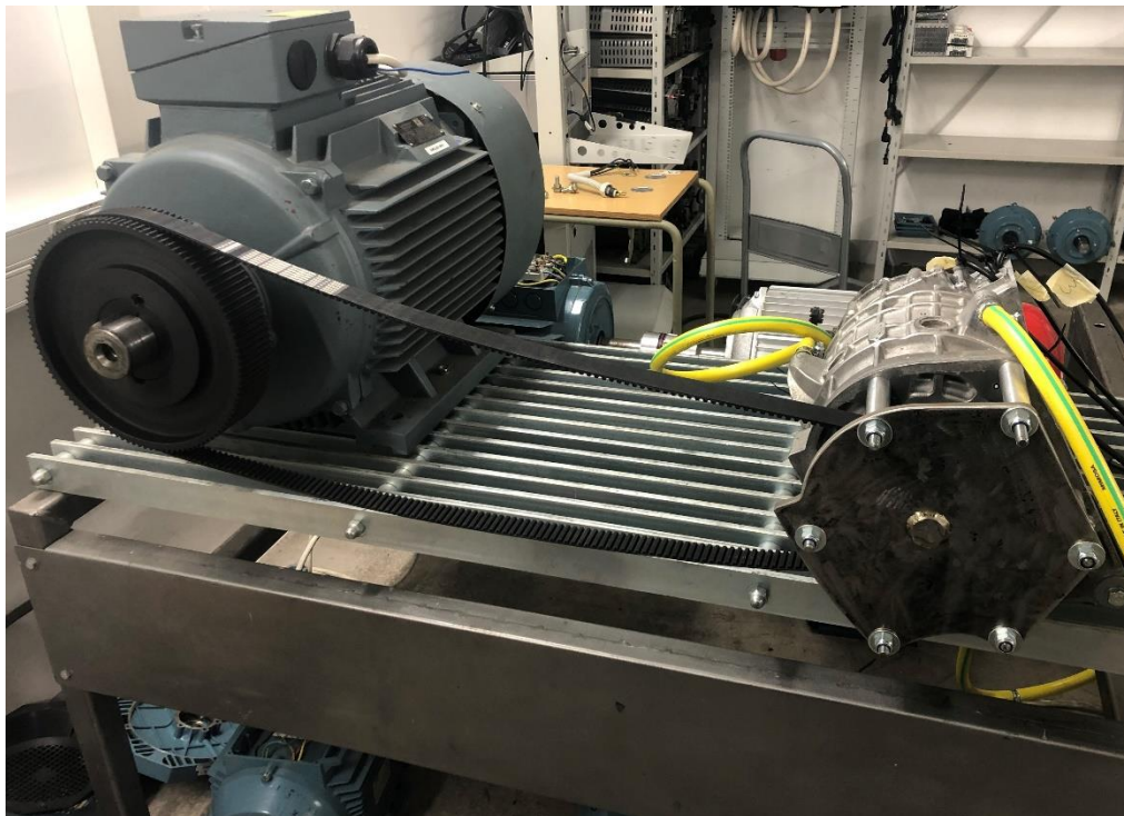
Fig.9: The clutch system (the load motor is on the left).
