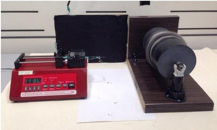
**Figure 3.** Electrospinning device which was used in our project.
