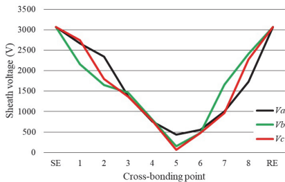
Fig. 10. Sheath voltages for three-phase cable line system with cross-bonded sheath installation at fault in RE bus.
