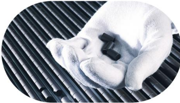
Figure 3: Pressed pellets of uranium dioxide [53]
