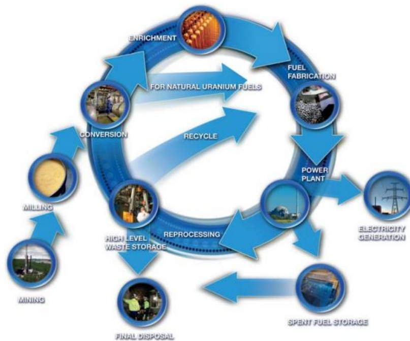
Figure 5: Nuclear fuel cycle, process starting from uranium mining and ending with nuclear waste disposal [15]
