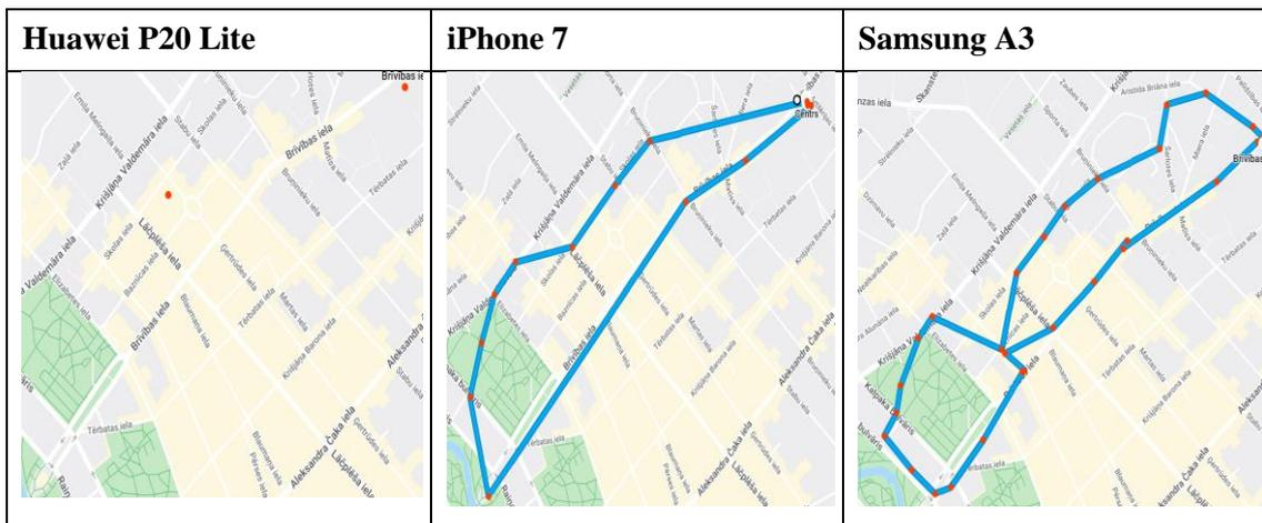
During the 53 minutes, only one location data point was collected on Huawei P20 Lite. We believe that this may be a one-time error. Therefore experiment 2 iteration two is performed to test this device configuration again. Device Huawei P20 Lite location accuracy was calibrated before the experiment.
