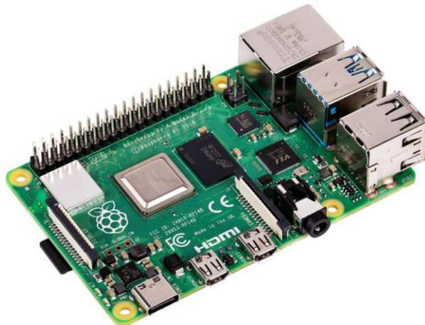
Figure 9. Raspberry Pi 4 model B [66] used for hardware deployment of the algorithm on the AP device.
