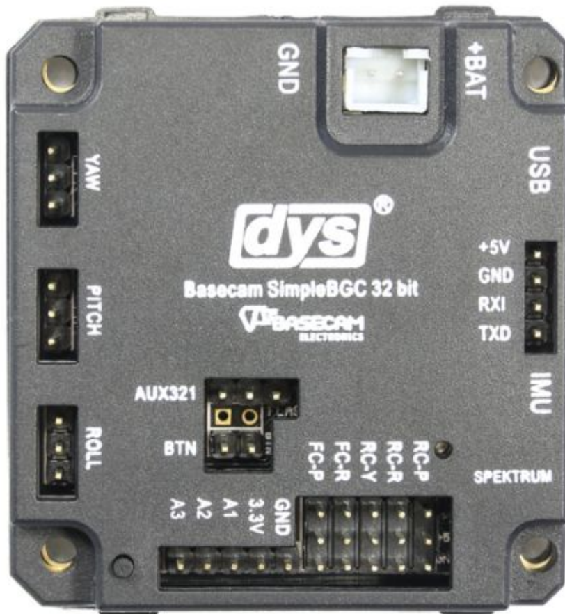
Joonis 2.4.1 Gimballi mootorite kontrolleri Basecam SimpleBGC 32 bit.[11]
