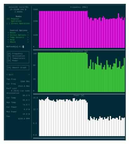
Figure 27. Screen capture of s-tui demonstrating the effect of Intel Powerclamp with 50% idle time.
