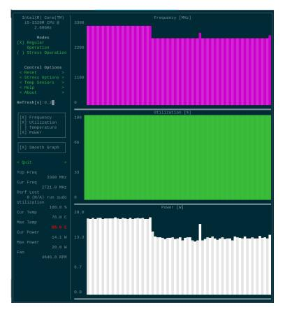
Figure 26. Screen capture of s-tui demonstrating the effect of disabling turbo mode using intel\_pstate driver.
