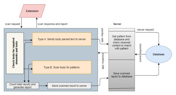
Figure 18. System architecture (extension)
