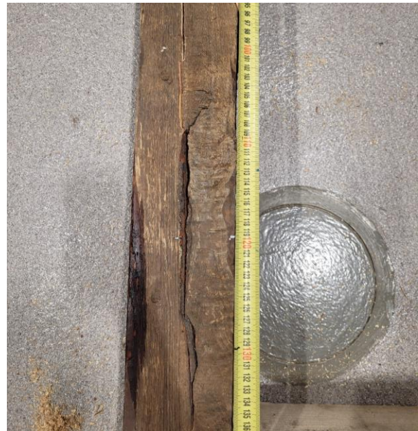
Photo 5.1.1-2 Specimen 21B with visible curly grain
