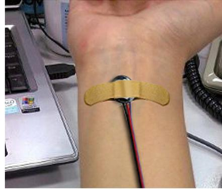
Figure 5.3 Wrist-attached Electrode
