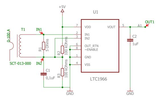
Figure 5.2. LTC1966 connection schematic
