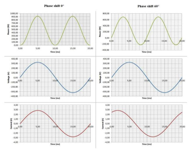
Figure 2.4. Sinusoidal waveforms of AC circuit
