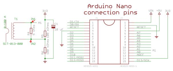
Figure 5.9. RMS measuring circuit based on Arduino Nano
