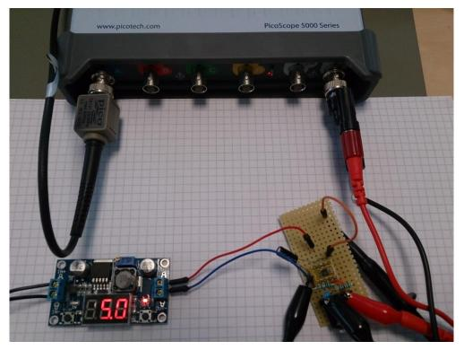
Measuring LTC1966 RMS to DC converter
