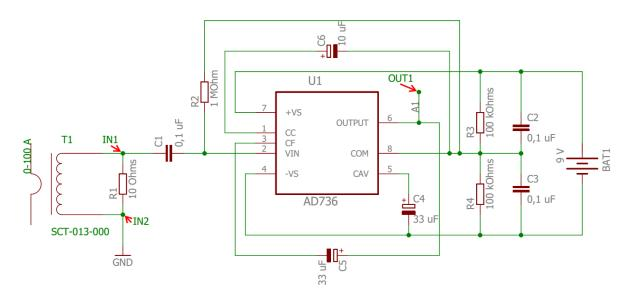
Figure 5.6. AD736J connection schematic
