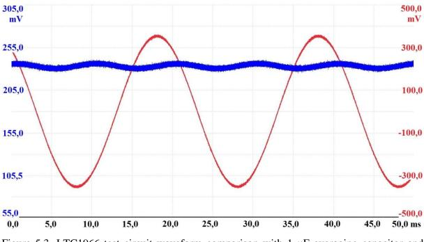
Figure 5.3. LTC1966 test circuit waveform comparison with 1  $\mu F$  averaging capacitor and 0,707 V peak to peak 50 Hz input
