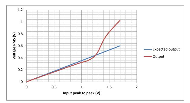
Figure 5.5. LTC1966 output comparison
