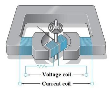
Figure 2.3. Simple wattmeter design [6]
