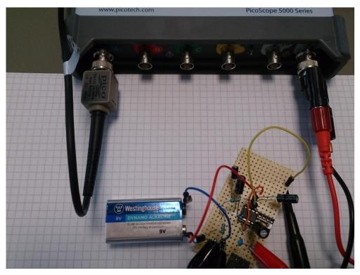
Measuring AD736J RMS to DC converter
