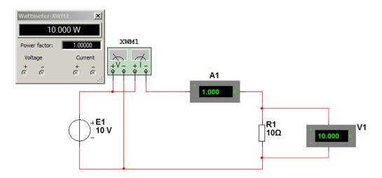
Figure 2.2. Power in simple series circuit
