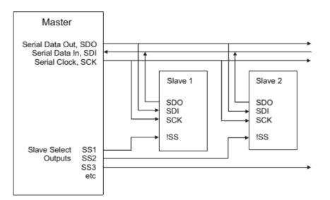
Figure 5.11. Serial peripheral interface (SPI) communication [29]
