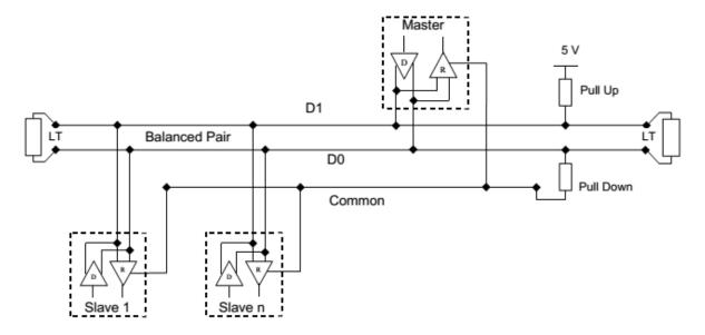
Figure 5.13. RS-485 two-wire (half-duplex) topology [32]
