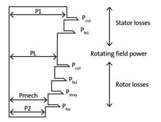
Figure 3.2. Losses in the induction motor [16]
