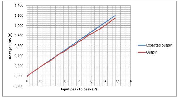
Figure 5.7. AD736J output comparison
