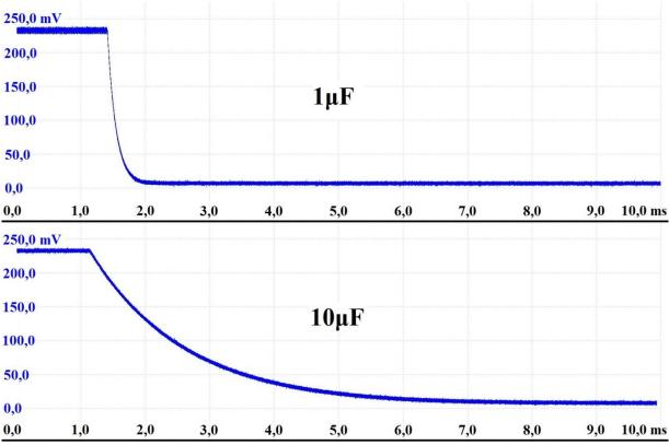
Figure 5.4. LTC1966 circuit output comparison with different capacitors
