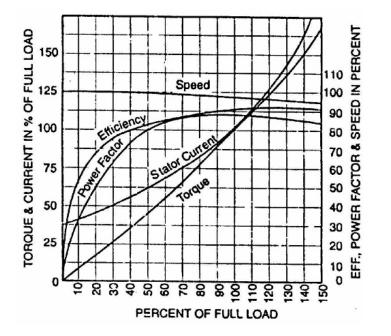
Figure 3.3. Performance curve of a three-phase squirrel cage motor [17]
