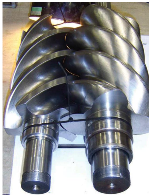
Figure 2.15 The screw expander rotors for wet steam expansion [65]
